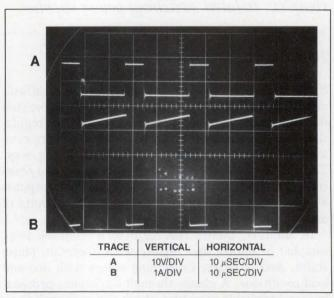
Fig 3—This photo is the result of the same setup as Fig 2, but shows what happens when the output demand doubles. In this case, the duty cycle doesn't change appreciably, but current doubles.
