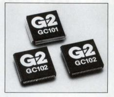
Chip sets such as the GC(PC/AT) from G2 can squeeze the functions of an IBM PC/AT-compatible mother board into as few as three ICs.
