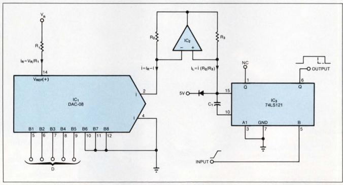
Fig 1—Op amp IC<sub>2</sub> mirrors the D/A converter's output current to the timing capacitor of one-shot IC<sub>3</sub>, providing digital control of the one-shot's output pulse width.
