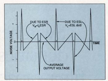
Fig 2—To establish practical limits for ESL, ESR, and  $C_{MIN}$ , derive each value by assuming that the other two make no contribution to output ripple and noise.
