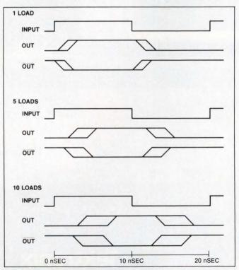
Fig 1—These waveforms show the effect of loading on the optimum clock driver circuit of Fig 2c.
