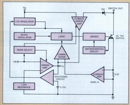
Fig A—The LT1070 is a current-mode, switching-regulator IC in which the switch current directly controls the switch's duty cycle.
