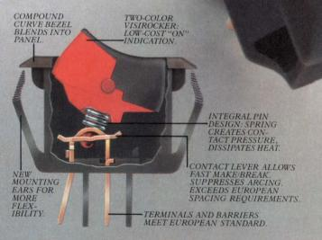
arc-suppressing fibre, in most applications. It will operate at maximum load in high ambient temperatures. Withstands 50,000 actuations, minimum, at full load. UL recognized, CSA certified for 16AMP 125VAC and 10AMP 250VAC. VDE certified for 10 (4)AMP 250V~µ.
