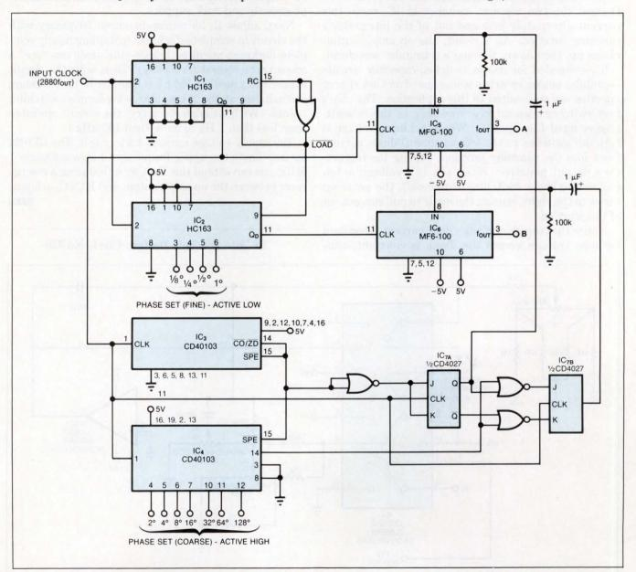
Fig 1—By extracting the fundamental components from two digitally synthesized square waves, this circuit produces two constant-amplitude sine waves with a programmable phase difference.
