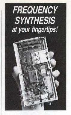
STEL-9272 Digital Direct Synthesizer provides a signal in the 2 KHz to 130 MHz band with a 1.1 Hz resolution. (Uses the STEL-2172 NCO.)
