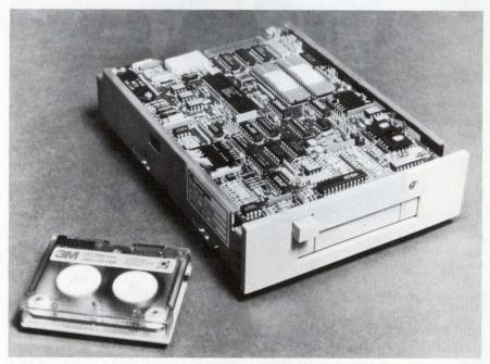
An error-corrected hard-error rate of 1 bit in 10<sup>11</sup> characterizes Wangtek's FAD-3500 tape drive. This error rate exceeds the hard-error rates of typical Winchester drives.
