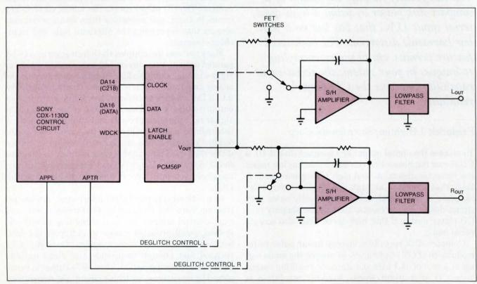
Fig 1—This CD-player design uses a single DAC for both channels. The control circuit operates at a clock frequency of 4.23 MHz and includes a  $2\times$  oversampling filter. The single serial output sends data that is decoded by the DAC and multiplexed to the appropriate channel by FET switches.
