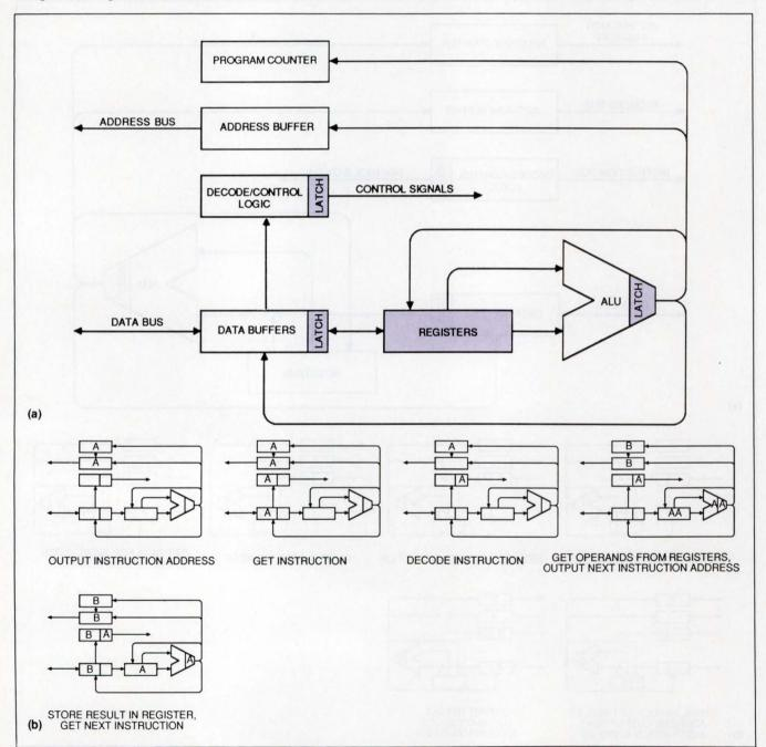
Fig 4—The RISC machine's divergence from the Von Neumann model is evident from the instruction sequence of b. Operands are generally available in on-chip registers (a) and results are stored there as well, resulting in better performance because of the faster accesses afforded by the on-chip registers.
