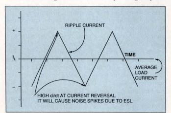
Fig 1—High ripple current is a fact of life in most switch-mode power supplies. The ripple shown is for a simple LC output filter typically found in forward or flyback converters; other designs, however, will have similar current waveforms.
