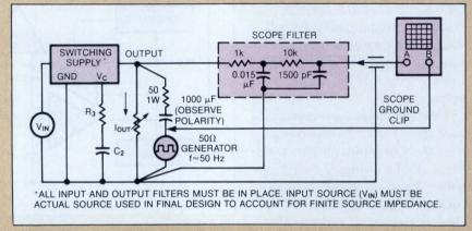
Fig A—You can use this setup to couple a load variation into the output of a switching supply and to observe the waveform of the supply's response to the load variation. Typically you set the amplitude of the generator's output to 5V p-p to generate a 100-mA p-p load variation.
