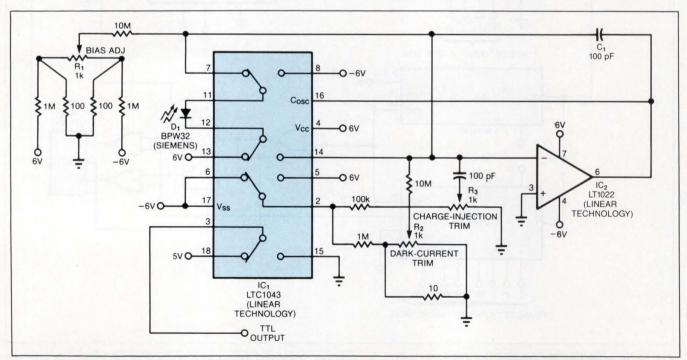
Fig 1—This wide-range (140-dB) I/F converter converts photodiode current to a frequency that ranges from 0.1 Hz to 1 MHz.
