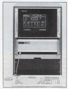
disk drive, a 20M-byte hard disk, serial and parallel I/O ports, six open expansion slots, and a video adapter that supports Hercules
