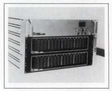
each accommodating from one to 16 plug-in cards; each card contains eight 2-pole crosspoints for a maximum of 4096 crosspoints. The crosspoints can be a mixture of coax, low-voltage and high-voltage types. The control options include an RS-232C, an IEEE-488, or a 16-bit-parallel bus. Configured with IEEE-488 and 128 double-pole low-level channels, \$3200.
