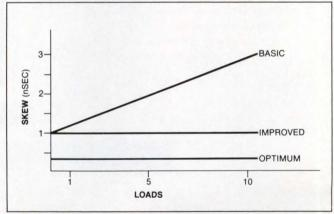
Fig 3—This graph of output load vs output time skew shows that Fig 2c's optimum circuit exhibits skew that is small and independent of load.
