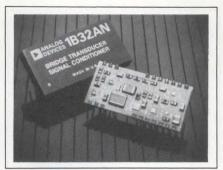
for 2 mV/V and 3 mV/V load cells. Additional features include a direct transducer interface with no external parts and a remote sensing interface with 6-wire load cells. To optimize performance, you can program the transducer's preset excitation from 4 to 15V at 100 mA. The integral 3-pole lowpass filter offers a 60-dB/decade roll-off from 4 Hz.
