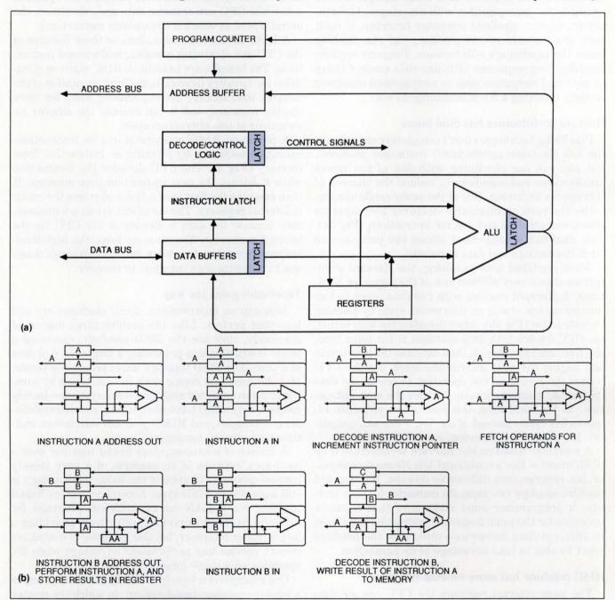
Fig 2—To increase the throughput of a Von Neumann machine, you can add latches to the control signals, data buffers, and ALU output (a). The latches allow the CPU to overlap the execution of an instruction with the fetch of the next instruction, which you can see in b's 3-instruction sequence.
