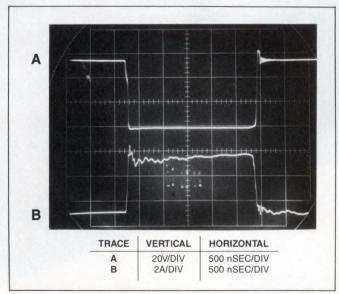
Fig 5—Trace A is the voltage, and trace B is the current at the V<sub>SW</sub> pin of the circuit in Fig 4. The ripples in the current trace are due to a nonoptimal breadboard layout. Inductor ringing during turn-off (trace A) is characteristic of flyback configurations.
