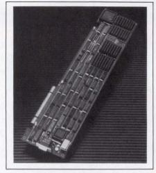
VDI standards. The board allows you to zoom to 30 levels and thus provides a virtual window of  $16000 \times 12000$  pixels. In an Auto-CAD environment, a bird's-eyeview feature gives you a close look at the portion of a drawing you're working on. Optionally, you can see four different views of an image simultaneously. A fast-erase feature lets you erase any portion of a draw-
