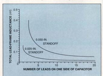
Fig 3—Adding lead frames has a small impact on component inductance, but that's the price you have to pay for reliable operation over temperature.
