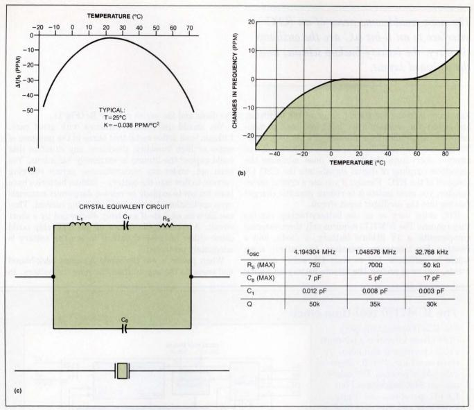
Fig 2—It's important to choose the right crystal for an RTC timebase. Wide variations of temperature cause the frequency of a tuning-fork-type crystal to drift (a). An SC-cut crystal is stable over a much wider temperature range (b). The characteristics of various crystal types are shown in (c).
