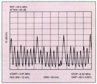
Fig 2—The spectrum-analyzer display of the pulse train shown in Fig 1 demonstrates that the spacing (62.5 kHz) of the noise spectral components is determined by the 16-usec period of the noise-waveform period.
