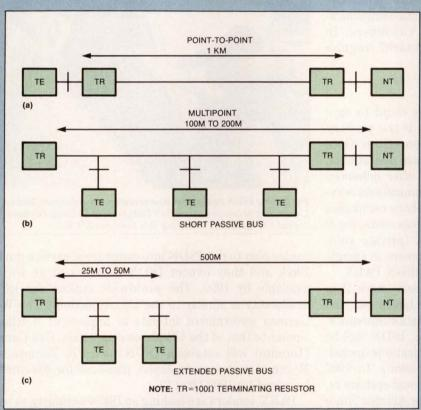
Fig B—Wiring for an ISDN S interface (S bus) can assume one of three topologies: a simple point-to-point configuration that's generally limited to 1 km (a), a short passive bus that allows terminal equipment to be distributed evenly along the bus (b), or an extended passive bus that clusters terminal equipment at one end and supports longer runs than the short-bus topology does (c).
