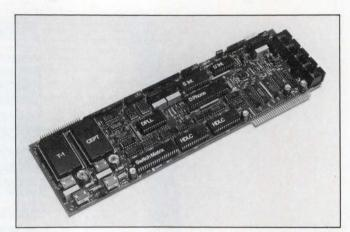
Combining ISDN basic-access and primary-rate chips, the MB89000 ISDN Express card from Mitel allows you to experiment with all of the ISDN interfaces.
