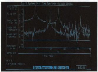
The R370 is a PC-based 10MHz Spectrum Analyzer. 2-channel, real-time, 10MHz FFT spectrum analyzer. Sample 2 channels simultaneously. 64K data buffers. Autosave in time or frequency displays to hard or floppy disk. Two modes of spectrum averaging: either blockmode (64-1K buffers) or individual sweeps. Linear or log amplitude scaling. Amplitude and frequency cursor. Display 1024 FFT spectrums 5 to 10 times a second (depending on PC configuration).
