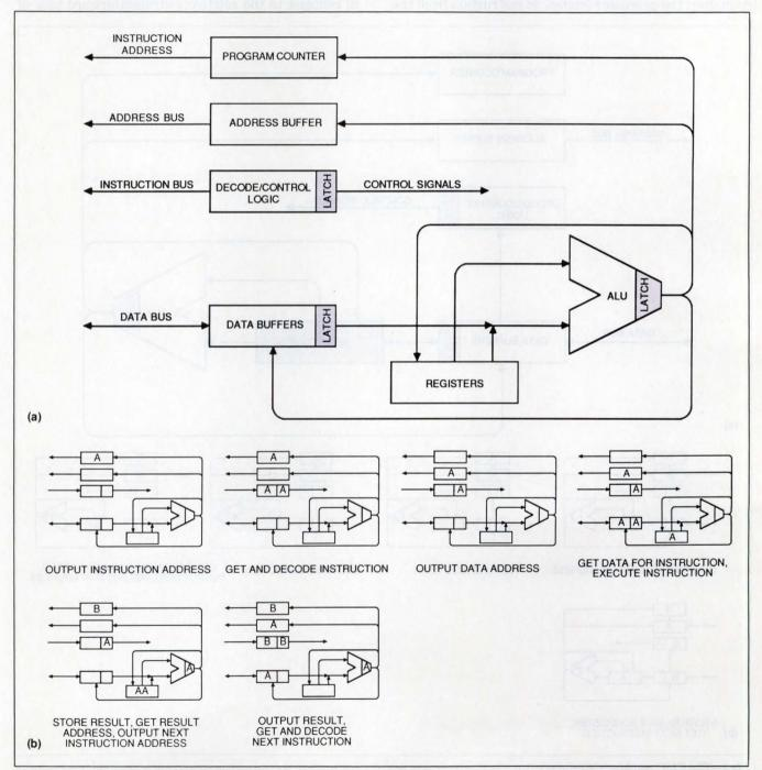
Fig 3—A pipelined Harvard processor, in addition to providing latches for pipelined operation, comes with both an instruction bus and a data bus, allowing some degree of parallel operation.
