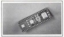
troller, an 8k×8-bit static RAM, an 8k×8-bit ultraviolet EPROM, and a proprietary logic-control unit. The epoxy-encapsulated, chip-on-board assembly yields a cost reduction of greater than 30% when compared to the price of the same device in a ceramic module. Device samples are available now; full production is scheduled for the first quarter of 1988. \$100 (100).
