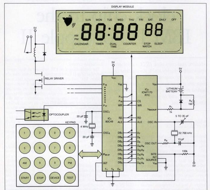
Fig 1—You can combine a modern real-time clock chip with an 8-bit  $\mu$ C to implement a universal timer/process controller. You can use ports  $P_{12-17}$  of the  $\mu$ C to drive a variety of alarms and peripheral devices.
