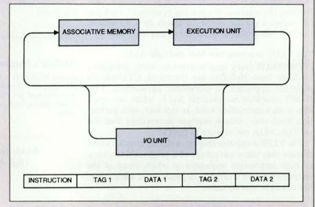
Fig A—Three basic units characterize a data-flow architecture: the execution unit, associative memory, and I/O unit (a). In the representation of the associative memory's internal organization (b), each instruction and each bit of data has a tag associated with it. After the comparator gathers all the data with the help of the tags, the instruction and data are all sent to the execution unit.
