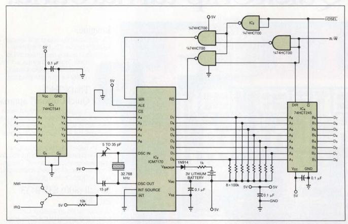
Fig 4—Interfacing an RTC to an Apple II is extremely simple because Apple expansion slots have unique base addresses; you don't need to perform any address decoding.
