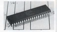
The ST-1172A generates digital sine and cosine functions of very precise frequency at clock speeds of up to 25 MHz. Features: 32-bit frequency resolution, 8 bits sine and cosine amplitude resolution, 12-bit phase outputs, 300mw power dissipation at 25 MHz.
