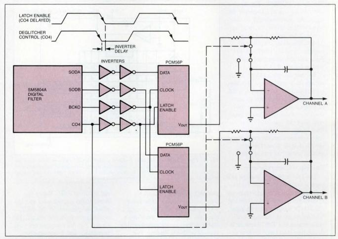
Fig 2—This high-end CD-player design provides separate DACs for each channel. The digital filter's left- and right-channel outputs operate at 4× oversampling frequencies. This scheme employs deglitching circuits, and the control signal is generated from the CO4 latch-enable output.
