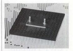
The STEL-2172 ECL Numerically Controlled Oscillator generates sine waves at very precise frequencies at clock speeds of up to 300 MHz.
