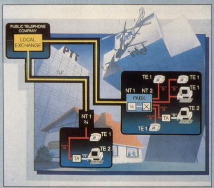
Fig A—CCITT's reference model for ISDN subscriber lines includes the undefined U interface (in yellow), which links the CO switch with the network terminator (NT) on the customer's premises, and the S interface (in red), which links an NT with the ISDN terminal equipment (TE). (Photo courtesy Intel Corp)
