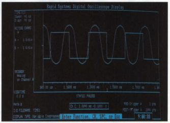
And the R370 is a PC-based 20MHz Digital Oscilloscope. Sample 2 channels simultaneously at 20MHz. 64K data buffers per channel. EMI protected metal case with power supply. Switchable 50 ohm or 1Meg input impedance. Software-selectable gain ranges allow resolution of 1mv to 250 volts. Full analog and 100% digital triggering. Trigger adjust potentiometer. Software drivers for "C", BASIC, and Turbo-Pascal.
