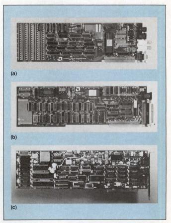
Semiconductor companies offer evaluation boards to help you determine the suitability of their ISDN chips. The boards from AMD (a and b) contain the company's Am79C30 and Am79C31, respectively. The board from Intel (c) mates the company's 29C53 and 29C48 with an onboard 80188  $\mu$ P. All three boards plug into an IBM PC or compatible computer.
