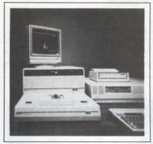
and operator interface, and report generation. You can program the test limits for many devices using menus; a Pascal-based language allows you to write programs for other parts. A 12-way multiplexer enables you to rapidly switch the 16-bit voltmeter from device pin to device pin; an S/H amplifier allows
