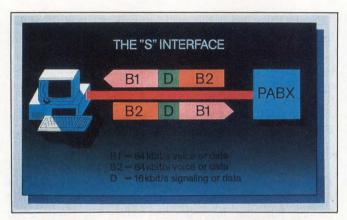
The ISDN S interface carries data at a 144k-bps rate in both directions simultaneously; the rate is allocated to two 64k-bps B channels (B1 and B2) and a 16k-bps D channel in each direction. (Photo courtesy Intel Corp)
