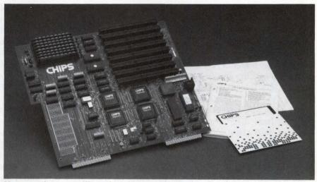
Most manufacturers will supply a chip-set evaluation board so that you can test a chip set before you buy. Chips and Technologies' CS8221 fits in the same form factor as the IBM mother board.
