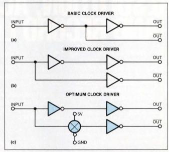
Fig 2—These are alternative circuit configurations for a biphase clock driver. Output skew for these digital CMOS circuits is illustrated in Fig 3.
