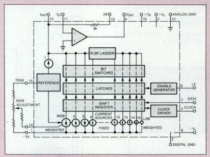
Fig A—The PCM56P 16-bit DAC includes a shift register followed by a latch for maximum loading flexibility. The ability to separate analog and digital supplies reduces the possibility of digital feedthrough, and its voltage reference and output amplifier minimize external component requirements.
