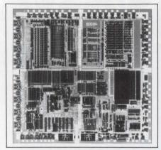
quarter of 1988. The device operates in several modes, including an HMOS-based 80186-compatible mode, a high-impedance test mode for in-circuit testing, and an enhanced mode with dynamic-RAM refresh and power-save logic. The dynamic-RAM-refresh controller is programmable to automatically
