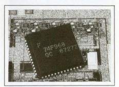
the four RAS (row address select) and CAS (column address select) outputs. The typical current drain is 265 mA. The unit eliminates the need for multiple controllers for the same function. It is functionally equivalent to the 2968 dynamic-RAM controller, but addresses four times the memory-array size and directly drives as many as 88 dynamic RAMs. In a plastic LCC, \$30 (100).
