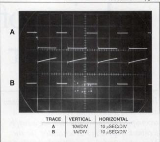
Fig 2—Trace A is the voltage, and trace B is the current waveform at the  $V_{SW}$  pin of the IC in Fig 1.
