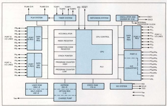
The MC68HC05B6 1-chip  $\mu$ C is an upgraded version of the MC68HC05C4; it includes an on-chip A/D converter, 256 bytes of EEPROM, and bidirectional I/O for synchronous and asynchronous communication.
