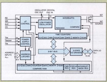
The ICM7170 RTC chip automatically switches to the backup battery when system power is turned off. The RTC can generate periodic interrupts as well as an alarm interrupt.
