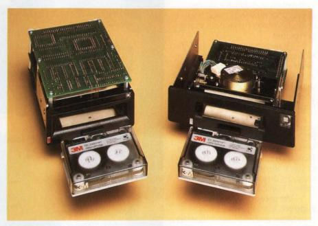
By offering both floppy-interface and QIC-100 models in 3½- and 5¼-in. form factors, 3M targets its MCD-40 tape-drive offerings at both low-end single-user systems and more-powerful systems that use the SCSI I/O bus.
