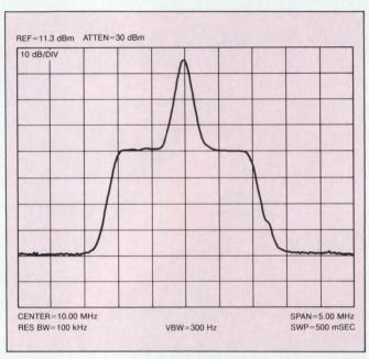
Fig 4—This spectrum-analyzer display shows a 10-MHz test signal contaminated with noise that is bandlimited to 2 MHz. The noise has a nearly Gaussian distribution with an SNR of 20 dB.
