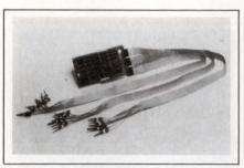
nel logic analyzer with 1k samples of memory for each channel. If you need only six channels, you can configure the analyzer to store 4k samples/channel. You can set the internal clock to any of eight frequencies from 25 kHz to 50 MHz, or you can supply an external clock at a frequency as high as 25 MHz and trigger on the rising or falling edge. You can begin the data display from 64 to 960 clock periods before or after the trigger point. \$749.
