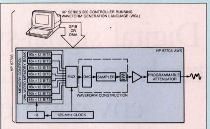
Fig A—In this arbitrary-waveform-synthesis system, the AWS is interfaced to an HP Series 200 controller running WGL.
