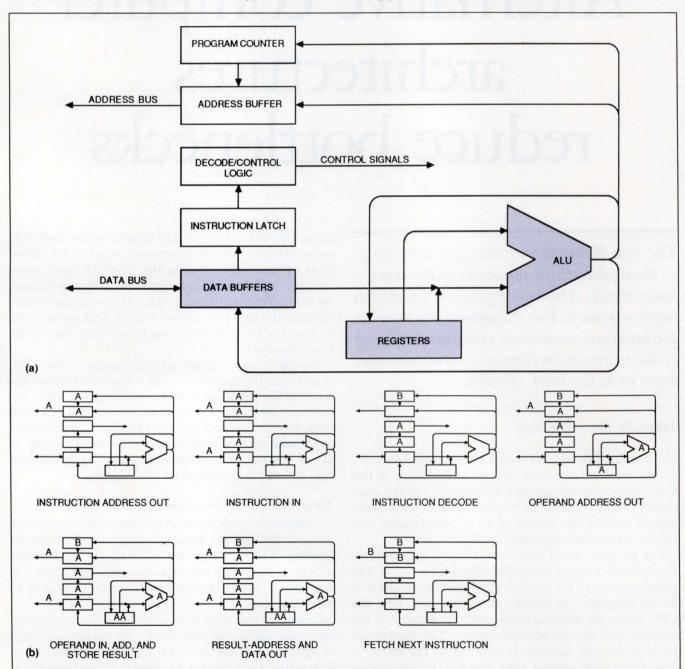
Fig 1—In a typical Von Neumann configuration (a), the ALU has input paths from the registers and data buffers and feedback from the ALU output. In b—an illustration of the flow of instruction and data information for two instructions, A and B,—note that instruction A has to be complete before the next instruction, B, is even fetched.
