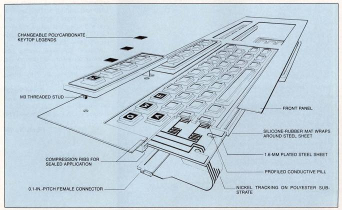
While retaining tactile feedback and positive key travel, the self-supporting keys of the SF62000-Input conductive-rubber keyboards eliminate the need for rigid switch housings. As a result, the keyboards have no cracks or crevices to harbor dust and dirt, and you can scrub them down.
