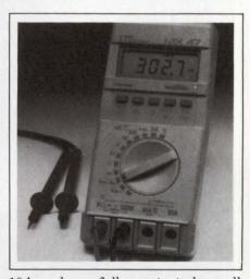
10A and are fully protected on all ranges. Typical voltage drop in the meter for current measurement is 500 mV. Basic dc accuracy ranges from 0.7 to 0.1% depending on the model. The top-of-the-line modelthe MX47-includes rms measurement on ac voltage and current, and ac or ac and dc coupling. You can also use the MX47 with K-type thermocouples to provide a direct read-
