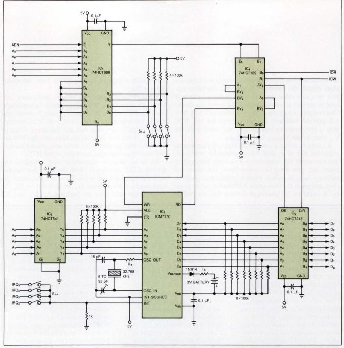
Fig 3—You need only four 74HCT support chips and a few discrete parts to construct an interface between the ICM7170 RTC chip and an IBM PC. Buffers isolate the RTC from the PC bus except during I/O operations specifically addressed to the RTC.
