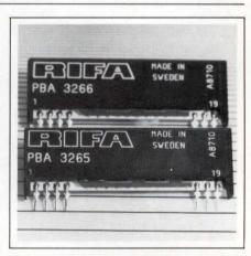
The resulting group-delay variation is constant within  $\pm 30 \ \mu$ sec for frequencies to 19 kHz. You can employ its built-in sin x/x compensation network to facilitate the use of the filter/equalizer combination as a reconstruction filter following a D/A converter. The sin x/x section is designed for a system that provides a 48-kHz sampling rate. Each circuit comes in a single-in-line package. PBA-3265, \$24.50; PBA-3266, \$29.50 (100).
