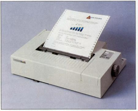
An extended version of the manufacturer's PCL (printer control language) includes color commands to control the Paintjet printer from Hewlett-Packard.
