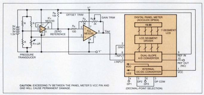
Fig 9—This bridge-transducer interface circuit conditions the bridge's output signal for ratiometric operation and eliminates the need for a reference voltage and an instrumentation amplifier.
