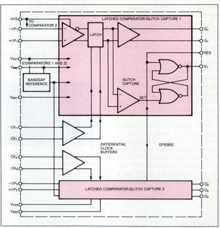
Fig 3—Each channel in the Plessey SP9380X dual, quad, and octal comparators includes a comparator, an output latch, and glitch-capture circuitry.
