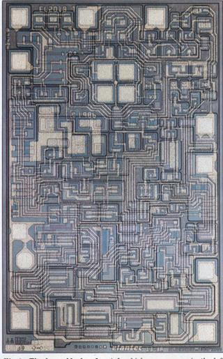
Fig 1—The large blocks of metal, which you can see in the left center of this die photo of Elantec's EL2018, are replaced by a second latch in the otherwise-identical EL2019. The second latch implements the EL2019's flip-flop.
