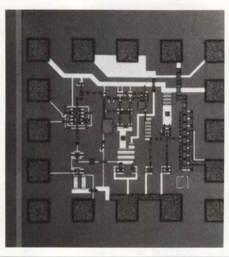
A 100-mV overdrive enables the ACP10010 from Anadigics to achieve a propagation delay of 500 psec. This GaAs comparator can maintain a gain of 100. er-supply requirements might drastically increase the complexity of the external circuitry.
