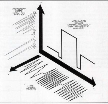
Fig 1—The "modulation domain" is the term Hewlett-Packard coined to describe the measurement area where its 5371A excels, and to contrast the types of measurements it makes to those made by scopes and spectrum analyzers.
