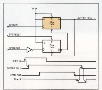
**Fig 1—In this configuration**, flip-flop  $IC_{1A}$  exhibits edge-sensitive set and clear controls: A low-to-high transition of XFER IN sets the device, and a high-to-low transition of XFER OUT clears it.
