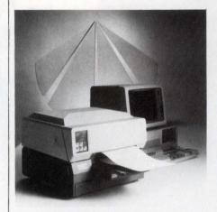
Liquid-Crystal-Shutter (LCS) technology charges the photosensitive drum in Data Technology's Crystalprint VIII page printer.
