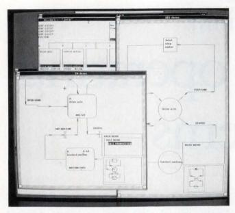
This display of a task map, data-flow diagram, and control map from Ready Systems' Cardtools CASE package documents a realtime software system.
