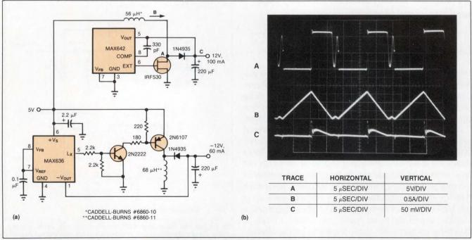
Fig 2—With the addition of a few external components (a), the circuit of Fig 1 can supply currents of 100 mA at 12V and 60 mA at -12V. Traces A, B, and C (b) represent the switch voltage, inductor current, and output ripple for the 12V supply.
