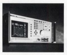
Besides having a set of keys adjacent to firmware-generated legends on the screen, the 5371A's front panel also provides cursor arrows and both keypad and rotary controls for data entry.
