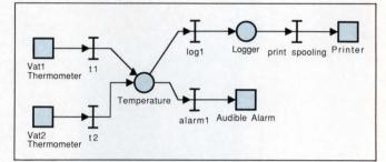
In this data-flow diagram of a real-time system, squares are external devices, I-beams are communications interfaces, and circles are tasks. The diagram was produced with a graphics editor, from Andyne Computing, that allows you to document the structure of a real-time system.
