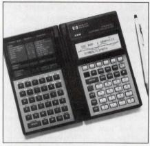
With increased memory and an augmented user interface, the HP-28S scientific calculator supercedes the HP-28C.
