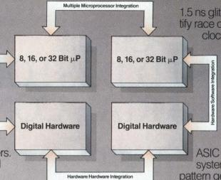
**3** Simultaneous integration of up to six microprocessors. Use the dual timebases and real-time handshaking between system modules to set up split-screens displays that scroll in precise time alignment.
