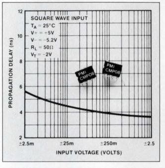
A comparator's propagation delay isn't constant. For example, Precision Monolithics' CMP08 exhibits a variation in propagation delay with a varying input signal level.
