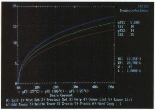
Characterizing a power MOSFET using Parts
