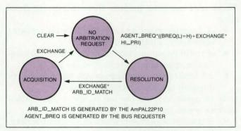
Fig 3—The arbitration-control state machine controls an agent's bus requests. An agent acquires ownership of the bus when the EXCHANGE condition is met and when the agent's ID matches the ID on the bus-arbitration lines.
