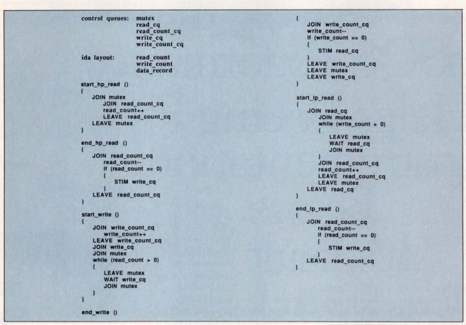
Fig 4—Using all the techniques developed in Figs 1, 2, and 3, these routines allow for two classes of readers: a high-priority class that takes precedence over readers and a low-priority class that doesn't.
