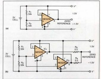
Fig 8—The circuit in a converts a 3V cell into a  $\pm 1.5V$  dual tracking supply. By connecting two amplifiers in parallel (b), you can nearly double the circuit's load-current capability.
