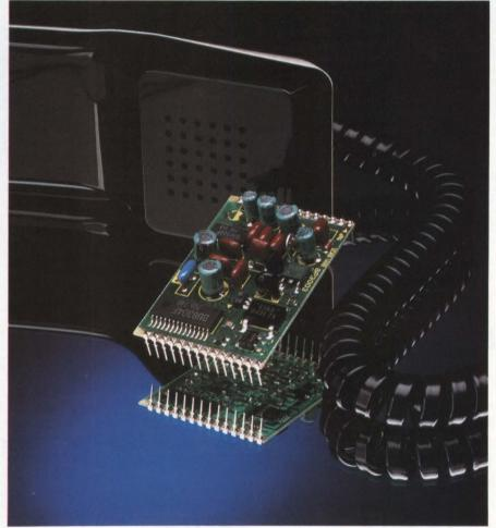
Forming the basis for a complete telephone, this module from Rohm includes a DTMF dialer, a speech network, and a tone ringer.
