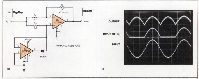
Fig 3—This absolute-value circuit (a) achieves full-wave rectification by clamping  $IC_2$ 's noninverting input to 0V when  $V_{IN}$  is negative, and removing the clamp when  $V_{IN}$  is positive. Thus,  $IC_2$  alternates between an inverter and a follower every half cycle. The photo (b) shows circuit performance at 400 Hz for a 5.7V p-p input signal. The vertical scale is 2V/div, and the horizontal scale is 0.5 msec/div.
