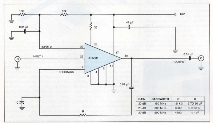
When you use the LH4200 as a feedback amplifier, you can control its gain with a single resistor in a series-feedback configuration. The accompanying table shows various gain/bandwidth options for the part. The only external decoupling required for this amplifier is the  $47-\mu F$  electrolytic capacitor.
