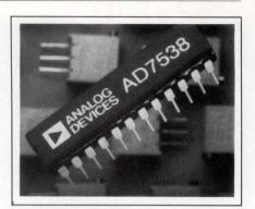
simultaneous updating in systems that use multiple DACs. Using standard chip-select and memorywrite commands, the current-output DAC is parallel-loaded by a single 14-bit word. Applications include microprocessor-based control systems, digital audio, and precision servo control. You can obtain the device in a 24-pin plastic or ceramic DIP. \$10.50 to \$51.90 (100).
