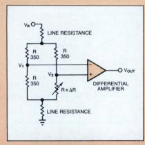
Fig A—In a conventional transducer bridge, the parameter of interest causes a variation ( $\Delta V$ ) in the bridge's output. The amplifier senses the resulting small differential signal and also rejects the bridge's relatively large common-mode voltage.
