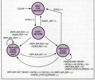
Fig 6—The replier-transfer state machine manages the handshake logic in the replying agent to transfer data.
