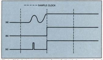
Fig 3—If the logic state at normal sample time is the same as that of a preceding glitch (a), the latch-mode display (b) completely fails to show the glitch. The second-order glitch display (c) does indicate the transient.
