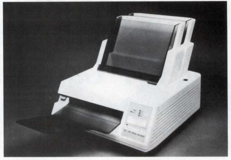
The LED engine that Fujitsu uses in its 5-page/minute RX7100 proves to be a low-cost alternative to a laser-based engine.
