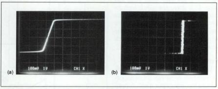
Fig 2—The transfer function of Elantec's EL2018 (a), operating in a transparent mode, shows the limitation of its gain as the input moves through the active region. In the latched mode, the EL2019 (b) has a gain limited only by the noise of the input. For both photos, the vertical scale is 1V/div, and the horizontal scale is  $100 \ \mu V/div$ .
