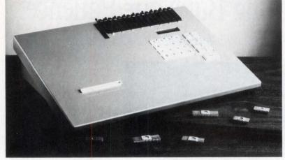
THREE PROGRAMMERS IN ONE. With the addition of the 135 MultiProgrammer<sup>™</sup> BYTEK has provided a true Universal Programming Site. The 135 is a SET EPROM Programmer, a GANG EPROM Duplicator, and a UNIVERSAL DEVICE Programmer, designed for Engineering Development, Production and Field Service Environments.
