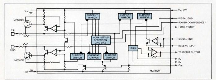
Fig 5—Because it provides all the basic functions for a subscriber-line interface, the MC34120, along with a codec, can replace the transformer in PABX systems and other applications.
