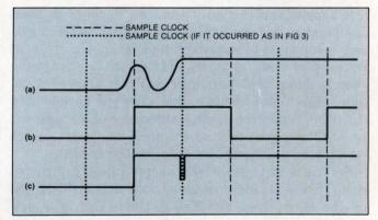
Fig 4—When normal sampling and a positive-polarity glitch occur simultaneously (a), the latch-mode glitch detector can be fooled into detecting a negative-going glitch (b) after the real glitch. The secondorder glitch detector (c) provides a fairly accurate representation.
