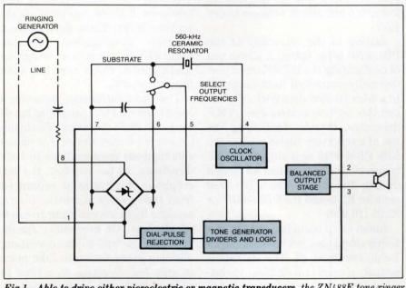
Fig 1—Able to drive either piezoelectric or magnetic transducers, the ZN488E tone ringer from Ferranti includes an on-chip bridge rectifier for direct-line operation.
