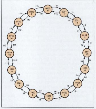
Fig 1—This diagram describes a state machine based on four T flip-flops. The state machine has 16 states; none are unused.
