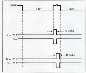
Fig 2—These timing waveforms for the circuit in Fig 1 show the relationship between the  $\overline{MUTE}$  signal and the reset and latch-enable pulses.
