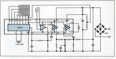
Fig 3—Essentially a 1-chip telephone, the PBL-3780 from Rifa includes a DTMF generator for tone dialing, a speech network for 2- to 4-wire conversion and signal amplification, and a simplified tone ringer.
