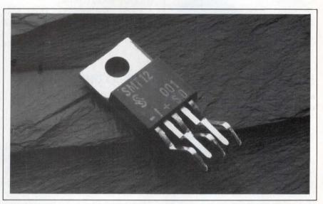
state, the device will block 45V at very low standby current consumption. \$6.25 (1000).
