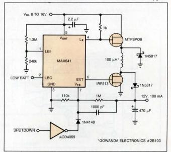
Fig 4—A buck/boost converter can accommodate wide input-voltage swings, such as the 8 to 15V swing typical of a 12V sealed lead-acid battery. The LOW <u>BATT</u> output indicates when input voltage drops below 8V. Pulling SHUTDOWN low turns off the circuit.
