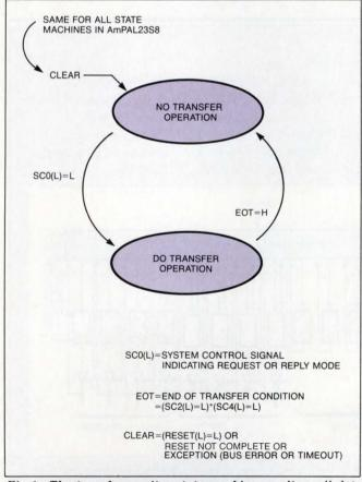
Fig 1—The transfer-monitor state machine monitors all data transfers taking place on the system bus. A transfer operation begins when SCO(L) goes low.
