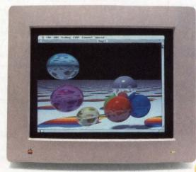
Macintosh II. 640x 480 resolution, displays 256 colors simultaneously from a 16.8 million color palette. Bt453. Triple 8-bit 40 MHz RAMDAC with 256 color lookup table. Monolithic CMOS.
