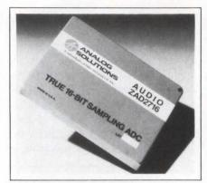
over the audio band of 20 Hz to 20 kHz. Its frequency response is stable to within 0.1 dB from dc to 50 kHz, and its rms noise is 30  $\mu$ V typ. The shielded, integrated module includes a precision A/D converter, a separate sample-and-hold circuit, clock circuitry, a precision reference, and a digital interface. \$235 (100).
