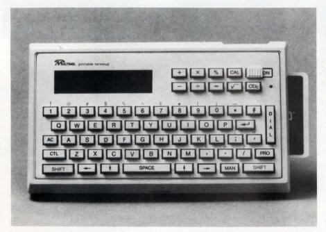
Weighing 12 oz and measuring  $6\frac{1}{3}\times3\frac{3}{4}\times1\frac{1}{4}$  in., the Multiportable terminal lets you read, write, and program a Memocard smart card that contains an 8-bit  $\mu$ P and 2k or 8k bytes of EEPROM. An optional modem adds voice- and data-communication capabilities to the terminal's standard word-processing and calculating functions.
