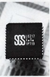
Incorporating two H-bridge drivers, outputcurrent regulators, and D/A converters, SGS-Thomson Microelectronics' L6217 and L6217A stepper-motor controllers allow you to microstep a 2-phase bipolar stepper motor. The plastic leaded chip carrier's special leadframe allows the devices to dissipate 2W.
