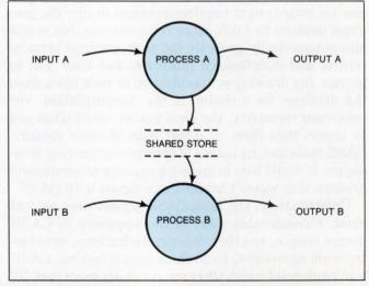
Fig 1—This simple data-flow diagram shows the symbology of the Yourdon-DeMarco structured-analysis methodology.
