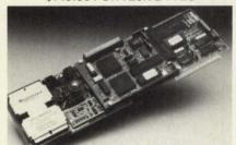
Rugged and reliable bubble memory systems for IBM PC/XT/AT. Master full length PC card includes SCSI host adapter and 720K Bytes of user available, non-volatile storage. Expandable to over 5M Bytes with additional slave cards. Acts like a hard disk under MS-DOS. 30ms access time. Comes complete with manual, drive and 2-year warranty.
