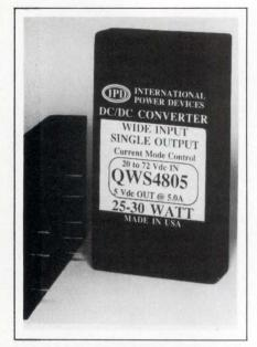
All modules operate at 100 kHz. Models are available that operate on nominal input levels of 24 and 48V dc, having 9 to 36V and 20 to 72V limits, respectively. All units output either 5, 12, or 15V. The full-load efficiency specs at 82 to 86% and is virtually unaffected by line and load changes. The output accuracy specs at  $\pm 1\%$ .
