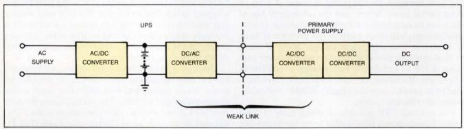
Fig 2—The weak link in a conventional UPS system is the dual power-conversion circuitry. The electrolytic filter capacitors used to reduce line-frequency ripple and to provide long hold-up times are the main contributors to reliability compromises in these systems.
