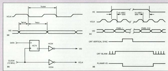
Timing for flat-panel displays differs from that for CRTs. A Planar display, for example, requires that data satisfy setup and hold times (a), which can be ensured by device propagation delays in a synchronizing circuit (b). The HS signal also must meet stringent timing requirements (c). VS can be derived from CRT-controller signals (d) and must meet HS/VS edge-timing requirements (e); a simple circuit suffices for VS generation (f). For an NEC display, timing requirements differ somewhat (g).
