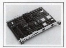
with 4-level arbitration. Its options include a VSB memory expansion interface, a 68851 paged-memory-management unit, and a 68881 or 68882 floating-point coprocessor. Software support for the board includes VRTX/32 Real-Time Executive from Ready Systems, OS-9 from Microware Systems, and PDOS from Eyring Research. \$2695.
