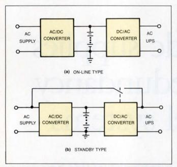
Fig 1—A conventional UPS comes in two configurations. An on-line type (a) operates continuously, and provides line filtering and battery back-up. A standby type (b) has a bypass switch that switches in the UPS only in the event of a line failure.
