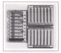
specifications, jumper positions for daisy-chaining Bus Grant and IJack signals, 20A power terminals, and 32-bit expansion and user I/O. The backplane design also lets you use a plug-in VMX board that connects to I/O-bus rows A and C on the connector. A 5-slot VMEJ1 backplane, \$195.
