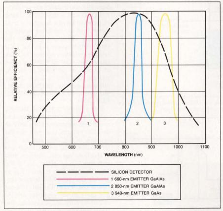
• Fig 2—Optocoupler emitters are usually made from materials such as GaAs, GaAsP, and GaAlAs. Application-dependent factors such as efficiency and the wavelength of the emitter's spectral emission determine which type a manufacturer selects. Fortunately, a silicon detector can accept a wide range of emitted wavelengths.
