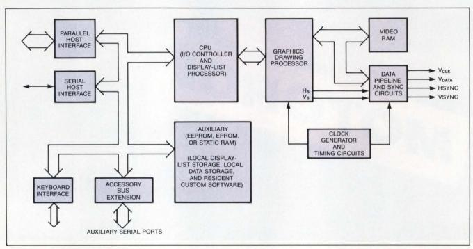
Fig 4—High-end smart controllers typically employ a dual-processor design. One processor controls all I/O tasks while the second provides parallel display processing and control functions.
