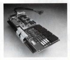
Plug-in boards for PC-based image processing such as Data Translation's DT2871 color frame-grabber board) let you perform gray-scale processing, hue and saturation processing, and frequency-domain analysis at capture and display rates reaching 30 frames/sec. The DT2871 plugs into the DT7020 floating-point array processor to boost system performance during computation-intensive operations such as color edge detection, compression, and FFT analysis.
