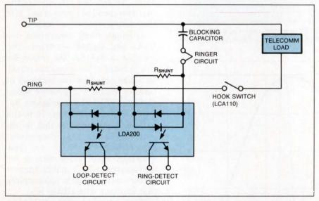
Fig 3—In this telecommunications application, the LDA200 optocoupler from Theta-J monitors the line to detect the presence of loop current and a ring signal.
