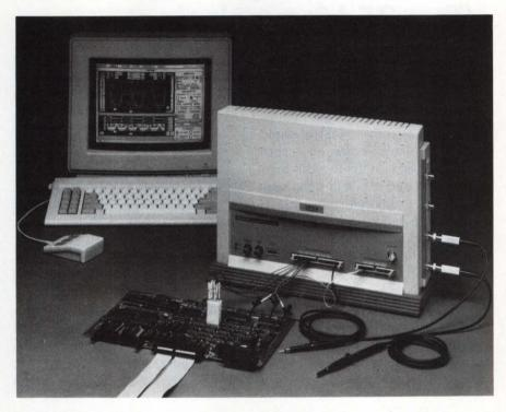
tion with flexible triggering permits the unit to capture and display every occurrence of infrequent events such as missing pulses, metastable states, noise glitches, and bus contentions. From \$8900. Orion Instruments, 702 Marshall St, Redwood City, CA 94063. Phone (800) 245-8500; in CA, (415) 361-8883. TLX 530942. Booth Nos 2741, 2743, and 2745.
