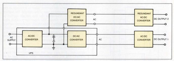
Fig 3—Building redundancy into a conventional UPS system can be bulky and expensive. In this configuration, both the dc/ac inverters and the ac/dc output rectifier supplies have redundancy.
