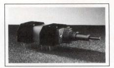
ing in of the lifetime lubricant and allows a mechanical life of 25,000 operations. Detent angles of 30, 60, and 90° are available, as are a variety of shaft and bushing sizes. Special options include molded Delrin spacers between decks and shaft extensions. The switch can carry 6A and has a make/break rating of 0.1A at 125V ac and 0.25A at 28V dc. \$8 (OEM qtv).
