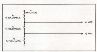
Fig 1—This circuit illustrates the general problem that Listing 1 solves. You provide the  $V_1$  minimum and maximum inputs, plus a value and tolerance for each of the resistors.
