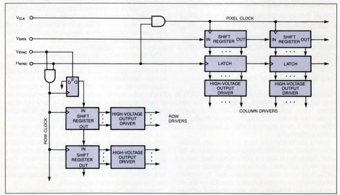
Fig 1—A flat-panel display's drive electronics typically includes three elements: row drivers, column drivers, and timing and control circuits.
