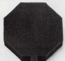
The secret of Soundcoat's exclusive SOUNDMAT LF is an inner limp mass flexible septum between one layer of isolation foam and an outer layer of embossed foam.
