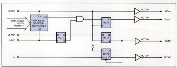
Fig 2—Flexibility is a key feature of today's flat-panel controllers. This output stage, for example, can drive all popular sizes of EL displays as well as many plasma-type devices.
