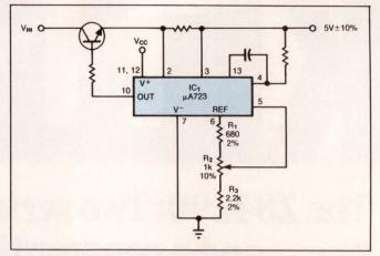
Fig 2—Using the Listing 1 program, you can choose a combination of standard values and tolerances for resistors  $R_1$ - $R_2$  that will be nearly optimum for production.
