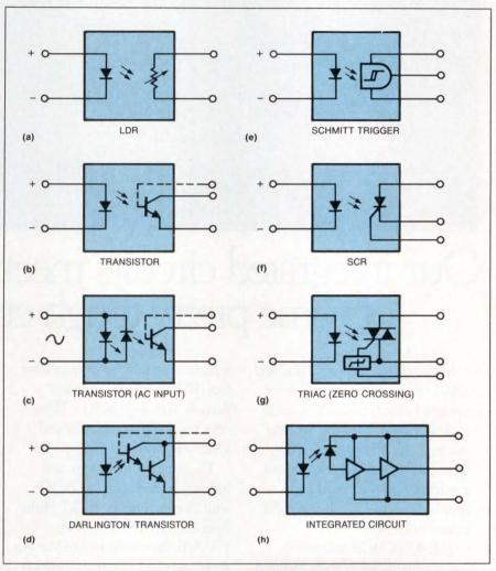
Fig 1—Optocouplers come in a wide variety of types. The primary differences show up in the output stages, which include, but are not limited to, the types depicted here.
