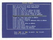
**Analyzer Triggers.** Commonly used triggers can be selected quickly from a list of standard and user-defined triggers.
