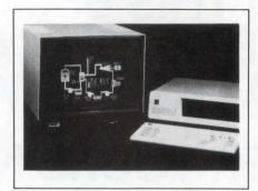
resolutions from 640×350 640×480 pixels as well as other resolutions in the 20- to 33-kHz range. The preconverged CRT has a trio dot pitch of 0.31 mm. The vertical scan frequency ranges from 40 to 100 Hz. The video bandwidth is 65 MHz and the user controls include power, brightness, and degaussing. The TTL inputs provide a color palette of 16 out of 64 colors. The monitor is available in a 19-in, metal enclosure or a RETMA standard 19-in. rack mount. From \$1587.
