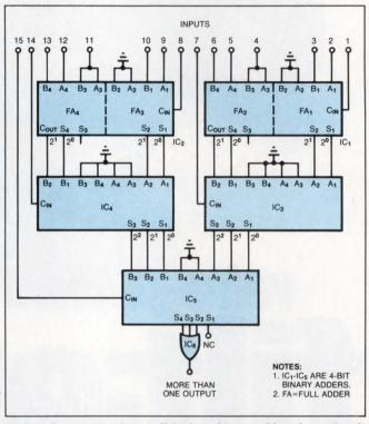
Fig 1—By counting in parallel, these binary adders determine the number of active inputs among a group of 15. The OR gate indicates whether more than one is active.
