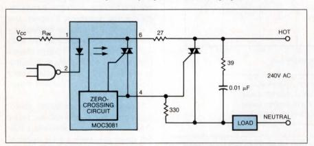
Fig 4—Optocouplers are commonly used to isolate high voltages from sensitive input circuits. This triac-output type from Motorola switches power to a load connected to a 240V ac line. The MOC3081's blocking-voltage rating is 800V.
