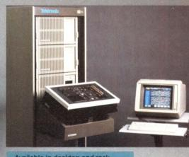
Available in desktop and rackmount versions, the DAS9200 mainframe can be augmented with up to three expansion mainframes for a total of 28 card slots.
