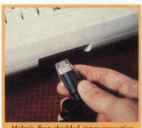
Molex's first shielded interconnection system, SEMCONN, provides protection from electrical noise.
