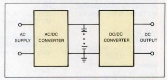
Fig 5—A more reliable UPS structure eliminates the dual powerconversion circuitry seen in Fig 4. This architecture eliminates the need for large electrolytic capacitors that would otherwise be required for hold-up purposes.
