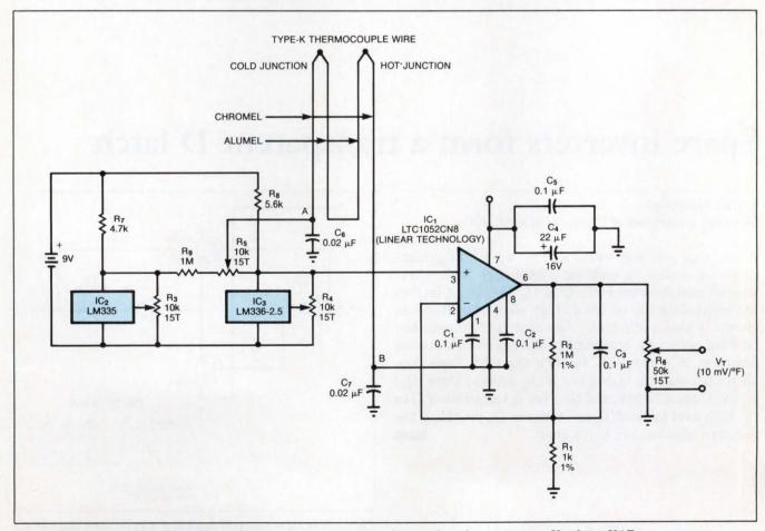
Fig 1—This circuit adds a linearizing voltage to the thermocouple voltage and produces an output  $V_T$  of 10 mV/ $^\circ$ F.
