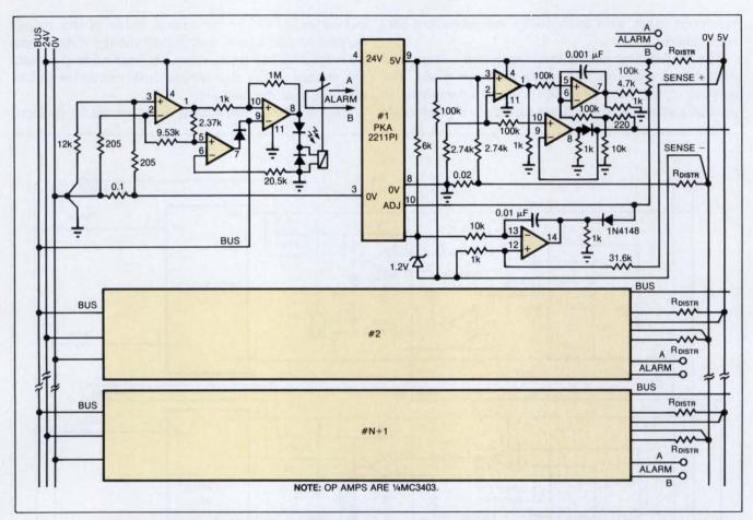
Fig 8—Current-sensing circuitry on the outputs of the dc/dc converters provides an equitable sharing of the load current. This configuration balances the load requirements for the converters to within 5%.
