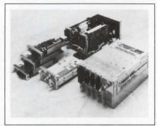
dual-, and triple-output plug-in power modules. All outputs are independent and floating, and can be configured for either positive or negative output levels. The outputs use fully isolated MOSFET switching regulators to achieve high conversion efficiency in a small package—the power density measures 3.4W/in<sup>3</sup>.
