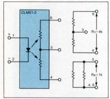
Fig 7—This optocoupler has an LDR as the detector. You can set the reference resistance of the Clairex CLM51-2 at 1, 2, or  $4 \text{ k}\Omega$ . By varying the LED current from 0.1 to 10 mA, you can vary the reference-resistance value over a 10:1 range.
