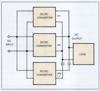
Fig 6—A redundant system built with parallel dc/dc converters connects directly to the load without the need for ORing diodes. This is a reliable configuration, thanks to the use of small ceramic filter capacitors in the converters' outputs.
