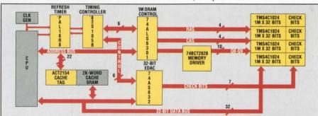
**High-speed memories** can be designed with less effort and implemented more cost-effectively by using TI's family of universal memory-management ICs. These devices, all of which are contained in TI's Memory Management Design Kit, will work with and enhance almost any high-speed processor.
