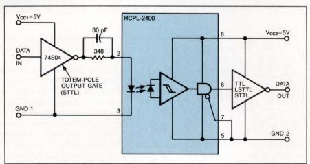
Fig 5—Designed for use in high-speed logic systems and computer-peripheral interfaces, the HCPL-2400 from Hewlett Packard has a typical data-transfer capability of 20M baud. Depending on operating conditions, the device can achieve speeds as high as 40M baud.
