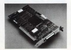
initializes the controller without necessitating the loading of software drivers. The unit is compatible with display matrices of 640×200, 640×400, and 720×350 pixels.
