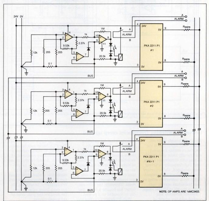
Fig 7—Supervisory circuits sense the input currents to the dc/dc converters and trigger an alarm when a fault is detected. The converters in this configuration typically share the load current in a 3:2 ratio. If a ratio exceeds 6:1, an alarm indicates a fault condition in the appropriate converter.
