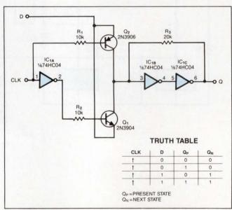
Fig 1—This transparent D latch operates on the clock signal's rising edge. Operation is transparent when the CLK input is low.
