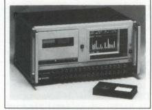
data for 3 hours and 28 minutes with a 39-dB S/N ratio. If the unit is operating in the optional direct-record mode at the maximum tape speed, the bandwidth extends from 200 Hz to 150 kHz with a 30-dB S/N ratio; if the unit is running at the slowest tape speed in the same mode, the bandwidth extends from 100 Hz to 2.35 kHz with a 26-dB S/N ratio. The vendor offers the unit with an option that enables it to perform PCM recording that conforms to IRIG 106-80. \$35,750.
