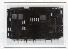
ler supporting three direct and eight multiplexed channels, four serial I/O channels, a synchronous or asynchronous LBX interface, and an SBX connector. It also includes two 28-pin EPROM sockets, a parallel I/O port, programmable timers, and Multibus interface and priority interrupt logic. One of the four I/O ports can be configured as either an RS-232C or an RS-422/449 port. RMX86 and RMX286 operating systems are available. 2M-byte version, \$2035; 4M-byte version, \$2980 (100).
