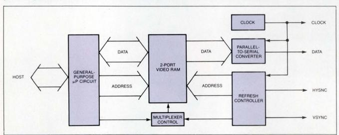
Fig 3—Although this low-end smart controller eases host-overhead tasks, it must still implement all the drawing algorithms in software and handle all communications with the host.
