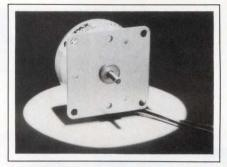
ty requirements. The holding torque specification for the PM motors ranges to 12.4 oz-in. and the step angle is 7.5°—48 steps per revolution. Noncumulative step-angle tolerance equals ±0.5°. The motors feature permanently lubricated bronze sleeve bearings. Versions are available for unipolar or bipolar operation from supply voltages of 5 or 12V dc. \$7.65 (500) for bipolar version. Delivery, 4 to 12 weeks ARO.
