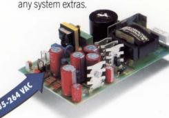
For small to medium systems, check out the NFS110 series 110 watt switchers. The +12V output will deliver up to 9 amps to start disk drives. The small 7.0" x 4.25" x 1.8" size delivers more than 2.0 watts per cubic inch.
