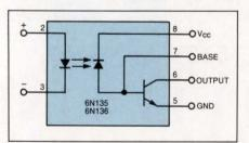
Fig 6—The 6N135 and 6N136 optocouplers are JEDEC registerd and UL approved. The 6N135 is useful for TTL/CMOS and TTL/LSTTL applications; the 6N136, for TTL applications. The separate biasing pin for the photodiode reduces the transistor's collector-base capacitance, which speeds operation by a factor of 20 to 100 compared with conventional phototransistors. Both types are available from a number of suppliers, including Texas Instruments, General Electric, General Instrument, and Hewlett Packard.
