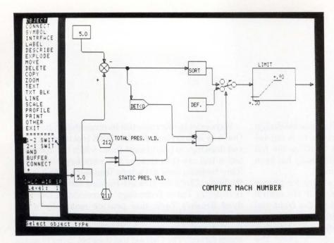
CASE toolsets such as the Excelerator from Index Technology are well-suited to embedded, real-time system design. The toolset's notation enables the portrayal of synchronous vs asynchronous events.
