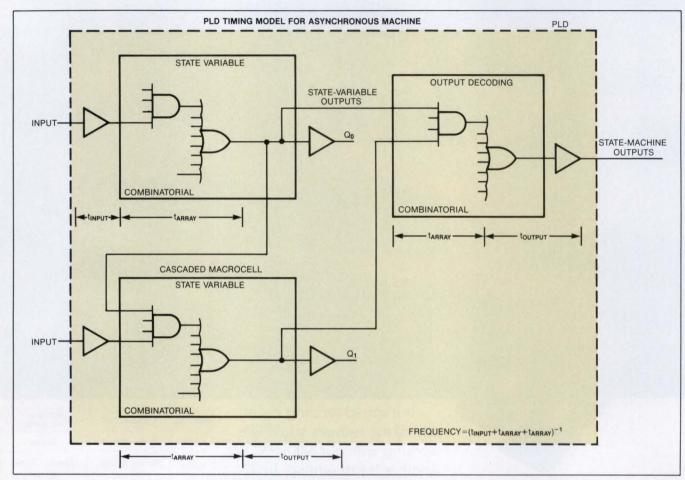
Fig 4—When you use this PLD timing model to calculate assignments in Fig 2b, these transition equations result for  $M_3$ .  $M_4$  is a Moore machine.
