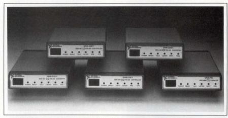
enable you to control the IEEE-488 bus from any computer's serial port without using special software. The units can act as normal or extended talkers and listeners. They support serial and parallel polling, service and pass/receive-control requests, and can be remotely programmed in
