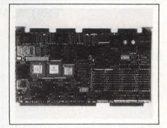
interrupt support, and a full master/slave interface to Multibus I. Optional features include a 68881 or 68882 floating-point coprocessor, and a time-of-day clock with battery backup. The board runs on Unix System V.3, Ready Systems' VRTX real-time executive, and Microware's OS-9 operating system. 4M-byte dynamic RAM version, \$4995.
