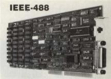
IEEE-488, PARALLEL, and SERIAL PORTS PLUS 4M BYTES of MEMORY
