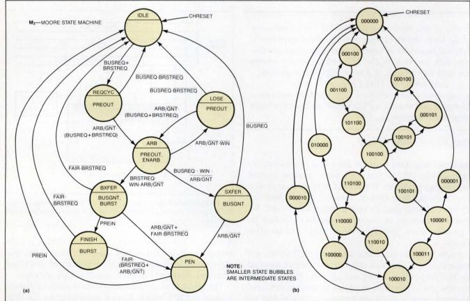
Fig 2—The state-transition-diagram in a is the formal definition of the bus-arbitration handshake for the IBM Micro Channel bus. The diagram in b has an extra intermediate state so that the  $M_s$  state machine will operate without glitches. Note that  $M_s$  requires six state variables, instead of only three, to specify the eight required states. The extra variables are needed to satisfy the requirement that each state transition change only one state variable.
