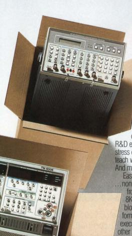
logarithmic and arbitrary sweeps, with any sweep usable in continuous, triggered, gated or burst mode. Users can receive instant frequency readout of breakpoints, notches, or response anomalies.
