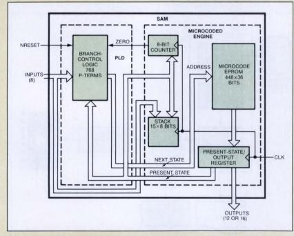
Fig A—The EPS448 SAM (stand-alone microsequencer) has a 768 p-term program-mable-logic block for selecting one of four state-machine branches per state. Operating as a bit-slice processor does, the SAM also includes 16k bits of microcode/state EPROM, an 8-bit loop counter, and a 15-level stack.
