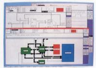
The Concept Express Design System's highly productive logic tools and silicon compilers were used to develop this very-large-scale ASIC. It incorporates a 2901 datapath, RAM, ROM,
