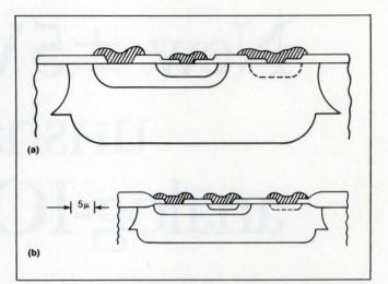
Fig 1—The need for high breakdown voltages to withstand  $\pm 15V$  dc supplies has meant that analog ICs need large structures (a). The smaller structure (b) shows the shrinkage possible with  $\pm 5V$  supplies. The smaller structure is not a direct scaling of the large one, but includes refinements such as partial oxide isolation.
