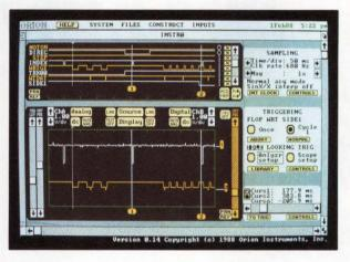
Logic timing analysis (top) of entire sequence for writing data to a floppy disk. Scope simultaneously displays detailed amplitude and multichannel timing information (bottom).
