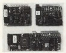
SBX ANALOG I/O MODULES. Up to 16 analog inputs and 8 analog outputs w/12 bit resolution on one card. Throughput rates from 3 kHz to 59 kHz. TTL or CMOS. Nonintelligent or intelligent w/FIFO I/O buffer and many preprogrammed modes of operation. Input filters, prog. gain amp, sample-hold.
