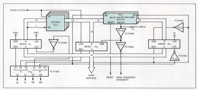
Fig 1—This content-addressable memory accepts a data word in  $IC_1$ . The counter,  $IC_{47}$ , then begins cycling the RAM through all of its 8k addresses (in 409.6  $\mu$ sec max) until the RAM finds a matching data word. The RAM then latches the address of the matching word into  $IC_2$  for reading by the system  $\mu P$ .
