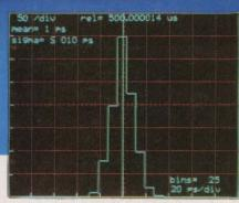
The SR620 provides graphic display of histograms and strip charts on any X-Y oscilloscope. With Autoscale and Zoom, graphics can be easily scaled. Attach a dot matrix printer or an HP-GL plotter and obtain hardcopy of any graph.
