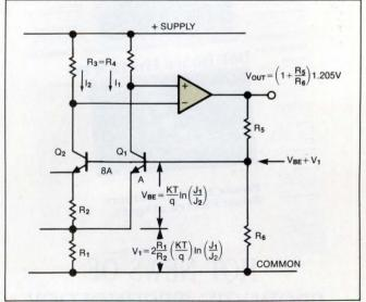
Fig 6—A bandgap voltage reference generates the sum,  $V_{BE}+V_{I}$ , in which the two voltages have equal and opposite temperature coefficients. The amplifier then raises the sum to a more convenient voltage level
