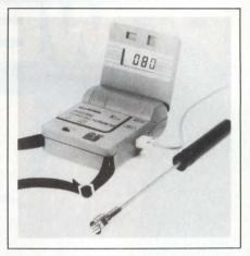
12 oz and measures from -58 to +1999°F and -50 to +1350°C. Its resolution is 1°F or C, and its accuracy equals  $\pm 0.2\%$  of reading  $\pm 1$  digit. A kit is available that includes the meter, a general-purpose temperature probe, and a carrying case. The meter, \$159; the kit, \$219.
