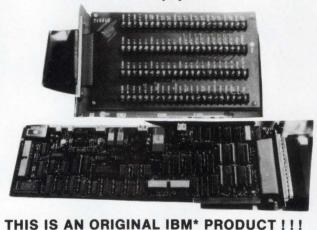
**ACQUISITION** AND CONTROL ADAPTER provides an easy to use interface for accessing the **ANALOG** and DIGITAL I/O. Integrates analog.
