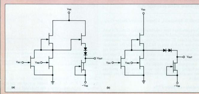
Fig A—Five 2-input NOR gate configurations—the BFL (a), the FETL (b), the CEL (c), the DCFL (d), and the SCFL (e), for GaAs logic circuits exhibit tradeoffs between speed, power, complexity, and manufacturability.
