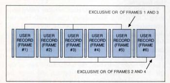
Fig 5—Redundant data lets you reconstruct damaged frames. On this QIC-100 tape, which has an interleave of 2, block 1 contains user-data frames 1 and 3; each byte of frame 5 contains the exclusive OR of the corresponding bytes of frames 1 and 3, and allows you to reconstruct damaged bytes in those frames.
