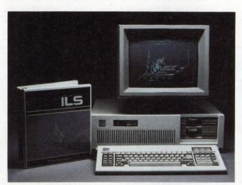
You can view your data in a variety of ways by using PC software that provides data analysis and graphic display. This 3-dimensional spectral display, for example, was generated by the \$2495 Interactive Laboratory System (ILS) from Signal Technology Inc.
