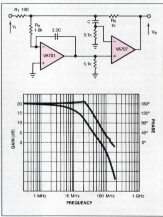
Fig 4—Op amps optimized for ±5V operation yield a composite amplifier with a gain of 20 dB and a bandwidth of better than 30 MHz. They can replace open-loop video amplifiers designed with discrete components, and they offer advantages in linearity, size, and power dissipation.
