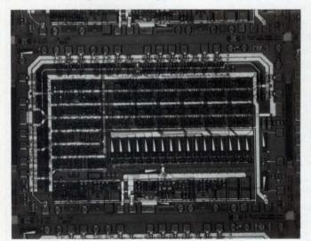
Fig 3—This developmental 12-bit,  $\pm 5V$  ADC integrates a DAC, successive-approximation register, control logic, and voltage reference on a 17,000-mil $^2$  die. Comparable devices using  $\pm 15V$  supplies occupy 40,000 mil $^2$ . The prototype device's conversion speed improves from the 10 to 25  $\mu$ sec typical of high-voltage ADCs to less than 2.5  $\mu$ sec.
