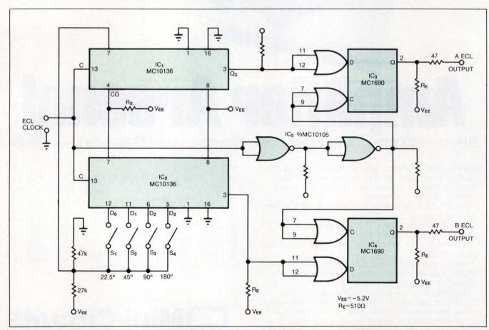
Fig 1—This high-speed ECL circuit develops a pair of phase-shifted square waves suitable for calibrating phase meters. By setting switches  $S_{1:4}$ , you can add programmable delay to the signal path through  $IC_2$ .
