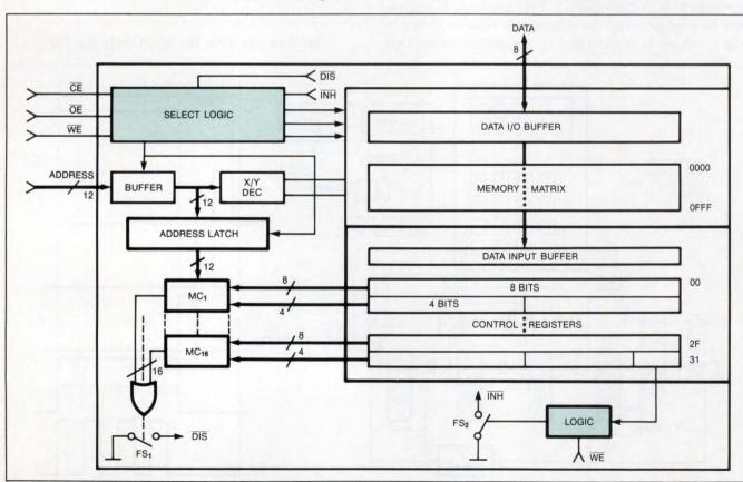
Fig 1—Adding a set of control registers and magnitude comparators to an ASIC that has a memory element can render the memory immune to data pirating. The control registers contain unused memory addresses. If a pirate attempts to access one of these unused program locations, the magnitude comparator sets a programmable switch that permanently disables the ASIC's select logic.
