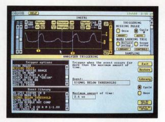
SELECT triggering on a rare event. Using Trigger Options and Event Library from the popup panel (at bottom), a trigger is selected to capture a dropout occurring when a disk drive index signal is below threshold for too long.
