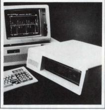
occur at rates as high as 10 MHz. A ring buffer that can hold 1M samples is standard; you can expand it to hold 2M samples. The A/D converter resolves 12 bits. Programmable-gain amplifiers with 3-MHz bandwidth and programmable offset of 4× full scale precede the converter and provide 31 calibrated full-scale ranges from 50 mV to 80V. You can trigger the unit with a TTL trigger command or from a signal
