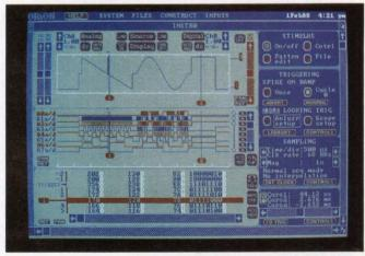
Software that comes with the Omnilab 9240 from Orion Instruments can display time-aligned waveforms from the instrument's digital-storage-oscilloscope and logic-analyzer sections. In addition, the software can store these waveforms on a PC's disk for subsequent analysis.
