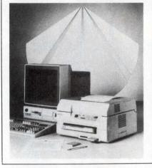
resolution. Also included are ROM-resident and cartridge-based type fonts from Bitstream, one font cartridge slot, a removable paper tray, a 10,000-pg drum set, a 6000-pg toner set, and maintenance and warranty service. Two emulation options for the unit provide graphics capabilities, and HP LaserJet or Epson FX-85 dot-matrix printer emulation. \$1299; emulation op-
