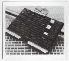
nal-processor board for the Sun-3 workstation utilizes two TI TMS32020 DSP chips and a 16×16-bit multiplier to multiply and accumulate in a single cycle at 10 MIPS. One of the DSP chips acts as a master to control the operational functions, and the other chip acts as a slave to perform arithmetic processing. This arrangement lets the host simultaneously move process integer data with no wait states. A multiported static RAM, with capacities ranging from 64k to 256k
