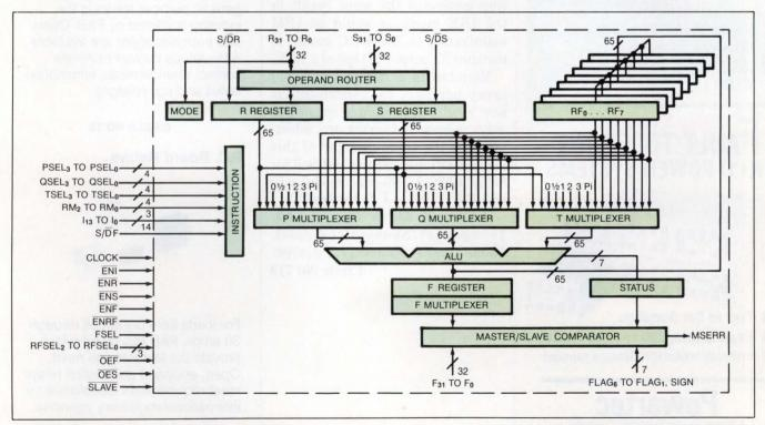
**Providing double-precision accuracy,** the Am29C327 64-bit floating-point-processor IC, offers both floating-point and integer instruction sets and performs single-, double-, and mixed-precision operations.
