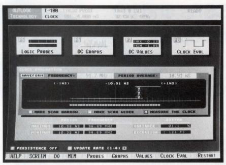
This display presents clock information in graphic and numerical form on the host PC's screen, letting you examine your system's clock during logic-analyzer setup. Similarly informative displays present data about voltage levels and signal activity at the probe tips.
