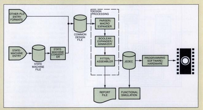
Fig A—State-machine and general-purpose PLD-design software can automate many of the rote tasks associated with state-machine design.
