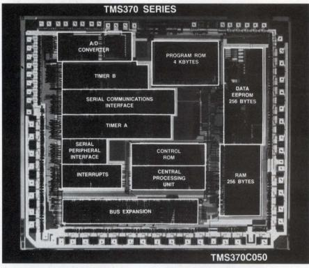
The TMS370 family of 8-bit  $\mu$ Cs allows you to mix and match modules to meet your design goals. You can then configure the TMS370 XDS in-circuit emulator to develop your code before you've even ordered the device.
