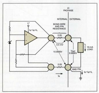
Fig 2—When this reference supplies current to a load, voltage drops inside the package are inside the feedback loop and have little effect on accuracy. The voltage drop across the package's output pin can be significant, however.
