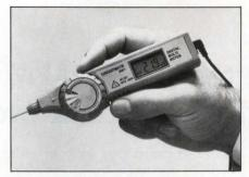
The latest probe-type DMMs, such as this Beckman DM71, now feature a rotary dial for selecting ranges instead of the tiny pushbuttons employed by earlier versions.
