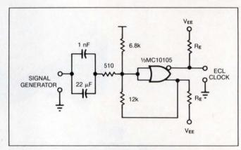
Fig 2—You can slave the circuit in Fig 1 to your system's signal generator with this simple Schmitt trigger.
