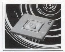
section. The circuit then adds the four weighted results in combinations that you select. The final scaled and combined results are available from two parallel, 3-state output ports. The output is either 2's complement or unsigned magnitude. The device is available in a 68-pin pin-grid-array package. 17-MHz version, \$61; 20-MHz version, \$73 (1000).
