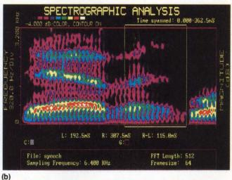
The excellent graphic-display capabilities of today's PCs allow laboratory-automation software to present data in a variety of ways so you can pick a format that best matches your data. Hypersignal-Plus from Hyperception can display 3-dimensional spectrographic data as a series of 2-dimensional plots (a) or, by using color, can add the third dimension to a flat screen display (b).
