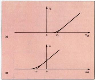
Fig 1—Because an n-channel enhancement-mode device (a) draws no drain current  $(I_D)$  when the gate-to-source voltage  $(V_{GS})$  is 0, the device is normally off. In contrast, an n-channel depletion-mode device (b), which draws drain current when  $V_{GS}$  equals 0, is normally
