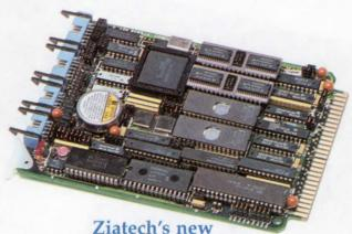
STD Bus ZT 8809 Single Board System for OEM applications.
