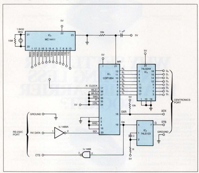
Fig 1—The CDP-1854 UART assembles serial RS-232C data into bytes for a Centronics port.  $IC_2$  provides a baud rate that matches the RS-232C transmission rate, and  $IC_3$  buffers the data byte to the Centronics port. Signals DA and  $\overline{DAR}$  control the timing of the two ports.
