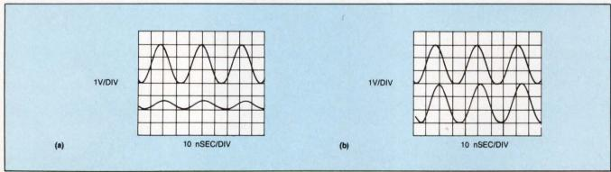
Fig 1—These input (top) and output (bottom) waveforms show the frequency-response improvement that results when you modify the LH0002 current amplifier (whose response is shown in a) by adding the external components in Fig 2. The improvement illustrated in b results when  $R_S=1$  k $\Omega$ ,  $R_L=50\Omega$ , and frequency equals 30 MHz.
