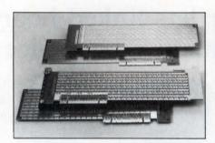
all ground and signal connections are made before power is applied to the board, the 5V edge-connector fingers are reduced in length so that they are the last to make contact. All the edge connectors are gold plated.
