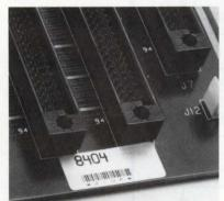
Advanced statistical process controls provide close computer monitoring of production. Bar code system tracks individual assemblies in real time.
