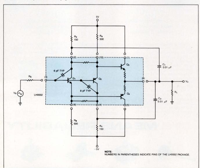
Fig 2—You can add components to extend the bandwidth of an LH0002 amplifier. This circuit increases the input-stage bias currents and bootstraps the amplifier's input capacitance.
