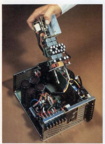
A 600W supply that uses a separate assembly for a 150-kHz converter (Kepco Inc)
