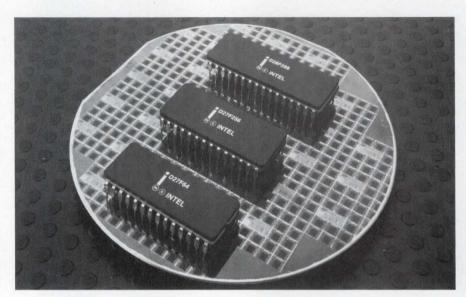
100- $\mu A$  max standby current. The devices also exhibit a failure rate of less than 0.01% for 100 erase/program cycles. They sell for \$19.90 (10,000).
