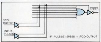
Fig 3—Using a PLD with 3-state outputs, you can implement Fig 1's circuit. Just connect the pulse source to a gate's output enable and the VCO's output to the gate's input. Because these PLDs have inverted outputs, you'll have to invert some signals.
