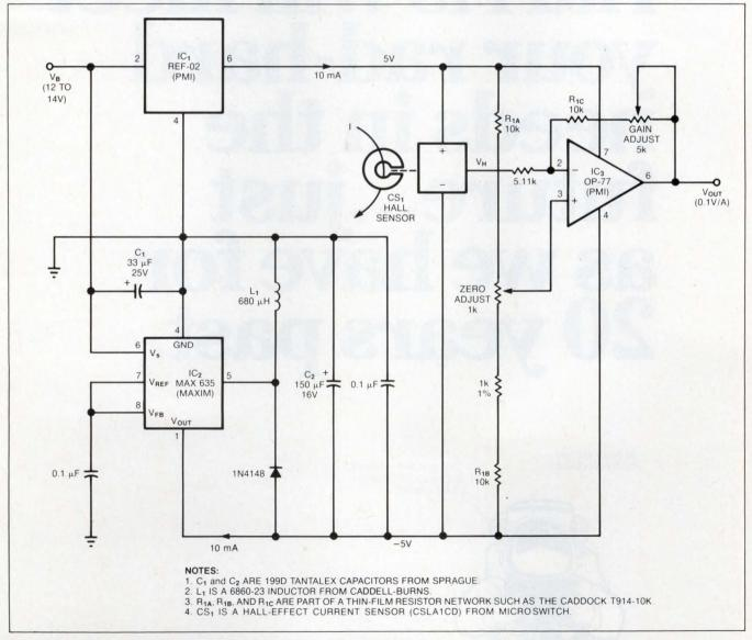
Fig 1—This circuit's Hall-effect current sensor  $CS_t$  enables  $V_{OUT}$  to register dc current at IV per IOA.
