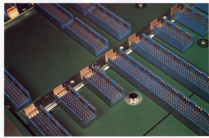
Backplane with modular connectors (Teradyne Connector Systems)
