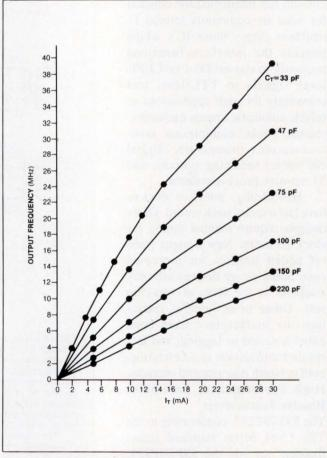
Fig 2—This graph illustrates how different values of Fig 1's timing capacitor  $C_T$  provide different output frequencies for a given value of input current.
