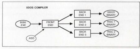
directly execute the program on the Unix system, because the XDOS utility maps MS-DOS, MS-DOS BIOS, and hardware system calls to Unix calls, and also manages calls that invoke MS-DOS data structures.
