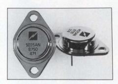
a  $C_{\rm ISS}$  of 2400 pF. You can also obtain units with 800-pF  $C_{\rm ISS}$ , 180-pF output capacitance ( $C_{\rm OSS}$ ), or 60-pF transfer capacitance ( $C_{\rm RSS}$ ). The dies for hybrid applications
