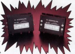
The KZ 400 delivers an impressive 80% typical efficiency and has a fixed switching frequency of 200 KHz. Line/load regulation specifications are ±1% main channel and ±5% auxiliaries. The unit is available in PC board and side mount models.
