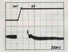
AD744 Settling Characteristics 0 to + 10V Step
