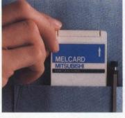
(SRAM, OTPROM, masked ROM), upgrade and downgrade memory density, and change data width (8 bits, 16 bits). All with an extremely rugged device that's the size of a credit card (86mm x 54mm x 3.4mm).
