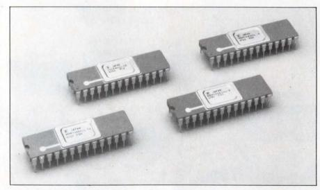
it's compatible with 100K ECL products. The devices come in 28-pin ceramic DIPs. The  $1k\times4$ -bit units cost \$55 (1000); the  $4k\times4$ -bit devices sell for \$75 (1000).
