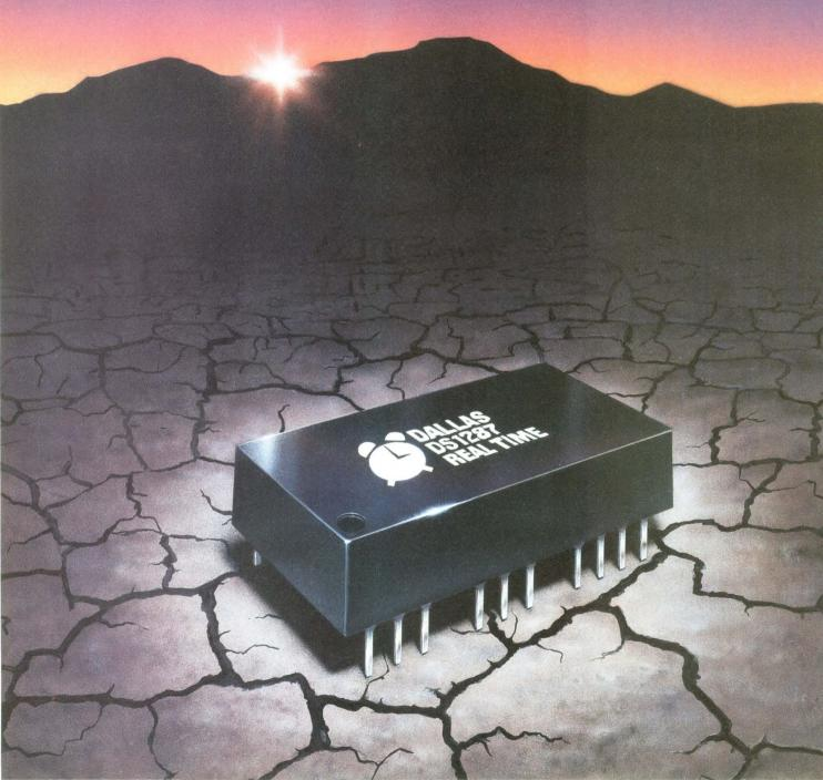
allas Semiconductor clock/calendars are so efficient that they give personal computers virtually permanent timekeeping, yet eliminate 19 components from the assembly of IBM AT or PS/2 compatible computers. The DS1287 Real Time
