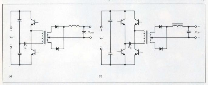
Fig 1—Most high-power switching supplies use either a half- or a full-bridge configuration. The half-bridge circuit (a) is the most popular for transistor currents to about 20A. At higher currents, designers usually switch to the full-bridge circuit (b), which nearly doubles the power output. Bridge circuits can use transistors that have about half the breakdown-voltage rating required for flyback or push-pull circuits.
