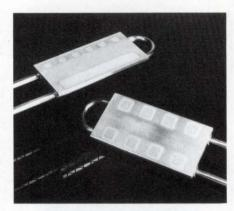
Part number 180-10-6, for example, is a 3×6-in. plate, with 0.01-in.-thick ceramic pads cooled by water. When the attached components are dissipating 400W, and the water is flowing at 1 gal/minute, the plate's
