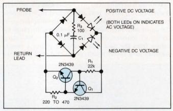
Fig 1—This simple test probe indicates ac or dc voltage over a 4 to 220V range. The current source  $(R_1, R_2, Q_1, \text{ and } Q_2)$  ensures a constant current in the LEDs for any acceptable test voltage.
