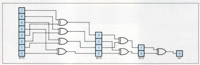
Fig 1—You can quickly test 8-bit character codes for parity by emulating this hardware in a software routine.
