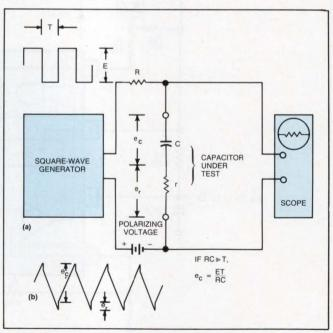
Fig 1—You can quickly determine a capacitor's series resistance by using the circuit in **a**. By looking at the relative magnitudes of  $e_{\tau}$  and  $e_{C}$  (**b**), you can decide whether the capacitor's resistance lies within acceptable limits.
