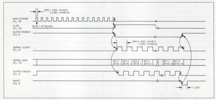
Fig 2—These waveforms for the Fig 1 circuit illustrate the serial transmission of one 16-byte block of data
