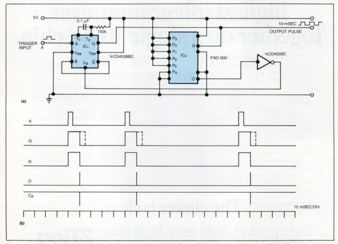
Fig 1—This circuit (a) lets you set precise pulse widths (b) that are independent of component aging, power-supply variations, and temperature. The monostable multivibrator ( $IC_1$ ) is configured in the nonretriggerable mode, and the RC time constant is greater than the desired pulse width.
