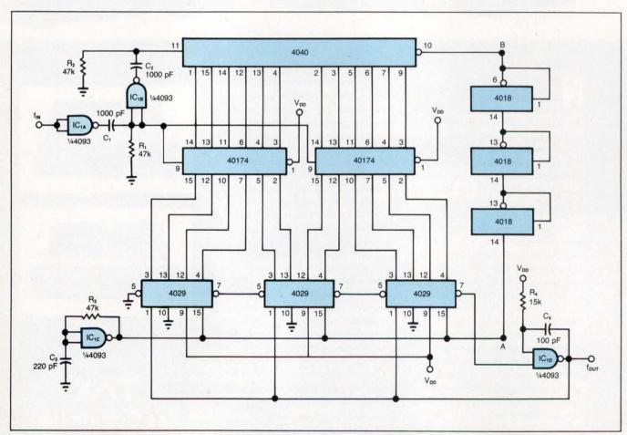
Fig 1—You can multiply frequency fin from eight to 1000 times by using 10 CMOS ICs and several passive components.
