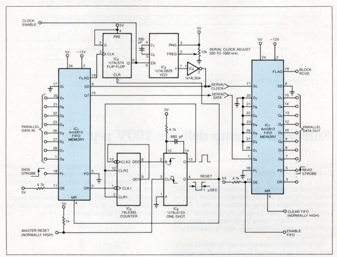
Fig 1— $IC_1$  provides a 16-byte buffer memory for parallel-input data and formats the data for serial transmission to  $IC_7$ .  $IC_7$  then reorganizes the data in byte-parallel format.
