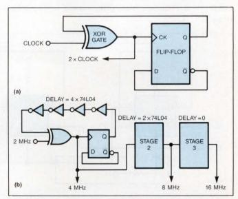
Fig 1—A simple circuit can double the clock input frequency (a). However, you cannot cascade such doublers unless you insert appropriate delays in the feedback paths as in b.
