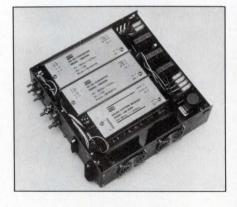
and -12V outputs. Except for the 2-output version, whose line- and load-regulation spec is 1%, the modules feature 0.3% typ line and load regulation. The units' output ripple is 1% of output (max) over a 20-MHz bandwidth. The single-output modules can share current when operating in parallel.
