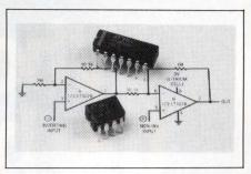
250-pA-max offset current, 0.4  $\mu$ V/°C offset voltage drift, a 200-kHz gain-bandwidth product, and a 0.07V/ $\mu$ sec slew rate. The 1/f corner of the voltage noise spectrum is 0.7 Hz. This low frequency corner permits a voltage noise specification of 0.6  $\mu$ V $_{\mu}$  $\mu$ p and a current noise specification of 3 pA $_{\mu}$  $\mu$ p over the 0.1-Hz to 10-Hz frequency range. The outputs can source and sink 5 mA of load current. LT1078, \$2.80; LT1079, \$3.50 (100).
