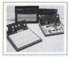
into DIP-spaced breadboard socket connections. The boards come in four models that offer from 810 to 2940 tie-points. Each model includes an area containing both distribution and terminal strips that accommodate all DIP sizes, lead components, and wire gauges of 20 to 29 AWG. The phosphor bronze, nickel-plated contacts provide a 3-m $\Omega$  initial contact resistance and a 10,000 in-outcycle min lifetime rating. Each breadboard features four multipurpose binding posts. \$16.95 to \$59.95.
