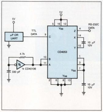
Fig 1—Two inexpensive ICs convert serial TTL data to a bipolar format suitable for transmission on RS-232C lines.
