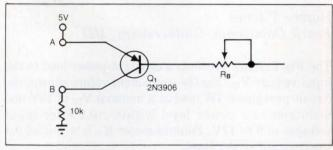
Fig 2—In this test configuration,  $R_{AB}=0.061R_B\pm2\%$  as  $R_B$  varies from 34 to 825  $k\Omega$
