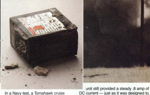
In a Navy test, a Tomahawk cruise missile exploded into a concrete building. When the dust settled, little remained but gravel and fragments of casing.
