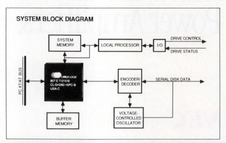
late the IBM Task File for the PC/AT and the IBM Command Descriptor Block for the PC/XT. The chip can sustain a 2M-byte/sec transfer rate to the disk and a 4M-byte/sec transfer rate on the host
