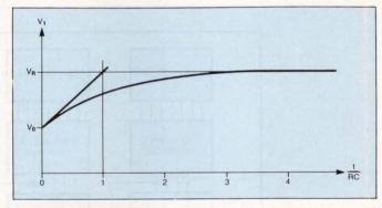
Fig 3—This curve shows the variation of  $V_1$  following closure of  $S_1$  and caused by the charging of capacitor  $C_1$ .
