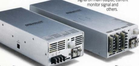
Low profile cases only 5" wide by 2.75" high permit convenient stacking of the supplies. Power density is up to 2.4 Watts per cubic inch, and all models are efficiently cooled by a miniature internal ball bearing DC fan.
