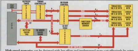
High-speed memories can be designed with less effort and implemented more cost-effectively by using Tl's family of universal memory-management ICs. These devices, all of which are contained in Tl's Memory Management Design Kit, will work with and enhance almost any high-speed processor.
