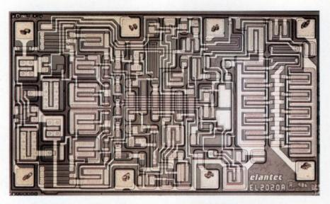
Micrograph of low-cost, 50-MHz op amp (Elantec Inc)
