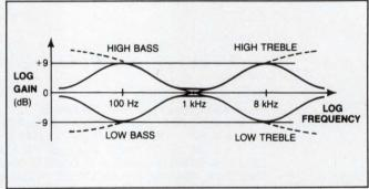
Fig 2—The frequency response of the dual-filter tone control (Fig 1) shows little effect at 1 kHz but  $\pm 9$ -dB variation in the treble and bass regions. For comparison, the dashed lines show the response of a Boxandal tone control.
