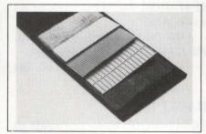
FCC regulations for EMI/ESD protection; it features a full 360° wrap of extended copper shield. Dielectric PVC material, located above and below the cable inside the shield, maintains precise shield-cable spacing, thus providing the high-impedance and low-capacitance values.
