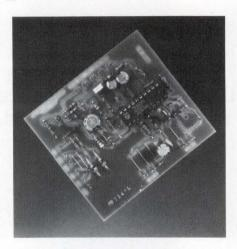
The IC has an interface for a dialer, and it produces an earpiece-confidence tone during DTMF dialing. A Mute input allows you to disable speech transmission during DTMF or pulse dialing. The DTMF amplifier has a typical gain stability of ±0.2 dB over the device's -25 to +75°C operating-temperature range. It also has automatic gain control, which allows you to operate
