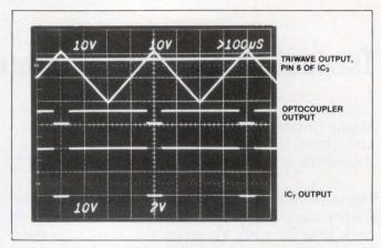
Fig 3—Looking at these waveforms, you can see how the Fig 1 circuit uses PWM to encode  $V_{IN}$  as a duty cycle.
