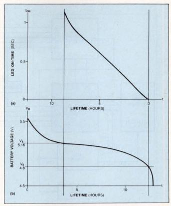
Fig 2—The calculated on-time in seconds for the LED in Fig 1 corresponds to the battery's remaining life in hours, based on a  $100\Omega$  load (a). The curve in **b** shows the measured rate of discharge for a NiCd battery (four Varta RS600 cells loaded with  $100\Omega$ ).
