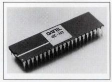
8-bit parallel outputs are buffered and have open-emitter arrangements. The chip dissipates 1.2W and has an integral and differential linearity of ±½ LSB over its operating range. You can select one of the following output codes: binary, complementary binary, 2's complement, and complementary 2's complement. The chip operates with an external clock and reference source, and comes in a 42-pin DIP. Its operating temperature ranges from −20 to +100°C. \$550.
