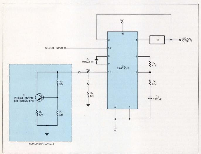
Fig 1—By connecting the nonlinear load Z to pin 11 of the PLL chip  $IC_1$ , you can extend the PLL's frequency range by a factor of 50, as compared with that possible by using a fixed resistor  $(R_i)$ .
