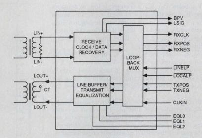
The receiver performs clock and data recovery on the incoming signal, and then converts them to TTL-level. This is accomplished through the use of a trimmed analog phase locked loop and an external precision resistor. No other tunable or precision components are required. Easy interfacing to deframer circuitry is achieved through the use of standard TTL-level receive outputs.
