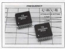
output resistance over the entire resistance range. An onboard data latch lets you set predetermined attenuation settings. It operates with power supplies ranging from  $\pm 6$  to  $\pm 15$ V and dissipates 0.5  $\mu$ W typ. The 16-pin hybrid package occupies 1 sq in. of board space. \$39.50.
