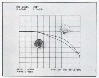
200-MHz, overdrive-protected op amps (Comlinear Corp)
