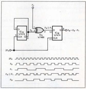
Fig 1—Two ICs generate the frequency difference between  $F_0$  and  $F_1$ .
