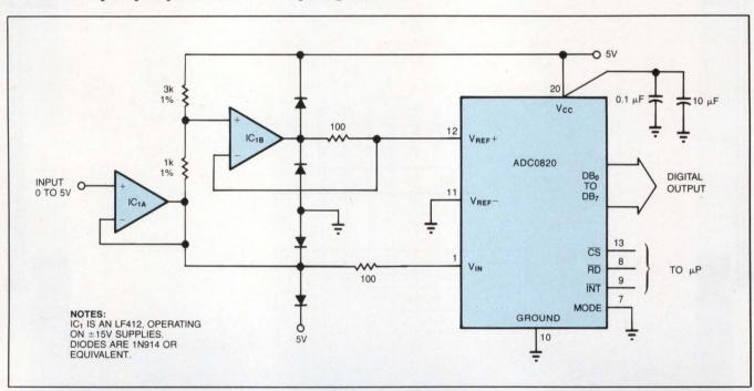
Fig 1—You can increase an A/D converter's apparent resolution by combining the input signal with a fixed reference voltage and feeding this sum to the converter's reference input.
