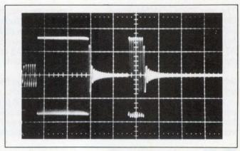
Fig 2—Ring duration for an electrostatic transducer is less than ½oth that of a piezoelectric type, allowing easy recognition of an echo that occurs 800 µsec after the transmit pulse begins. Here, scale is 5V/div in the vertical axis and 200 µsec/div in the horizontal axis.
