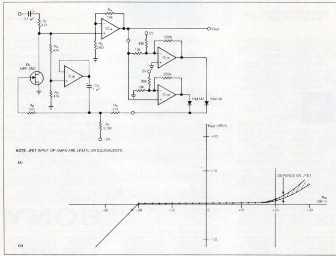
Fig 1—Using a JFET to control input attenuation, this AGC circuit (a) provides a dynamic range of ±20 dBm (b).
