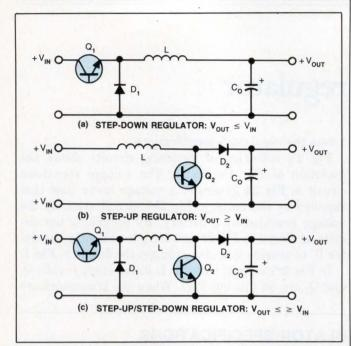
Fig 2—These three switching circuits show the evolution of Fig 1's circuit. The voltage step-down circuit in  $\mathbf{a}$  generates a voltage lower than that supplied by the battery. The circuit in  $\mathbf{b}$  steps up the voltage provided by a battery. By combining these circuits as shown in  $\mathbf{c}$  and using a switching-regulator IC to provide the switching function and  $Q_2$ , you derive the design in Fig 1.
