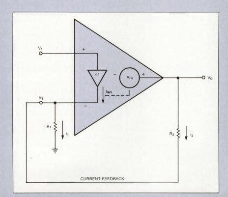
current-feedback op amp—unlike the conventional op amp—the position of the poles (contained within  $D_{(s)}$ ), and hence the bandwidth of the current-feedback op amp, is not dependent on the closed-loop gain. Provided that you keep  $R_2$  constant, you can change the closed-loop gain of a current-feedback op amp—with-
