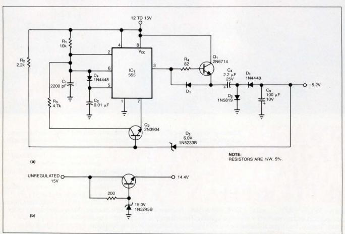
Fig 1—This converter produces -5.2V from a 12 to 15V supply (a). To ensure that the IC doesn't operate above 15V, you might have to use a preregulator (b).
