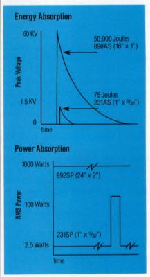
Regardless of the pulse shape, we have the resistor. Our Type SP handles large amounts of power from 60 cycles through VHF. Type AS can absorb huge amounts of energy in millisecond pulses. Type A solves high resistance problems in high voltage situations.
