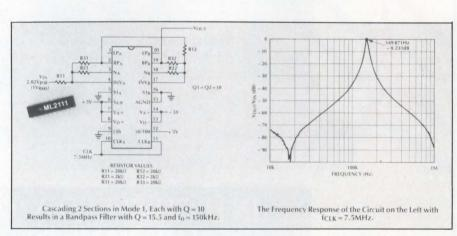
low-offset (15-mV max) voltage amplifier, a voltage summer, two integrators, and control logic. The filters maintain their specifications when operating from  $\pm 5 \mathrm{V}$  supplies with  $\pm 10.0\%$  tolerances. The device can also operate from a single  $5 \mathrm{V} \pm 10\%$  supply at a maximum operating frequency of 100 kHz. An
