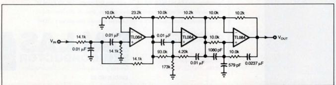
Fig 2—You can achieve a 39-dB stopband and 1.25-dB ripple using this bandpass filter. Scale the capacitor values to change its center frequency.
