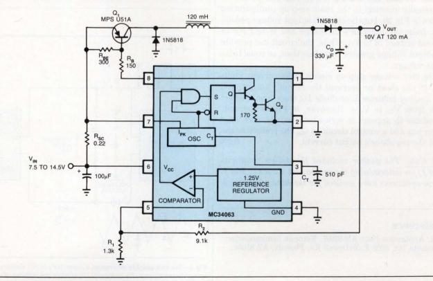
Fig 1—Using a single inductor, a switching-regulator IC, and a few external components, you can build a step-up/step-down switching regulator.
