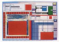
This highly-integrated design combines control logic, a register file, a refresh counter, and five peripheral chips onto a die size of 275 x 315 mils. The logic design, layout, and verification were completed in
