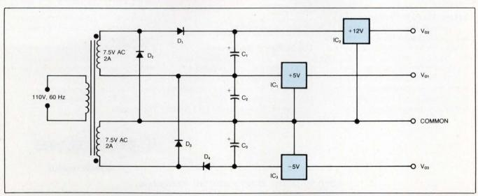
Fig 1—This simple power supply generates three regulated voltages using a minimum of components.
