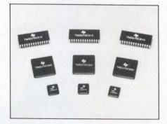
serial peripheral interface, a watchdog timer, a 16-bit timer (on three of the units, two timers are standard), and either 128- or 256-byte data registers. The units use a single 5V supply and can function with a 20-MHz clock. They operate over -40 to +85°C. Chips packaged in 28-pin plastic DIPs or PLCCs cost \$3 to \$7, depending on quantity. Parts housed in 68-pin PLCCs range in price from \$4.50 to \$10.
