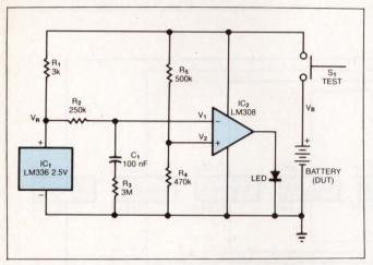
Fig 1—This test circuit checks the remaining charge in a battery; the charge is proportional to the time the LED remains on after you depress  $S_i$ .
