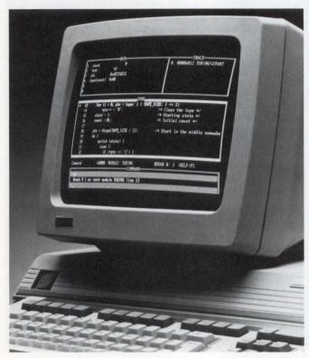
A typical cross-debugger with multiple windows (Applied Microsystems Corp)
