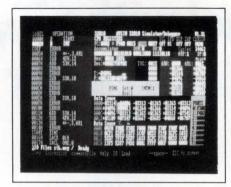
tion stream and the contents of registers, flags, and areas of data memory. You can examine and modify these at any time; by using an Undo key, you can back up, one instruction at a time, through recently executed instructions to determine where an error occurred. You can issue commands either from a menu structure or from a command line. \$379 each.
