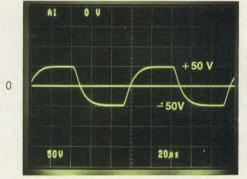
Reproduction of a 10KHz square wave by a Kepco bipolar Power Manager Model BOP 50-2M, which actually has a 20KHz bandwidth in the voltage mode.
