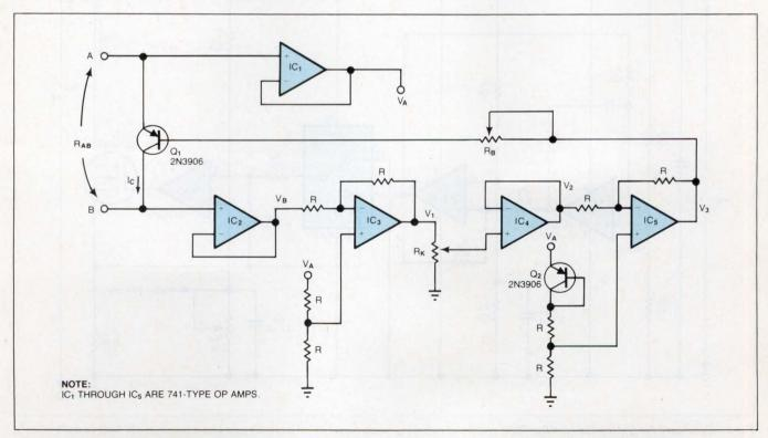
Fig 1—Resistance  $(R_{AB})$  between nodes A and B is a linear function of the wiper positions for potentiometers  $R_B$  and  $R_K$ .
