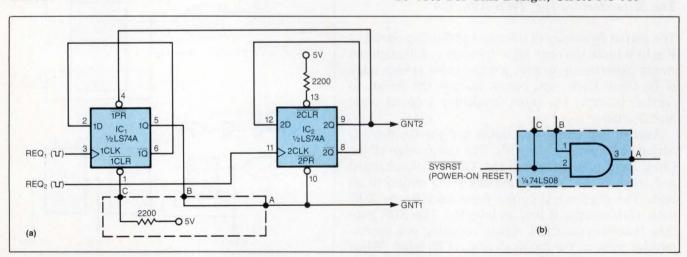
Fig 1—A pair of back-to-back flip-flops can arbitrate access to a shared resource. A master requesting access will be blocked until the second master relinquishes control because each resource-grant flip-flop, when active, engages the other flip-flop's preset input. The AND gate in **b** forces the circuit to a predetermined state upon power up.
