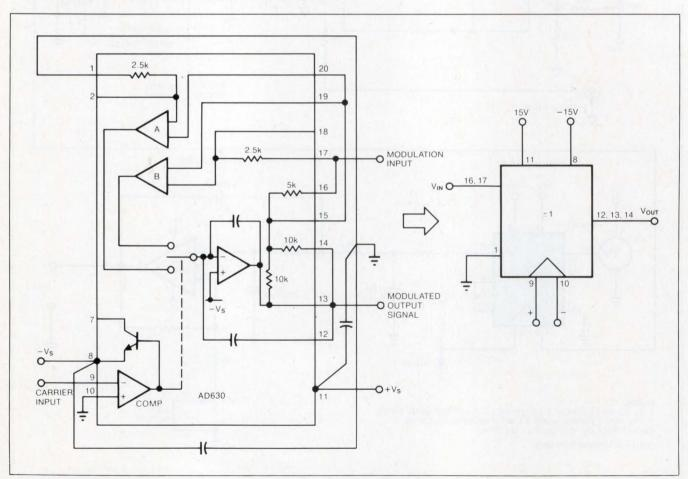
Fig 2—This balanced modulator/demodulator is configured as a ±unity-gain device.
