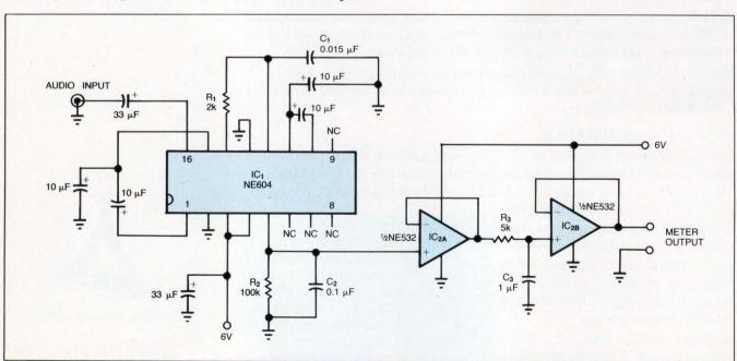
Fig 1—You can measure audio signal levels to  $\pm 1.5$ -dB accuracy using a dual op amp and an FM IF chip (normally used for cellular-radio and other RF applications). Sensitivity is 10.5  $\mu$ V; power consumption is 30 mW.
