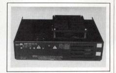
and 15V outputs are provided by a single model, which employs a potentiometer for output selection. The 24 and 50V versions have a potentiometer, which gives you approximately  $\pm 10\%$  control over the output voltage.
