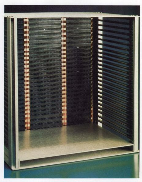
Backplane mounted in a card cage (Teradyne Connector Systems)
