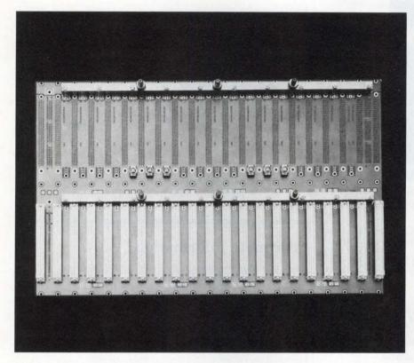
Monolithic backplane with press-fit construction (Bicc-Vero Electronics)
