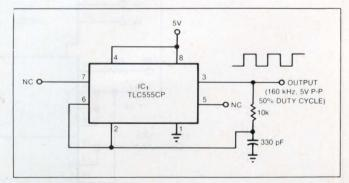
Fig 1—Based on a CMOS version of a 555 timer, this astable multivibrator's output symmetry depends on the tolerance of the internal switching thresholds.
