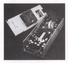
80% min, the vendor claims. The unit specs 0.2% rms max ripple and noise.
