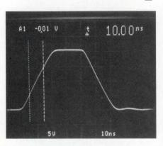
the  $1000\text{V}/\mu\text{sec}$  slew rate. You can power the device from supplies ranging from  $\pm 5$  to  $\pm 17\text{V}$ . Other
