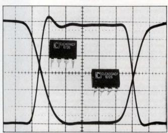
200-MHz, ±5V-supply op amps (Comlinear Corp)
