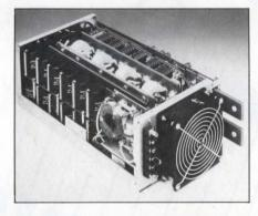
0.1% (whichever is greater) line regulation, and 10 mV or 0.2% (whichever is greater) load regulation; dynamic response of 4% max for a 25%-step load change; 200-µsec output recovery to within 1% of nomi-
