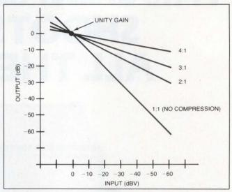
Fig 2—The input/output transfer-function curves of the circuit in Fig 1 show the four possible signal-compression slopes and the unity-gain point for each slope.
