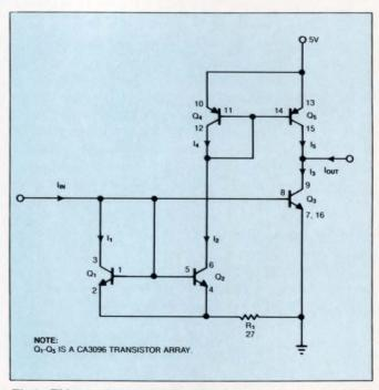
Fig 1—This transistor-array circuit performs square-law amplification of  $I_{IN}$ .
