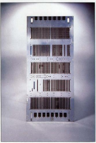
MIL-spec backplane measuring 42×22 in. (Methode Electronics)
