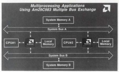
ance state. All the I/O lines go to a high-impedance state upon power-down. The device is available in a 68-pin PLCC or LCC, and it exhibits typical port-to-port delays of 9 nsec. The ports for each of these devices are TTL compatible and can sink 48 mA of output drive current.
