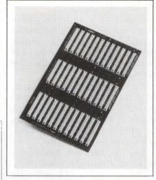
els that require such a configuration. Based on transmission-line technology, the backplane is mechanically compatible with both VME and Sun card cages. It duplicates the Sun backplane and includes the signal busing necessary to implement the Sun proprietary P2 bus. The 5-layer combination microstrip/stripline design provides high-performance operation to 40 MHz. Bus bars facilitate the power hookup and disconnection. \$1275.
