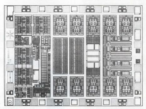
first level to route macrocells and the second to interconnect them. The vendor offers VAX-based and IBM PC-based CAD tools to support IC design with the arrays; it also offers kits of individual components and macrofunctions that you can use to make breadboards of your design. Nonrecurring engineering charges for prototyping are around \$10,000, and engineering for volume production costs about \$10,000. The
