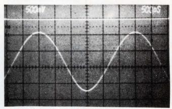
Fig 3—The Fig 1 free-running oscillator furnishes a clean output that varies between -0.5 and -2.25V. Here, the vertical scale is 500 mV/div; the horizontal scale, 500 psec/div. The horizontal line at the top of the display represents the zero level.
