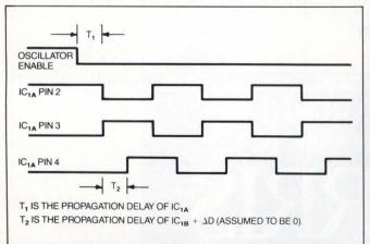
Fig 2—The Fig 1 oscillator always starts in the same state. Either  $IC_{1B}$ 's internal propagation delay by itself or the delay and an optional feedback loop determine the frequency of oscillation.
