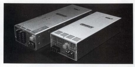
ture a modular design that provides one to seven outputs. Their line- and load-regulation performance is 0.2% or 10 mV max, and their switching frequency measures 100 kHz. The units' efficiency figures range from 70 to 85%. The maximum ripple and noise specs (for a 20-MHz bandwidth) are 1% or 50 mV for the main
