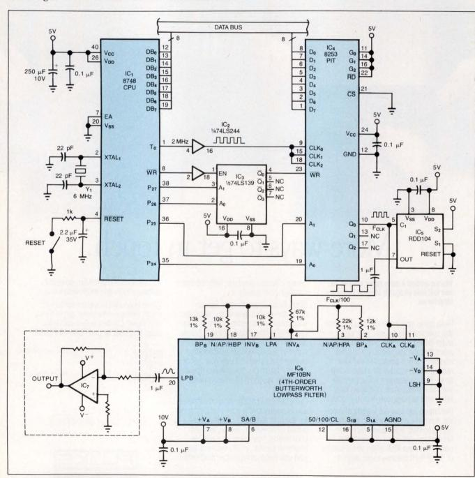
$\label{lem:fig:computer-controlled system} \ produces\ a\ constant-amplitude,\ programmable-frequency\ audio\ output.\ Frequency\ range\ spans\ five\ decades\ to\ 20\ kHz.$
