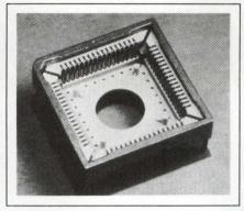
The units feature liquid crystal polymer housings rated for continuous operation at 200°C. You can obtain them with three types of contacts: beryllium copper rated to 200°C, beryllium copper rated to 150°C, and phosphor bronze rated to 125°C.
