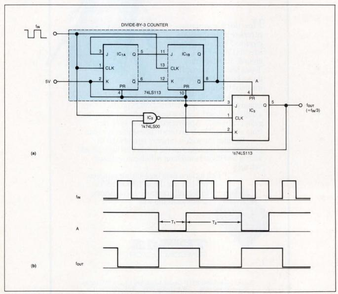
Fig 1—Odd-integer division performed using a divide-by-3 counter (a) produces the asymmetrical waveform (such as the one labeled A in part b), but you can add additional circuitry to generate a symmetrical  $f_{OUT}$  signal.
