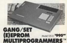
BYTEK's 135 is a SET Programmer, GANG Duplicator, & UNIVERSAL Device Programmer. Programs virtually all 24, 28, & 32-pin (E)EPROMs. RAM expandable to 2MegaByte. Optional support for 40-pin EPROMs, Bipolar PROMs, 40-pin Micros, & (E)PLD/GAL/FPLA
