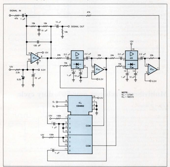
Fig 1—With this circuit, you can select gain-compression ratios of 1:1, 2:1, 3:1, and 4:1 without changing the unity-gain point. By changing inputs  $G_0$  and  $G_1$  of the analog multiplexer, you control the detector current in each half of the NE572 (IC<sub>2</sub>), and, therefore, the gain of each section.
