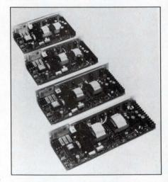
features of the switchers are built-in line filtering, 3750V ac safety isolation, shielded power transformers, built-in overload and overvoltage protection, overtemperature shutdown, remote-sensing capability, vacuum-impregnated magnetics, and fixed-frequency pulse-width modulation. You can opt for a power-valid indicator and for TTL-high or TTL-low power-fail-detection circuitry.
