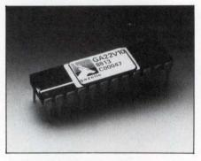
inputs and ten 3-state outputs that you can program for registered or combinatorial data with active-high or active-low polarities. It also has a power-up reset command, a synchronous preset command, and an asynchronous reset mode for statemachine applications. To prevent unauthorized access to the internal configuration, a security link disables the pattern-verification function and the preloading of the registered outputs. The PLD costs \$55 (100).
