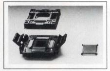
cepts devices with 52, 68, 84, 100, and 132 leads. The hinged-lid socket accepts devices with 84, 100, and 132 leads. The insulation material is polyethersulphone/polyetherimide. The contacts are made of beryllium-copper and feature gold-over-nickel plating. 132-pin socket and carrier, \$92.11 (100).
