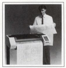
tion drawings on cut-sheet paper and film. The plotter can operate as fast as 30 in./sec. Addressable resolution is 0.005 inches, and accuracy is 0.1% of the distance moved or 0.01 inches, whichever is greater. Two dc-servo motors enhance throughput by providing fast pen positioning, and a look-ahead feature keeps the pen moving at high speed when a line changes direction by less than 45°.
