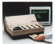
electronics stores device-specific instructions on a 31/2" micro diskette. To update your UniSite 40 with the latest device releases, simply load a new master diskette.
