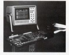
You can select from 13 predefined trigger functions, including edge, glitch, and window triggering. You need only specify the trigger word and timing information to complete the trigger setup. The instrument provides an on-screen graphical display of the trigger conditions in the form of a timing diagram.
