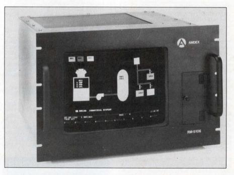
horizontal scan frequencies of 15 to 35 kHz and vertical scan frequencies of 60 to 90 Hz. Automatic synchronization is in accordance with the appropriate video standard. The display consumes 80W and operates over a temperature range of 0 to 55°C. \$1750.
