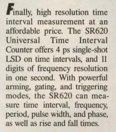
The SR620 has built-in statistical functions, including mean, min, max, standard deviation, and Allan variance for up to 1 million samples. Results may be displayed on the front panel, and graphed in histogram or strip chart form on an X-Y oscilloscope. Hardcopy is directly available on a plotter, printer, or chart recorder.
