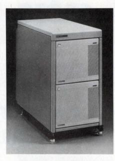
average seek time is 20.5 msec, and the burst transfer rate is 5M bytes/ sec.
