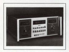
most measurements, accuracy is 0.05% of reading. Besides true-rms voltage and current, the variables measured include real, complex, and reactive "power" (watts, VA, and VARs), watt-hours, VAR-hours, power factor, and frequency. Measurement ranges extend from 4 to 660V, 25 mA to 55A, and 150 mW to 36 kW. An IEEE-488 interface is optional. \$7500.
