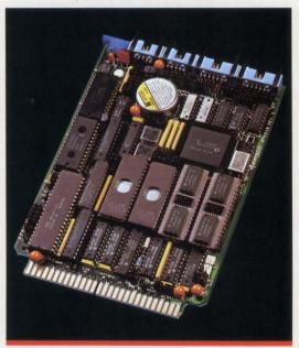
Ziatech's NEC V20-based STD computer (ZT 8808, above) or an NEC V50-based computer (ZT 8816) provide processing power for the new ZT 1000 (see photo page one).
