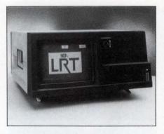
nent, fall time, and bit rate) and also measures the network's bias voltage. By examining the framing information to determine each packet's source, the analyzer can correlate most of these cable measurements with particular network nodes.
