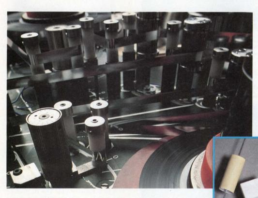
Automated high-speed winding operation for DC Film capacitors.
