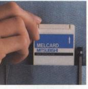
(SRAM, OTPROM, masked ROM), upgrade and downgrade memory density, and change data width (8 bits, 16 bits). All with an extremely rugged device that's the size of a credit card (86mm x 54mm x 3.4mm).
