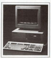
They incorporate a Basic language coprocessor, a plug-in card that includes—in addition to an IEEE-488 interface—a 68000 coprocessor with 512k bytes of RAM separate from the Vectras' system RAM, and ROMs containing the HP Basic 5.0 language.
