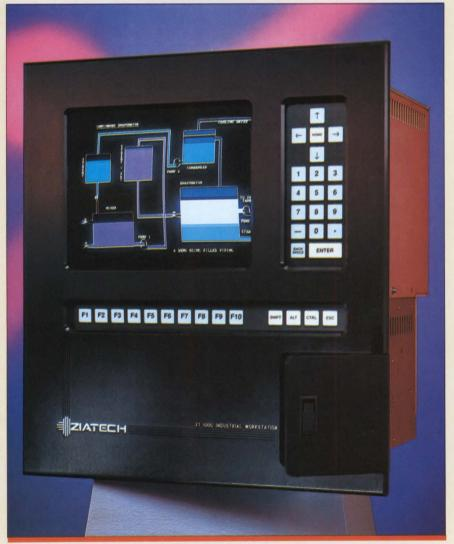
The ZT 1000 Industrial Workstation can be mounted in a panel cutout or on a 19" RETMA rack. The new controller meets NEMA 4/12 standards, and features the STD DOS operating system. See story on page 2.
