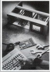
quire disk or communications capabilities, you can replace the SPEGA, SPDC, and SPCOM cards with an SPCGA graphics card. This card provides CGA-, MDA-, and Hercules-compatible graphics and includes four byte-wide memory sockets for as much as 128k bytes of RAM or 256k bytes of EPROM. SCPC88, £345; SPEGA, £385; SPDC, £185; SPCOM, £159; SPCGA, £195.
