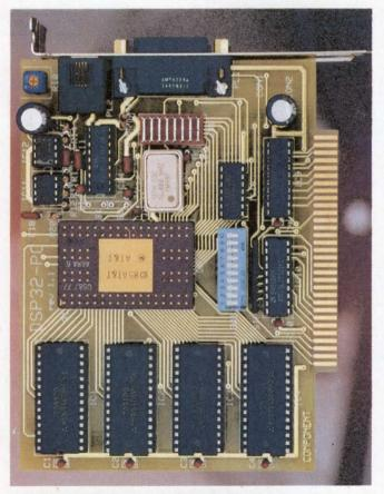
A 16-MHz accelerator board for developing DSP algorithms on an IBM PC (Communication Automation & Control)
