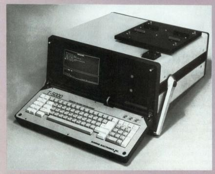
**Portable in-circuit programmer with sockets for programming off-board devices** (Sunrise Electronics Inc)
