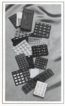
serves as the switch actuator and is positioned over a 3-layer membrane panel. The membrane uses conductive silver ink traces. In the conductive keypads, a carbon-impregnated silicone pill is molded on the underside of the rubber dome to accomplish the switching function. The conductive switch mounts onto a glass epoxy pc board.
