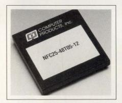
levels. Internal short-circuit protection guards against damage from load shorts, and overvoltage protection prevents damage from converter failure. The units operate at full power over a -25 to +70°C range. \$77 (50).
