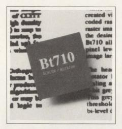
sion, gamma correction, or mapping from 4-bit gray to 8-bit pixels. A software tool kit provides CCITT compression and decompression, image scaling, rotation, mirroring, and Boolean bitblt operations to destination buffers. Bt710 version in 132-pin pin-grid array, \$132 (100); Bt710EVK IBM PC version under DOS and Windows 3.0,
