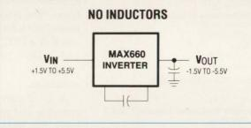
The MAX660 uses only 2 external components and is available in space-saving 8-pin DIP and SO\* packages.
