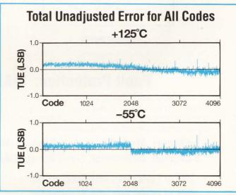
With **NO** gain, offset, or linearity adjustments, the total error for a MAX178 stays below  $\pm 1$  LSB from  $-55^{\circ}$ C to  $+125^{\circ}$ C for all codes.
