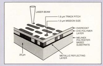
Fig A—Digital paper, or digital optical tape (DOT), has four layers. The heat of the write laser creates pits in the active dyepolymer layer.
