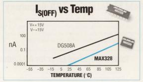
The MAX328/329 have  ${<}1\mathrm{pA}$  leakage at  $25^\circ\mathrm{C}$  — 1000X lower than the DG508/509.
