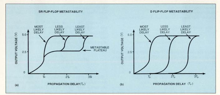
Fig 4—The metastable plateau in the output of an SR flip-flop causes an increase in the device's propagation delay (a). Although a plateau is not evident in the output of a D flip-flop (b), metastability still increases the propagation delay.
