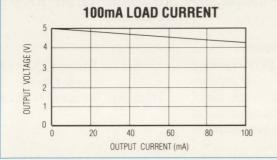
Maxim's new MAX660 voltage inverter powers 100mA loads.
