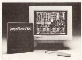
Simultaneously working on all layers, the Tango-Route Pro package for IBM-compatible PCs automatically generates pc-board designs optimized for manufacturing with 45° trace angles and minimized trace lengths.
