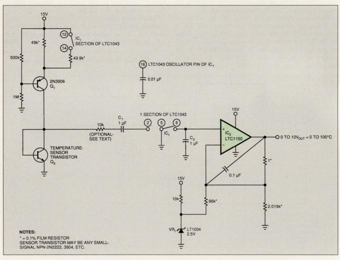
Fig 1—The transistor  $Q_2$  senses temperature. This circuit requires no compensation, even if you change transistors.
