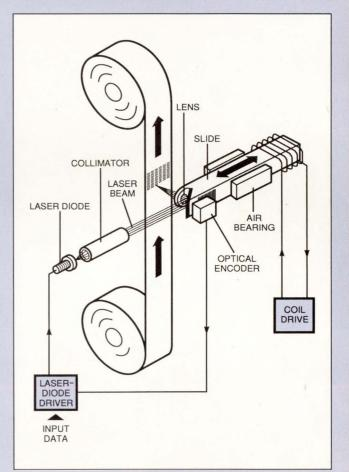
Fig D—Creo's optical tape drive writes 32 bits across the tape in one direction, then steps the tape and writes 32 bits across the tape in the other direction.
