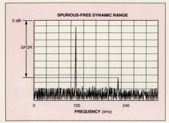
Fig 4—The spurious-free dynamic range of an A/D converter is the range, in the amplitude spectrum, in which frequency components other than the fundamental do not exist.
