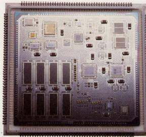
The motherboard of a microcomputer, on a multichip module made with BCB from Dow—actual size.
