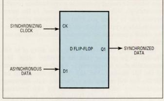
Fig 5—One of the simplest single-stage data synchronizers is the D flip-flop.
