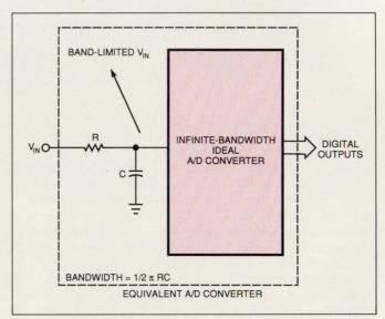
Fig 6—This equivalent circuit illustrates the effects of a bandlimited A/D converter compared with an ideal infinite-bandwidth converter.
