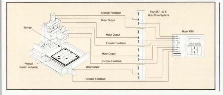
peatability at 0.0001 inches. This, coupled with extremely smooth motion of the Daedal tables, prevent liquid flashing. The transverse cross roller table carrying the X-Y-Z positioning system provides excellent rigidity and stiffness to the syringe needle motion.
