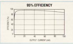
High efficiency makes the MAX660 ideal for portable applications.
