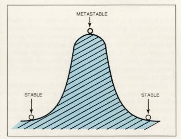
Fig 3—The metastable state is analogous to a ball balanced on top of a smooth hill. Any slight disturbance will start the ball rolling toward either of the stable states at the bottom of the hill.
