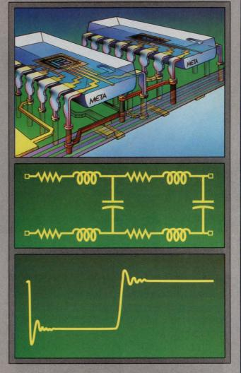
Transmission line analysis with HSPICE: Measure physical sizes of conductors (top). Simulate using output buffer and transmission line models (middle). View results (bottom).
