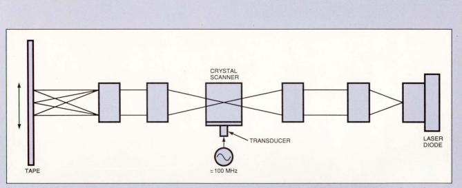
Fig C—A DOT tape scanner has no moving parts; the angle at which the beam emerges from the crystal depends on the radio frequency applied to the crystal via a transducer.
