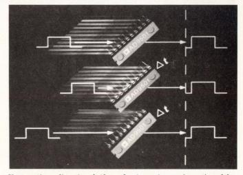
You can time-align signals throughout a system, using a time-delay generator such as Analog Devices' TTL-compatible AD9501.
