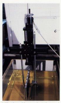
In Ultran's emulsion scanning tank, a sample is tested with the sweeping motion of a transducer attached to a Daedal table-configured bridge.
