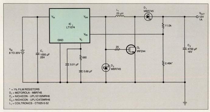
Fig 1—This switching regulator is suitable for battery-powered applications because it produces a 12V dc output from inputs ranging from 8 to 20V dc.
