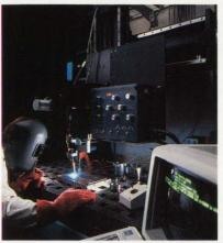
X-Y-Z -Axis translation system provides complex traversing of an arc welding torch head. Daedal Division is the most recent addition to the growing Parker Hannifin motion control group. Daedal specializes in the manufacture of custom positioning systems as well as standard components including ball slides, stages, and motorized linear and rotary tables.
