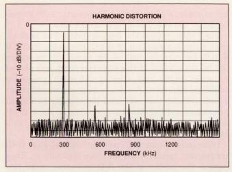
Fig 2—This harmonic-distortion plot shows the fundamental frequency at 300 kHz with harmonics present at 600, 900, and 1200 kHz.
