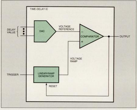
**Fig 1—Time-delay circuits typically contain a voltage ramp** initiated by a trigger input. When the voltage ramp reaches the level of the adjustable reference voltage, the comparator changes state, outputting the delayed edge. An internal DAC or analog input provides the reference voltage.
