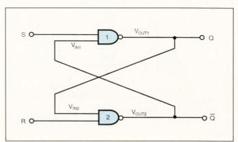
Fig 1—The cross-coupled NAND gates of an SR flip-flop can reach a metastable condition because the output of one gate is an input to the other.
