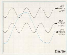
To demonstrate the ruggedness of MAX378, Input 2 is overdriven with a 150Vp-p AC signal. This Input survives, and the adjacent On Input (CH1) is unaffected during this abuse.
