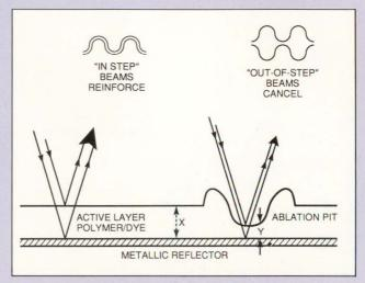
Fig B—Interference effects allow the system to detect pits or the absence of pits as the read laser passes over the material.
