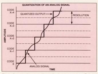
Fig 1—Quantization maps the analog input range into  $2^N$  digital words. This process results in a quantization error of  $\pm 0.5$  LSB max.
