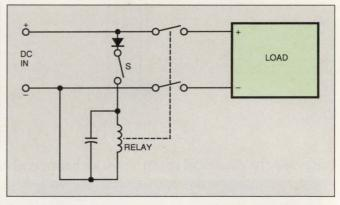
Fig 1—This simple relay circuit provides absolute reverse-polarity protection because it will not apply power to the load unless the power's polarity is correct.
