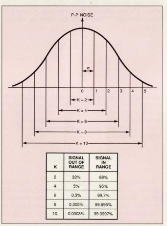
**Fig 5—The peak-to-peak noise of an ADC** is a function of its loading factor (K) and statistical deviation ( $\sigma$ ). If K is 2, 68% of the signal will fall within the full-scale range of the converter.
