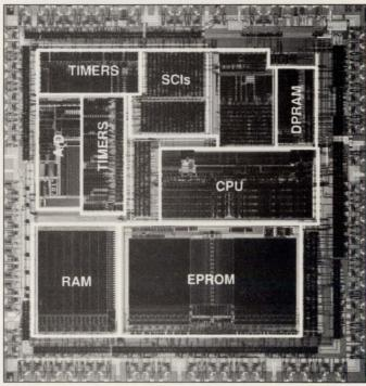
The H8/330's assorted peripheral functions complement a flexible 8/16-bit internal architecture that uses register-to-register operations.
