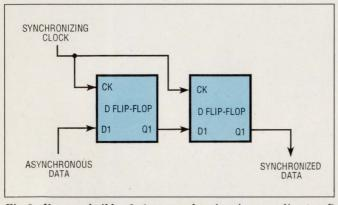
**Fig 6—You can build a 2-stage synchronizer** by cascading two D flip-flops that have a common clock. Continue adding D flip-flops to build a multistage synchronizer.
