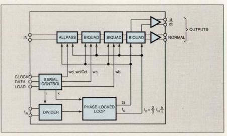
A phase-locked loop ensures the stability of this programmable sixth-order Bessel filter IC. The lowpass filter offers a cutoff frequency ranging from 1.5 to 15 MHz.
