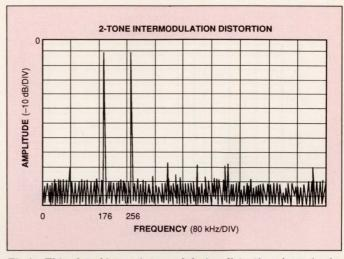
**Fig 3—This plot of 2-tone intermodulation distortion** shows fundamental frequencies at 176 kHz ( $F_1$ ) and 256 kHz ( $F_2$ ). Note the presence of distortion products at 80 kHz ( $F_2-F_1$ ) and 432 kHz ( $F_2+F_1$ ).
