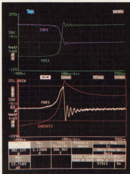
Current and power. Make accurate, high-bandwidth power measurements and energy calculations with our new 11A16 Programmable Current Amplifier. Current and voltage maintain their proper phase relationship to 50 MHz.
