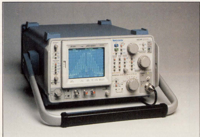
Low residual FM enables narrow resolution bandwidths. The Tektronix 497P portable spectrum analyzer has less than 5-Hz p-p residual FM, thereby permitting a 10-Hz bandwidth filter.
