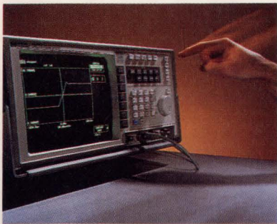
Frequency and time-interval analyzers make and store long series of measurements with little or no dead time between readings. The units help spot problems you can't find with conventional counters by letting you visualize the measurements (pg 79).
