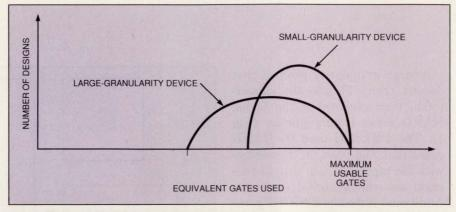
Fig 5—If you were to try many different designs on two PLDs with an equivalent number of maximum usable gates, one with large logic-cell granularity and another on a device with small granularity, you'd probably come up with something similar to the two hypothetical curves shown. Although the shape of the distribution is unknown, the smallergranularity logic cells should show less variation in equivalent gates due to their greater flexibility. See text for further explanation.
