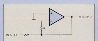
Fig C—Most current-feedback op amps won't tolerate a capacitor placed directly from output to input. This modified configuration is one suggested integrator from Ref 3.
