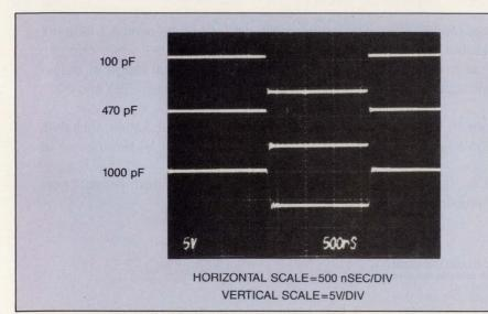
Fig 3—Stable operation while driving a capacitive load is a characteristic more and more high-speed amplifiers, such as the MAX404, share. However, as the capacitance increases, the amplifier must slow down to remain stable. Note the slowest response on the bottom trace. (Photo courtesy Maxim Integrated Products)
