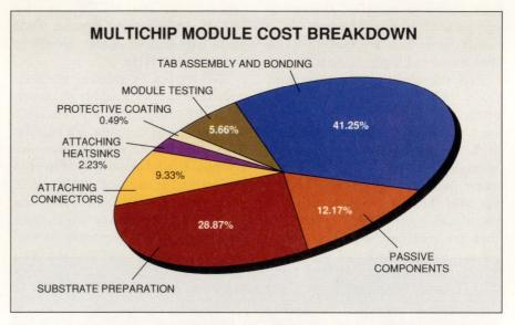
The cost of TAB assembly and bonding and the cost of substrate preparation constitute the two major factors affecting the price of MCMs, according to this analysis by MCC. The QTAI project and the TAB technology development project are working toward lowering these costs.
