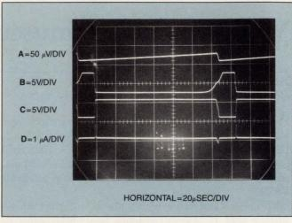
Fig 2—This scope photo captures one cycle of the VFC's action. The ramp in trace A causes  $IC_1$ 's output to eventually switch (trace B), thus developing a corresponding output pulse (trace C). Trace D is a reset pulse for the ramp.
