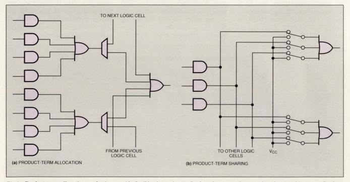
Fig 2—Product-term allocation or sharing provide flexible alternatives to fixed product terms in sum-of products architectures. Product-term allocation (a) typically lets you switch product terms in groups of four so that logic cells needing more product terms can take them from logic cells that need fewer. Product-term sharing (b) lets you use fewer product terms in a device by using a product term in more than one sum.
