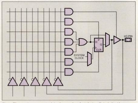
Fig 1—The generic components of simple sum-of-products logic cells include wide programmable-AND gates feeding into an OR gate. Additional product terms may be used to control preset, reset, output enable, clocks, and other functions in the logic cell. All product terms are fixed in this example.
