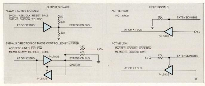
Fig 2—The four different types of PC bus signals each need a specific driver for the extension bus.
