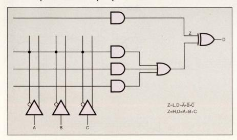
Fig 3—Using an XOR gate after the sum-of-products lets the Altera Max family change between active-high and active-low logic. Among other things, being able to invert the active state lets you use de Morgan's theorem to create wide sum terms from wide product terms. Some manufacturers provide an inversion select at the output of the logic cell, which provides a similar capability.
