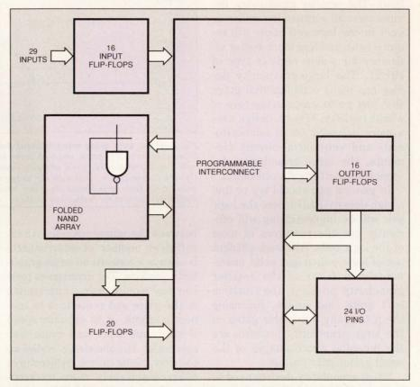
**Fig 4—A folded NAND array** is the basic building block of the PML2552. Ninety-six NAND gates with 258 inputs make up the basic logic element. Additional wide NAND gates drive the flip-flop inputs. The device provides flexible product sharing.
