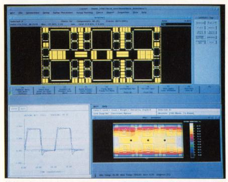
**Multiple design windows provide a concurrent framework** within Mentor Graphics' MCM Station. The top window shows placement of the die upon an MCM substrate; the bottom right window displays a thermal map of the module, and a high-speed analysis occupies the bottom left window.
