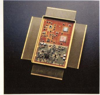
**Providing telecommunications and networking functions** at 622 MHz, this custom multichip module was designed using Valid Logic's Allegro MCM Design System.
