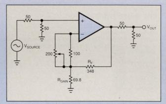
**Fig B—This circuit lets you decouple** the feedback resistor from the gain-setting resistor so you can tailor the op amp's frequency response. (Figure courtesy Comlinear Corp)
