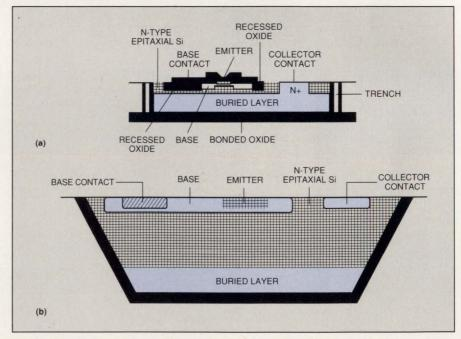
Fig 1—You can't choose op amps on the basis of process technology alone—you need some appreciation of how the devices achieve their specifications. A high-speed process developed by Harris Semiconductor lets the company build fast op amps using a smaller die (a) than the company's older process (b). The resulting 850-MHz op amps cost \$9.95.
