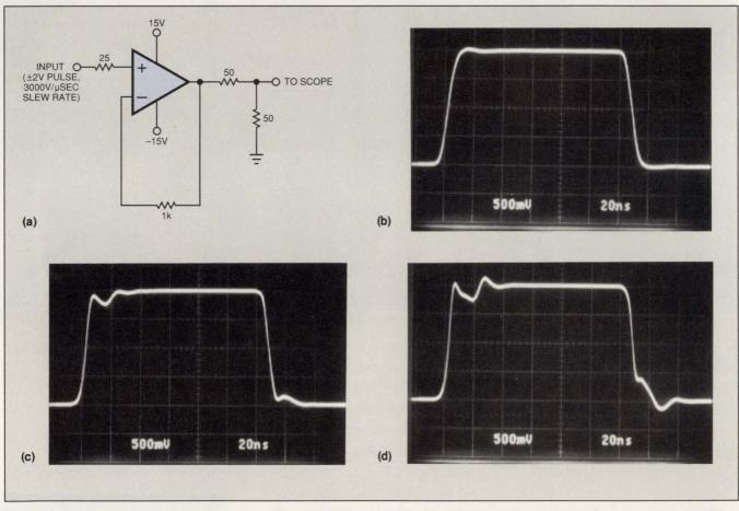
Fig 2—No two current-feedback amplifiers are alike, although they are all architecturally similar. For example, three of these amplifiers operating under the same slew-limited conditions exhibit three very different responses to a  $4V_{P-P}$  high-speed pulse (a). The amplifier in **b** is well behaved, but those in **c** and **d** reveal distortion that is most likely the result of input slew-rate limitations. (Photos courtesy Elantec Inc)
