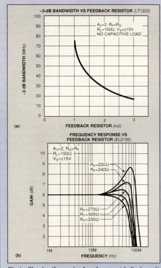
Fig A—Choosing the exact value of a current-feedback amplifier's feedback resistor  $(R_F)$  is crucial. As these graphs from the LT1223 (a) and EL2120 (b) data sheets show, this resistor's value directly affects the peaking and frequency response of the amplifier.  $(A_V$  is voltage gain.)
