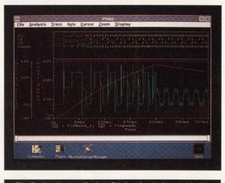
The Design Center displays PSpice simulation results for both analog and digital waveforms together on the same plot.
