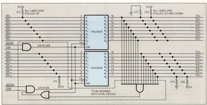
Fig 1—With this simple extension-bus circuit and the drivers in Fig 2, you can add extra cards to your PC and provide isolation for experimentation. Note the 16-input AND gate, which handles extension-card data writes.
