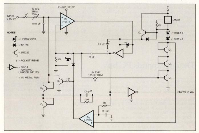
Fig 1—This voltage-to-frequency converter (VFC) consumes one-thirtieth the current of other VFCs.
