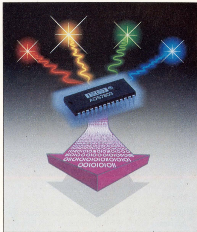
This 12-bit self-calibrating ADC, the ADS7803, is available from Burr-Brown. The low-power device can sample to 100 kHz and features a 4-channel multiplexer.
