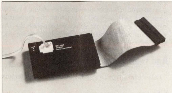
This evaluation board is a complete system. The Dallas DS5000KT has an 8051 \mu C, 32 kbytes of SRAM, and a backup battery. Systronix Basic or Franklin C can be used for higher-level languages.
