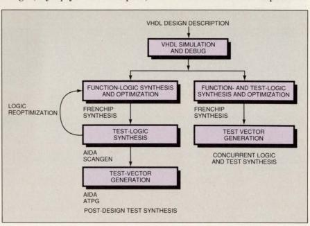
Post-design test insertion requires evaluating the impact of the added test on your design. Teradyne recommends specifying the test structures from the start.
