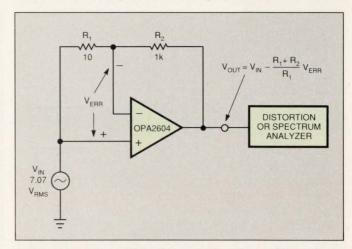
Fig 1—Selectively amplifying  $V_{\text{ERR}}$  magnifies the amplifier's distortion signal for direct measurement at the output of the amplifier tested.
