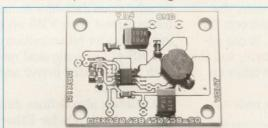
The MAX730 application circuit components fit into  $V_2$  in<sup>2</sup> (3.2cm<sup>2</sup>) of board space.
