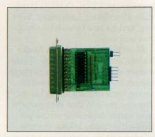
You can debug 68HC16 target code without an ICE. To monitor and control execution, the ICD16 links to the target  $\mu$ C via background mode.
