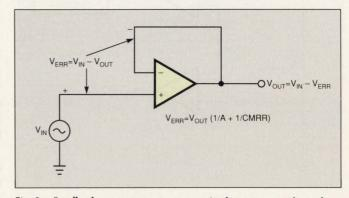
Fig 1—Feedback separates an op amp's distortion products from the test signal by developing a signal  $V_{\text{ERR}}$  equal to the difference between input and output signals.
