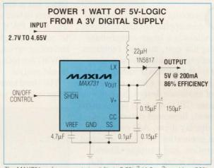
The MAX731 surface-mount circuit fits in 0.65ir<sup>2</sup> (4.2cm<sup>2</sup>) and has 86%
