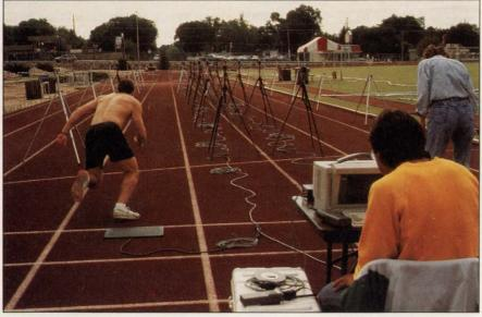
A sprinter gets set to run through a series of electronic timing lights, which measure his rate of acceleration.
