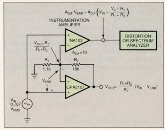
Fig 4—The amplifier's distortion products, included in  $V_{\text{ERR}}$ , remain separated from the test signal in measurements of the generalized noninverting circuit.
