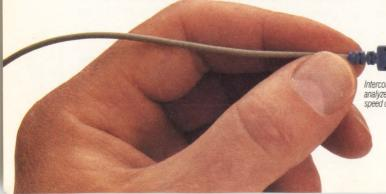
Interconnect assembly for Hewlett-Packard logic analyzer uses 105 ohm high-performance, high speed coax.
