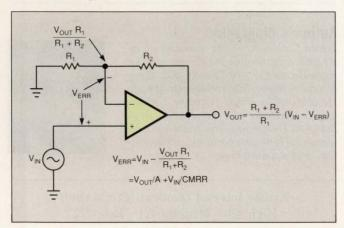
Fig 3—In the generalized feedback case, the output signal, along with its distortion, reflects to  $V_{\text{ERR}}$  through an attenuation.
