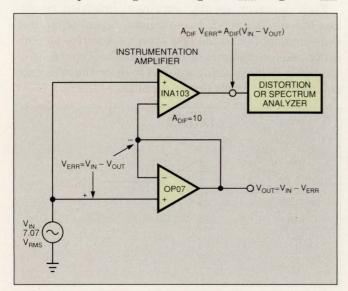
Fig 2—Directly implementing Fig 1's signal separation requires adding an instrumentation amplifier to provide a ground-referenced signal.
