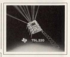
range of 118 dB, typically produces a 100-kHz signal in office desk lighting and 1 Hz in darkness. An external capacitor can adjust the output frequency for a given light level to match the sensor to the input frequency range of a μP. \$4.61 (1000). **Texas Instruments Inc**, Semiconductor Group (SC-91086), Box 809066, Dallas, TX 75380. Phone (800) 336-5236, ext 700; outside US and Canada, (214) 995-6611, ext 700.
