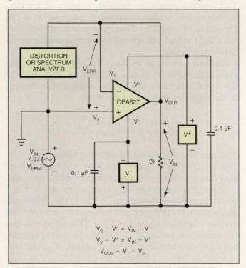
Fig 6—Power-supply bootstrapping permits directly measuring  $V_{\rm ERR}$  and does not change an amplifier's internal voltage swings.
