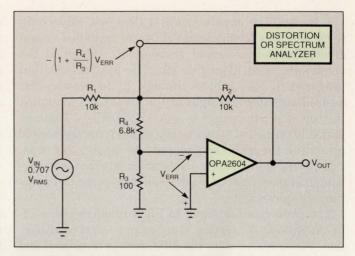
Fig 4—Adding R<sub>4</sub> combines selective amplification with signal separation for the inverting amplifier.
