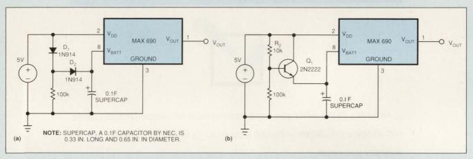
Fig 1—Teamed with a switch-over IC, large capacitors can serve as battery backup in certain applications. The  $100-k\Omega$  resistor in (a) ensures that  $D_1$  is forward biased so that normal variations in  $V_{DD}$  don't mistakenly trip the IC. The presence of  $Q_1$  and its associated resistors in (b) shorten the delay between power on and backup capability.
