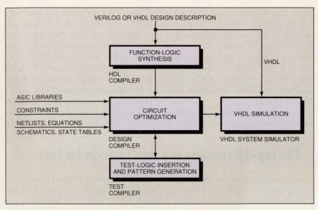
Beginning with either Verilog HDL or VHDL, Synopsys' test strategy is to first synthesize and optimize your function logic, then insert the test logic and generate patterns.
