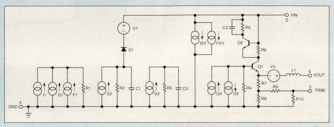
Fig 1—Simple dc components, such as voltage references, need accurate models. This REF-01 model includes the temperature coefficient for R1, so that the output voltage varies linearly with temperature. The model does not include second-order, nonlinear drift effects.
