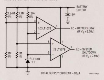
Figure 1. Low Battery Detector with System Shutdown
