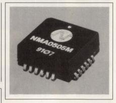
of  $\pm 5$ ,  $\pm 9$ ,  $\pm 12$ , or  $\pm 15$ V. Each output provides 1W of output power. The converters feature 1000V dc isolation, 80% efficiency, and operate over a -50 to  $+85^{\circ}$ C range with no derating. \$19.50. International Power Sources Inc, 200 Butterfield Dr, Ashland, MA 01721. Phone (508) 881-7434. FAX (508) 879-8669. Circle No. 396
