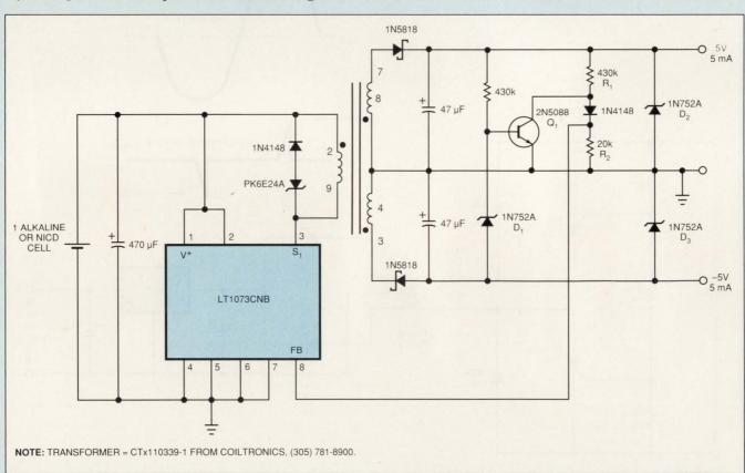
Fig 1—To produce a split supply from a single cell, this circuit uses a micropower dc/dc converter to supply ±5V and any 10-mA current combination.
