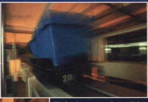
Wafer-bearing robots glide noiselessly overhead on a state-of-the-art ceiling railway.
