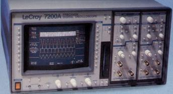
The new 7200A Series, our high performance line with high resolution color display, features 500 MHz bandwidth at 2 GS/s with 200k memory standard and 1 Meg/channel optional. Modular architecture allows the user to choose 2, 4 or even 8 channels, all with super-long memory. Floppy and hard disk drives are standard features.
