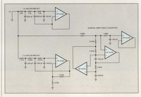
(Author's reply: The first difference Michael Wyatt points out is in the cutoff frequency that Fig 5 [in the article] had for the Sallen and Key filter. He says that simulations of this circuit show it has a cutoff frequency of about 29 kHz, not 40 kHz as specified. Upon examining my data and doing my own Spice simulations, I find that Wyatt is correct. The reason for this and the associated peaking that the filter exhibits is that the 1.731- and 6.227-k $\Omega$  re-
