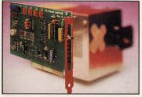
Designed as a diagnostic aid for PC/XT/EISA systems, the Wintek PC Bus Power Monitor Card (\$195) provides a quick way of checking the power supply in a personal computer. LEDs provide a realtime indication of power quality, as well as remembering momentary out-of-tolerance operation. A deluxe model (\$249) has an audible alarm, a system clock monitor, and a refresh signal monitor.
