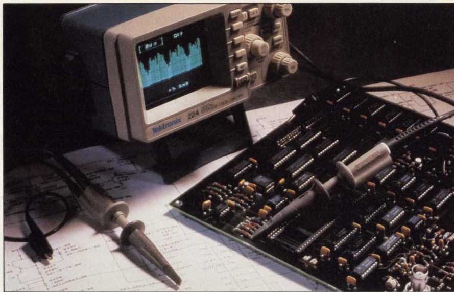
Although it resembles a pint-size version of a conventional scope, the Tektronix 224 is not conventional. It offers 60-MHz bandwidth, and its two inputs are ohmically isolated—not just from the chassis but from each other.
