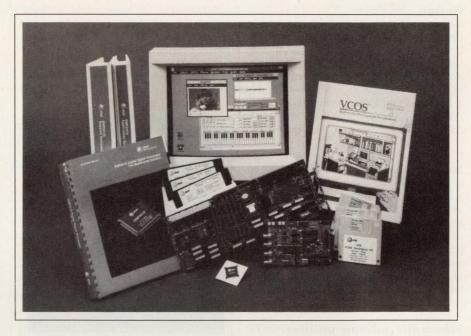
By caching critical code segments in the DSP's internal RAM, VCOS allows the DSP to run programs and access data directly out of host memory. The complete package includes a variety of software development tools and libraries. For PCs, the software requires an Ariel development board; for the Macintosh, it requires a board from Spectral Innovations. \$3000.
