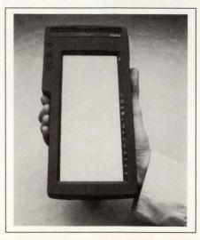
two drives can accommodate two memory cards having as much as 4 Mbytes each. A 7<sup>1</sup>/<sub>4</sub>-in. diagonal display has 25 lines of 80 characters each. \$1995.
