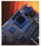
The 33MHz 040 processor is only one of the Motorola contributions that turned NeXT's vision into reality. Among the essentials NeXT wanted for the NeXTstation Turbo was super-fast memory transfer, so they chose Motorola's CMOS
