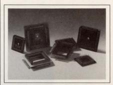
Surface-mount adapters. These surface-mount PLCC (plastic-leaded-chip-carrier) adapters interconnect a daughter card via a PLCC socket on a mother board. The phosphor bronze contacts feature 30 µin. of gold plating. The housing material accommodates all solder-
