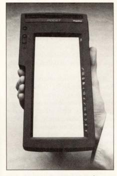
Poqet Computer Corp's Poqet Pad, a socalled palmtop computer, weighs 1.2 lbs. It sacrifices screen area for increased battery life.
