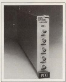
PCXI bus audio-analysis module. The PX2362 analyzer plugs into the PCXI (PC extended for industry) bus. The 2-channel unit, which has a bandwidth of 1 to 50 kHz, includes a 20-MHz μP with 256k words of dynamic RAM and 32 kbytes of zero-wait-state RAM. It averages signals and computes floating-point FFTs from 64 to 2048 points. \$3495. Rapid Systems Inc, 433 N 34th St, Seattle, WA 98103. Phone (206) 547-8311.
