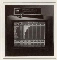
Background-mode emulator. The Performance Plus Model of the EST Series 300 is a background-mode emulator for the Motorola 68332, 68331, 68340, and 68300. It provides software performance analysis through Motorola's background-mode debugging port. The emulator costs less than an in-circuit emulator and is less intrusive than a ROM monitor. \$3050. Embedded Support Tools Corp, 10 Elmwood St, Canton, MA 02021. Phone (617) 828-5588. FAX (617) 828-7941. Circle No. 409
