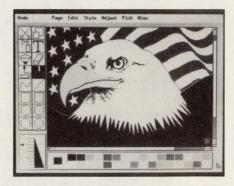
The TLX-1832S-C3M black-and-white display from Toshiba features a VGA resolution of  $640\times480$  pixels, a brightness of 50 cd/m², and a contrast ratio of 12:1. Using flexible TAB (tape-automated-bonding) driver chips, which fold behind the display area, reduces the panel's overall dimensions to little more than the size of the LCD glass.
