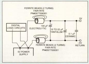
Fig 1—This simple filter will cut the noise on digital-logic power lines down to less than a couple of millivolts, allowing you to power sensitive analog circuitry.
