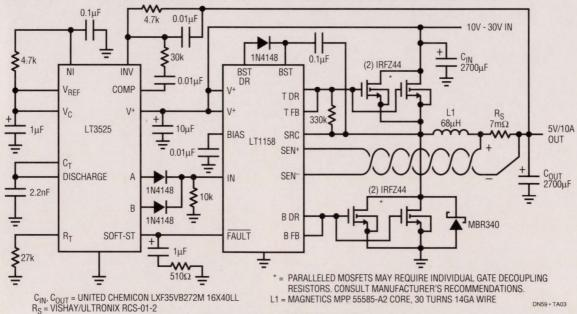
Figure 3. High Efficiency 50W DC-to-DC Converter
