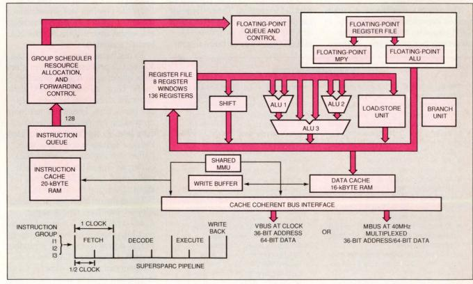
SuperSPARC is the first superscalar SPARC  $\mu$ P. It issues as many as three instructions per clock cycle, moving them through the 8-stage pipeline as an execution group.
