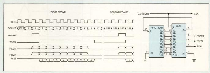
Fig 1—The PAL decodes the output of the ripple counter to produce a burst of eight bytes, during the proper time-multiplexed "frame," that a codec-filter combo IC can convert into a reference 1-kHz, 0-dBm analog output. Refer to Listing 1 for the definition of some of the signals in the timing diagram.
