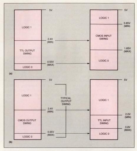
Fig 1—When both ICs are operating at 5V, TTL/CMOS logic compatibility is not a major problem. A TTL output can drive a CMOS input (a), and a CMOS output can drive a TTL input (b).
