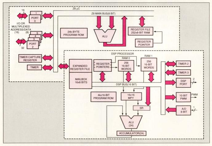
The Z89120 integrates a Z8  $\mu$ C with a 16-bit DSP processor. The processors are independent, each with its own peripherals; they communicate via a register mailbox and internal interrupts.
