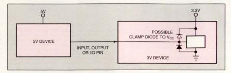
Fig 2—Problems can arise when a 5V device drives a 3.3V device. If the 3.3V circuit has a clamp diode to  $V_{cc}$  (the usual case), the likelihood exists that the output of the 5V device will forward bias that diode and damage the 3.3V device.
