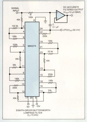
Fig 1—Adding an RC network to a lowpass filter removes offsets, restoring perfect dc accuracy.
