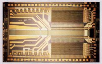
Surface acoustic waves carry electron-packet samples down the center of this GaAs ACT (acoustic-charge-transport) device where evenly spaced electrodes sense the packets and convert the charge into voltages. A summing amplifier combines the electrode voltages, thus creating a sampling (but not digitized) convolution filter that operates at 360 MHz with 8-bit equivalent accuracy.
