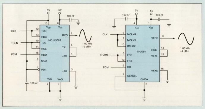
Fig 2—The test circuit in Fig 1 can excite two types of codec-filter combo ICs.
