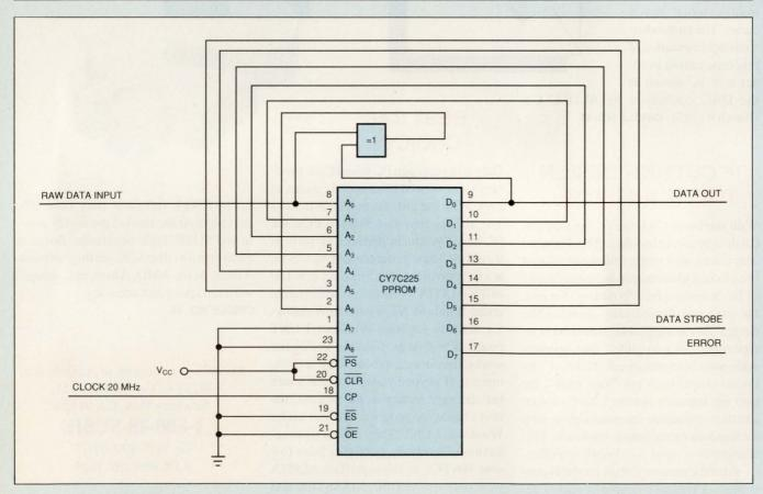
Fig. 1—A registered PROM can function as a high-speed finite state machine. Here, the PROM is a phase-locked loop (PLL), operating at 20 MHz, that can decode a 4-MHz Manchester-II data stream.
