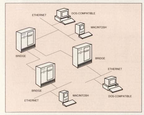
Bridges can extend the maximum LAN distance by acting as repeaters, or segment large LANs into smaller LANs to relieve traffic congestion. The tree topology guarantees that there aren't any loops in the network.
