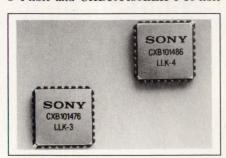
SRAMs are synchronous, self-timed versions organized as 1024 words×4 bits and 4096 words×4 bits, respectively. The devices feature access times of 3 and 4 nsec and cycle times of 4 and 5 nsec, respectively. These synchronous SRAMs include input and output latches and on-chip write timing. The CXB101474D-3 and CXB101484D-4 are asynchronous versions without the latches and write-timing features. Synchronous versions come in 28-pin LCCs; asynchronous versions come in 24- or
