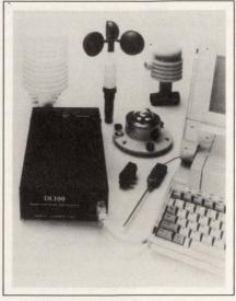
can set in 10 steps from 30 mV to 30V. After you set up the logger, an operation that requires a PC-notebook PC works fine—you can remove the PC and leave the logger unattended for as long as 300 hours in a location where ac power is inaccessible. The logger, which supplies transducer excitation, uses an integrating ADC to minimize noise and
