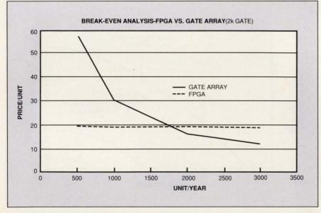
Fig 3—This simple break-even analysis begins with the following assumptions: the FPGA total engineering cost is \$5300; the mask-programmed gate-array NRE cost is \$27,300; an FPGA costs \$0.013/gate; a mask-programmed gate array costs \$0.0007/gate; and the package for both types of devices is a 68-pin plastic leaded chip carrier. By this analysis, mask-programmed gate arrays become economical at approximately 2000 devices/year.
