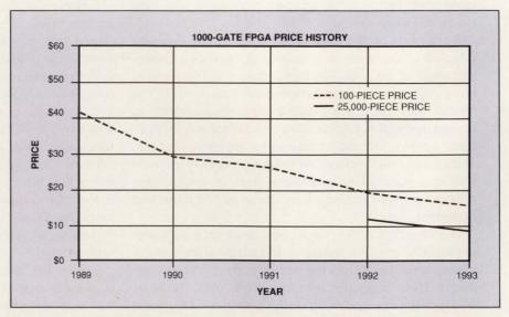
Fig 1—The price history of an older 1000-gate FPGA, which currently sells for 3 to 4 times the price of an equivalent mask-programmed gate array, indicates that the currently very high prices for newer FPGAs will probably drop drastically too.
