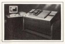
The systems include software for incircuit testing of boards that include IEEE-1149.1 boundary-scan features. The systems test circuits that have as many as 1296 nodes. From \$100,000. **Hewlett-Packard Co**, 19310 Pruneridge Ave, Cupertino, CA 95014. Phone (800) 452-4844. **Circle No. 398**
