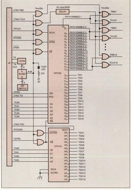
Fig 1—By adding a handful of ICs to your next pc-board design you can partition a single unwieldy JTAG scan path into 16 manageable boundary-scan paths.
