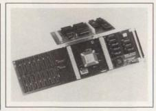
contains a 40-MHz TI TMS320C30 DSP chip and as much as 8 Mbytes of static RAM. Dual 96-pin DIN connectors accept a range of daughter boards ranging from prototype to A/D boards. The company can also build custom boards on a quick turnaround basis. The development system runs all of TI's development software. From \$995. Wintriss Engineering Corp, 4715 Viewridge #200, San Diego, CA 92123. Phone (800) 733-8089. Circle No. 440
