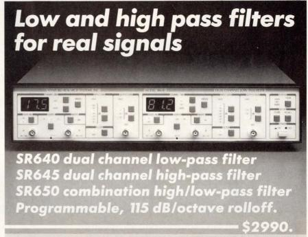
The SR640, SR645 and SR650 offer unique combinations of filter specifications, preamplifier performance, and programmability at a price far less than other instruments. Featuring two fully independent 8-pole, 6-zero elliptic filters with less than 0.1 dB p-p passband ripple and 115 dB/octave rolloff, these filters are ideal for general purpose signal processing as well as anti-aliasing for digital signal processing systems.
