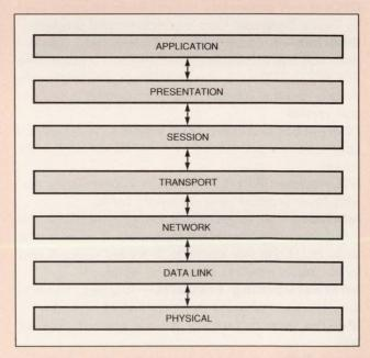
Fig A—The OSI model consists of seven hierarchical layers that vendors use to exchange data between computers on a network.
