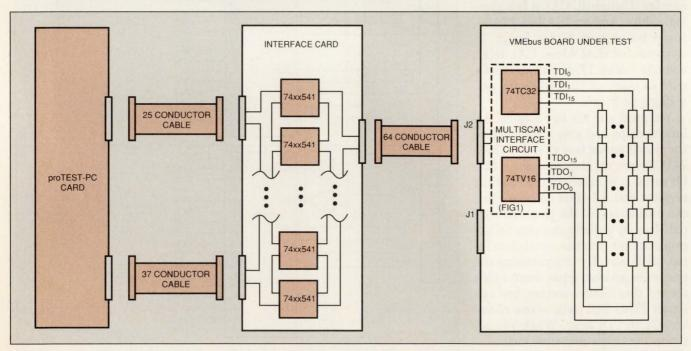
Fig 2—You perform boundary-scan tests using a DOS-based computer. An ISA bus JTAG tester board, the proTEST-PC from Alpine Image Systems has a 4-wire JTAG bus and a 24-bit parallel output port. The tester's output ports connect to the board under test via an interface card populated with 74xx541 Octal 3-State buffers.
