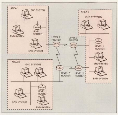
Routers operate at the network layer to transmit data between LAN clusters. The internetworking products use a variety of proprietary and open protocols to route the data.
