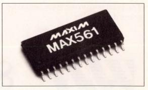
This RS-232C transceiver from Maxim Integrated Products implements the new EIA/TIA-562 standard, which guarantees operation with output voltages as low as ± 3.7V. The device can operate at voltages as low as 3.0V at a data rate of 20 kbps.
