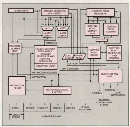
A superscalar RISC processor, the hyperSPARC issues as many as two instructions per cycle. Rather than relying on limited on-chip caches, the processor uses large, fast off-chip caches integrated with a cache controller on an MBus module.
