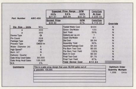
Fig 4—Showing the multitude of factors you must consider, this ASIC-cost spreadsheet from Valence Associates derives unit costs, GPMs (gross profit margins), and optimal ordering quantities for all vendors' currently available mask-programmed gate arrays.
