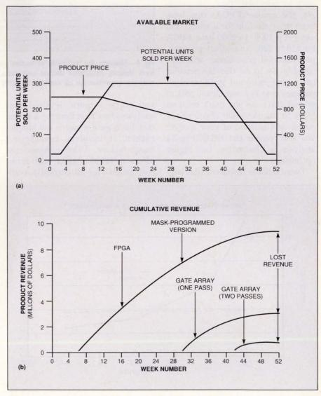
Fig 2—Your marketing department may be willing to trade the higher cost of an FPGA for an earlier product launch. This example from Altera depends on several variables: the shape of the product-sales curve and price curve in (a) and the development leadtimes in (b). Obviously, your analysis could vary significantly. Notice that the price curve also assumes a shift to a mask-programmed part.
