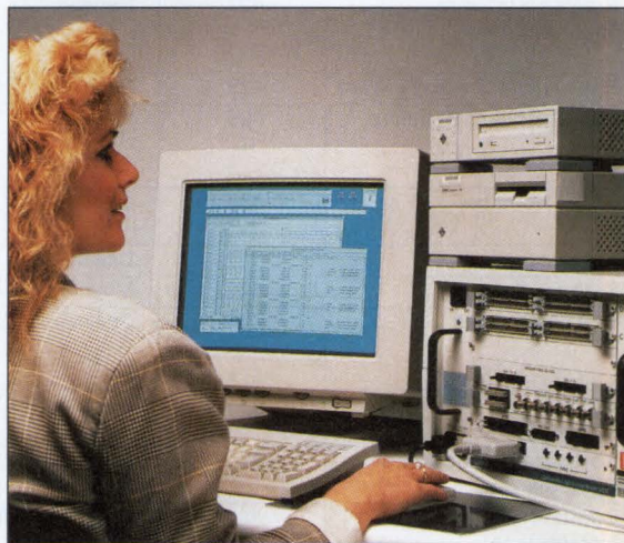
The configuration flexibility of high-end logic-analysis systems such as Biomation's CLAS 4000 lets you bring multiple cross-triggered analyzers to bear on thorny hardware problems in multiprocessor systems. Because one unit can contain several analyzers, the setup is more compact and less intimidating than you might expect.
