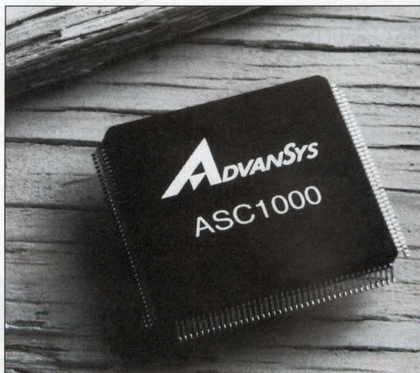
By processing 255 data-access requests simultaneously, the ASC1000 achieves 94% SCSI-2-bandwidth utilization.
