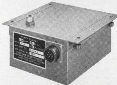
Conduction cooled, high voltage regulated power supply. Output: 10 KV. Regulation: 1%. Weight: 7.5 lbs. Meets MIL-E-16400.
