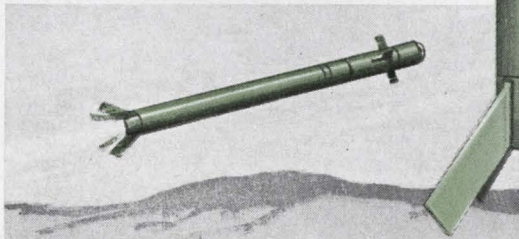
Infrared sensor locks on target. Miniature computer directs steering fins to guide Redeye.
