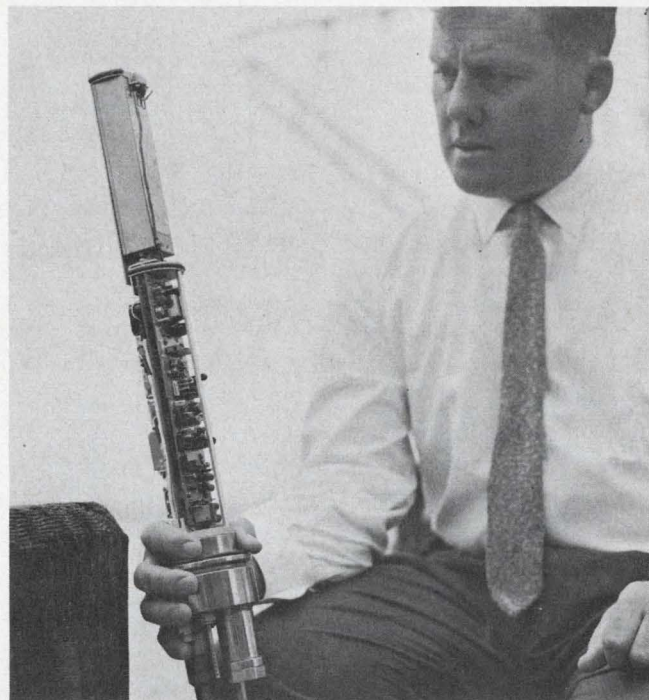
Latest Bissett-Berman in situ salinometer is held by its developer, Neil Brown. The unit incorporates a parameter-sensitive telemeter circuit. Instrument measures salinity of sea water by sensing its conductivity and automatically applying pressure and temperature compensation. Computed values are represented as frequency analogs.
