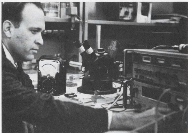
"When applying signals to a transistor under test, always start from zero," says the author, Ronny Mann, shown adjusting bias for the I_{CEX} measurement.
