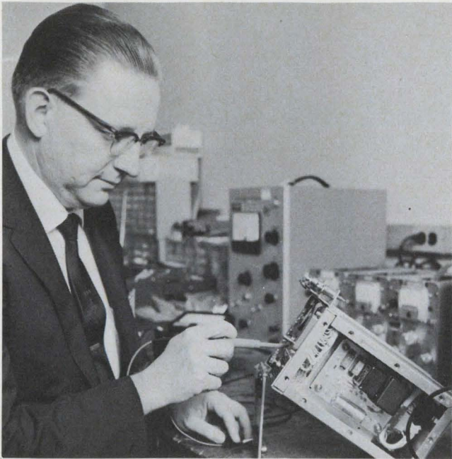
The afc circuit being tested by F. H. Wolf can cut drift in your pulse radar. p. 80.
