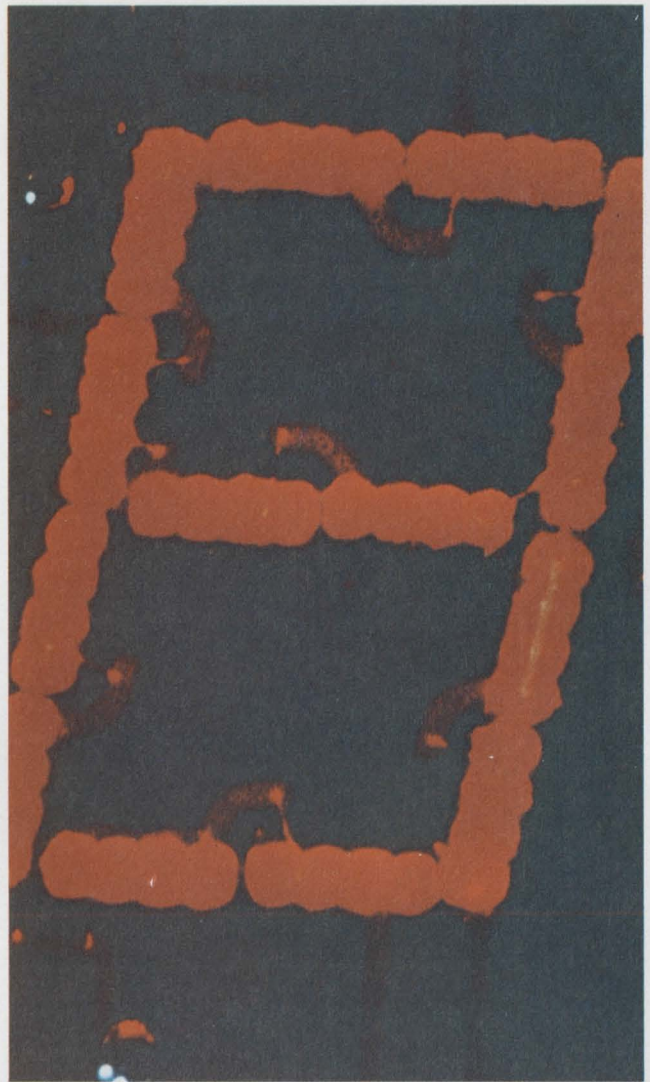
Monsanto's Man 2 is a seven-segment gallium-arsenide-phosphide numeric indicator, second-generation from new facility in Cupertino, Calif.
