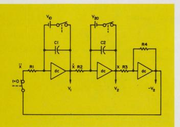
32. The harmonic oscillator used in the Type V converter solves differential equations of the form X = KX (K=constant terms).
