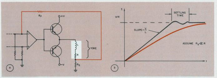
1. Sensing resistor  $R_{\rm s}$  feeds back a signal voltage proportional to the yoke current (a). The feedback scheme
