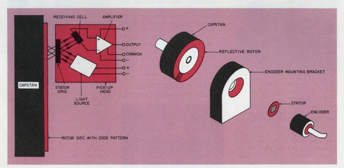
Reflective-surface rotary encoder permits digital speed control without increasing mass or sacrificing acceleration time. Code pattern on reflective plastic disc is
