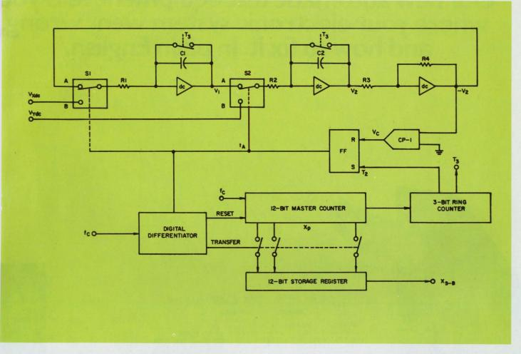
34. The Type V converter is controlled by a 12-bit master counter. Integration time constant dependence
