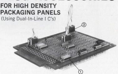
Provide greater flexibility in prototyping and packaging. Facilitate interposing of discrete components. Plugs have 14 and 16 leads with pins on .100" centers and .300" between rows.
