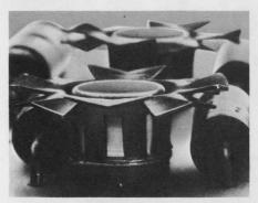
T05's and T018's in high density packages can be cooled off with efficient push-on Fan Tops that cost only pennies. T-shaped, need no board room, let other components snuggle close. Spring fingers accommodate wide case diameter variations. Models for R097's, R097A and D-style plastic devices also.
