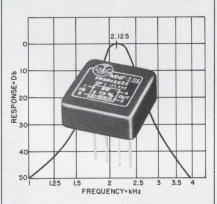
Designing for modem applications? You'll find this MNF 2.125 band-pass filter precisely what you need. It has a center frequency of 2125 Hz and a pass band from 2025 to 2225 Hz within 1 db. Impedances are 10K ohms source and load.
