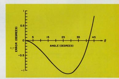
28. The accuracy of Circuit I is the difference between  $\theta$  and its approximation,  $\sin\theta/(\cos\theta + K \sin\theta)$ . Maximum error from 0° to 45° for K = 0.25 is <1.2°
