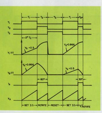
35. Operation of the Type V converter is divided into three modes. T1 sets initial conditions, T2 rotates vector R, T<sub>3</sub> resets integration capacitor voltage to zero.
