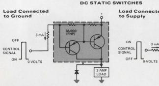
Put In Either Polarity. Positive or negative-based systems are possible with your choice of either PNP or NPN devices that can also be used as complements in audio amplifiers.
