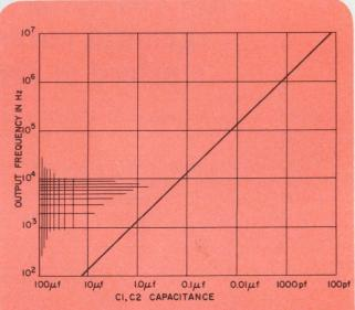
2. Linear relationship exists between capacitance and frequency for a wide range of capacitor values.
