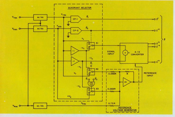
30. A reference voltage generator is used in the Circuit II design. Thermally induced variations in the transfor-
