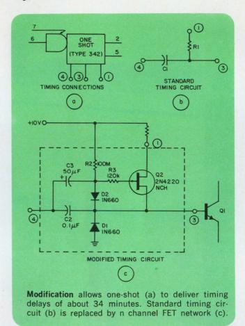
through C, since  $Q_2$  will not come on if this leakage is excessive.
