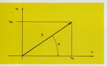
33. The imaginary vector  $\overline{\mathbf{R}}$  has the two integrating capacitor voltages  $V_{10}$  and  $V_{20}$  as components.  $\overline{\mathbf{R}}$  rotates with a constant velocity,  $K\omega$ .
