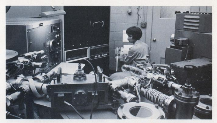
Mass spectrometer measurements are run in a laboratory environment under the control of a minicomputer.
