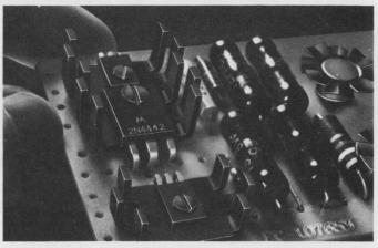
Power levels of plastic power devices such as X58's, MS9's, and M386's can be increased up to 80% in natural convection and 500% in forced air when used with PA and PB Dissipators. PA's need only .65 sq. in. to mount; PB's 1.17 sq. in. Staggered finger design gives these light-weight dissipators their high efficiency.
