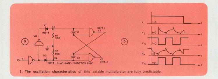
LOW level at  $V_{1b}$ . These levels will clamp  $V_2$  and  $V_4$ , respectively, negative (LOW) and positive (HIGH). The LOW level at  $V_2$  will cause  $V_3$  to be HIGH. Because of the NAND gate function, this HIGH level combined with the clamped HIGH level at  $V_4$  will cause  $V_5$  to be LOW. Note that under these conditions, no charge is stored in either  $C_1$  or  $C_2$ .
