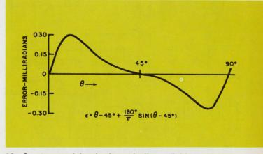
29. Greater precision is theoretically available from the Type IV converter—Circuit II. Error between  $\theta$  and its approximation (Eq. 59) from 0° to 90° is <1.0 minute of arc.
