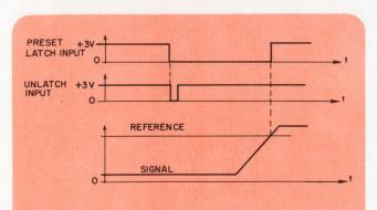
2. **Negative pulse** on preset latch and unlatch inputs sets up comparator to detect reference/signal equality.
