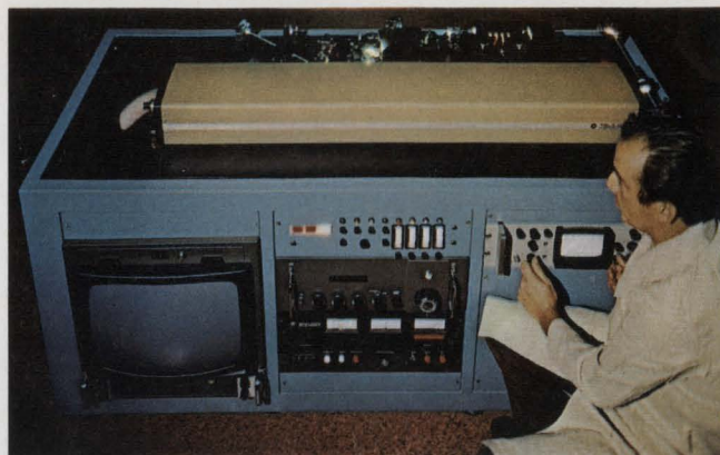
Laser color television projector , from General Telephone & Electronics Laboratories, produces pictures off the air with a single multicolor laser, single modulator and single scanner (Session 3E).
