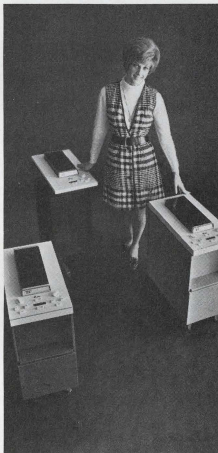
magnetic tape data terminals: Use compact reusable tape cartridges. Operate on-line at up to 2400 wpm, and connect "locally" to lower speed Teletype terminals using ASCII code.
