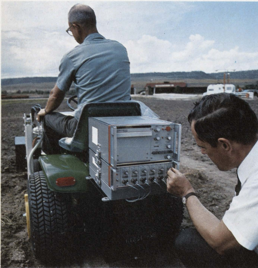
Portable on-board instrumentation is used for tractor testing. This Honeywell multiple-channel Visicorder is recording cylinder-head temperature, exhaust temperature and tractor-frame dynamics to check the suspension.
