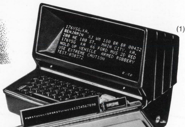
32/37, 80 Character Position Panel, 5 x 7 Dot Matrix, Characters 0.2" High. Alphanumeric panel with 64-character format.
