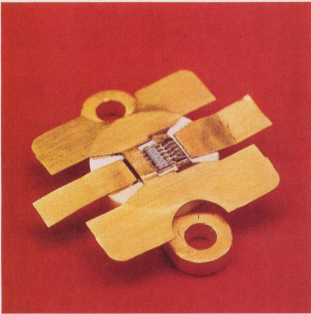
Motorola's Controlled-Q package reportedly offers a reduction in device Q for increased bandwidth, together with increased package input impedance.
