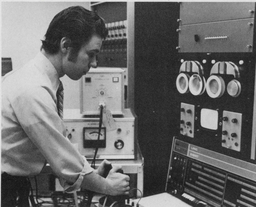
Minicomputer helps evaluate heart defibrillators. The output of the defibrillator is sampled by the computer, which then calculates the energy that the instrument delivers.
