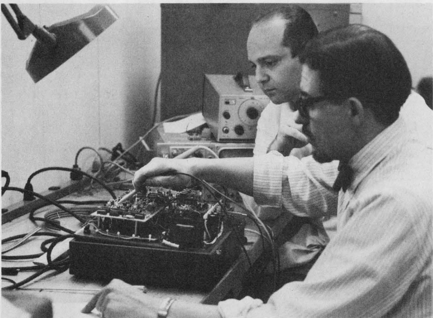
Electrocardiograph tester developed by the institute is being checked out. A semiautomatic device, it speeds evaluation of equipment.
