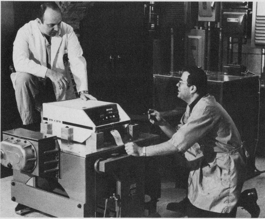
Shake test is among the stresses that the institute employs to check the ruggedness and reliability of medical electronic equipment.
