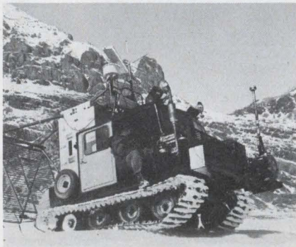
This snow cat carries a Ruggednova interfaced with two radar systems to help map the Canadian glacial fields.
