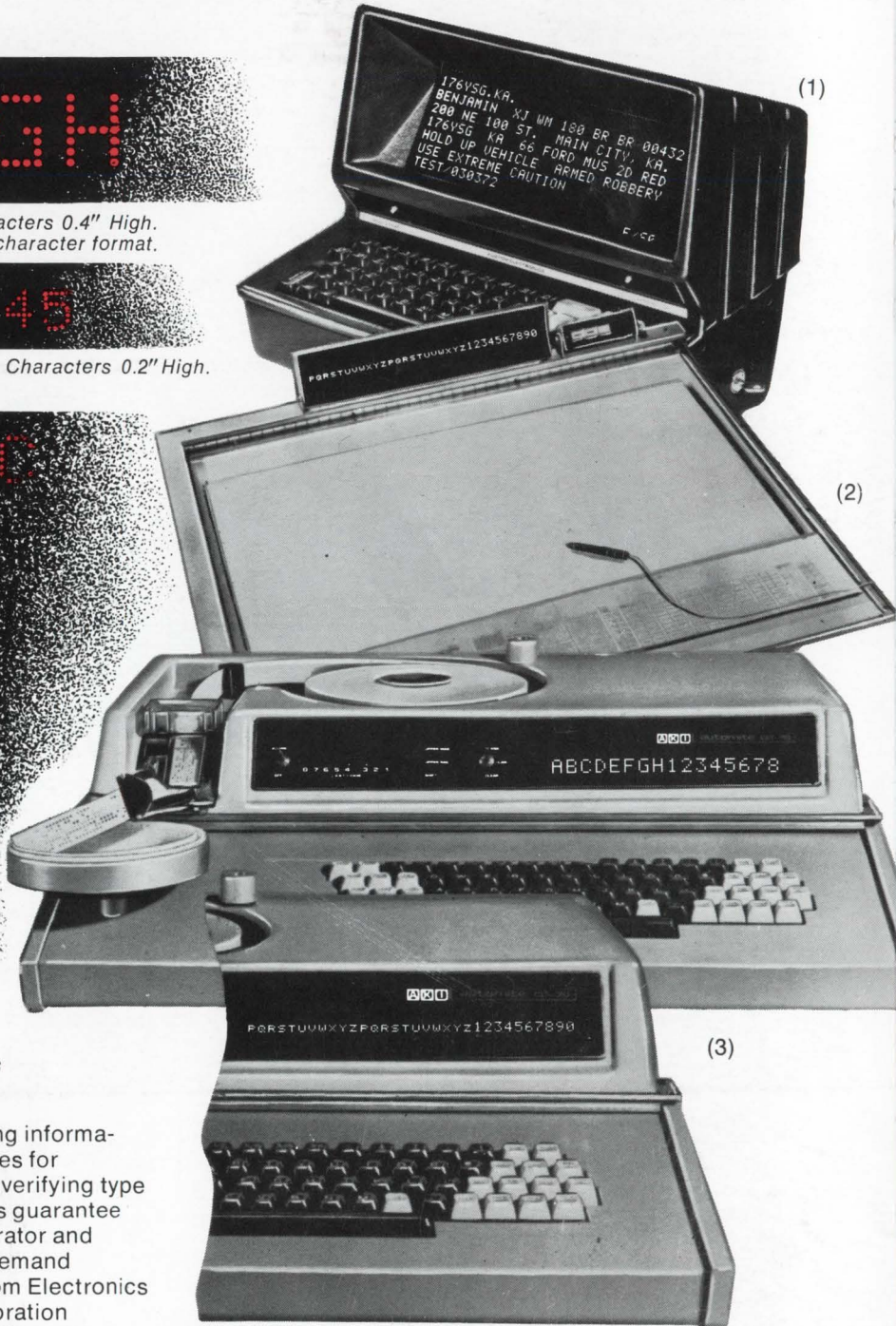
SELF-SCAN Panel Display Subsystem, 256 Character Capacity, 5 x 7 Dot Matrix, Characters 0.25" High. 64-character format, available with all drive electronics including memory, character generator, and timing.
