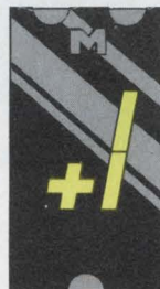
MAN 83 Common Anode; Overflow ( \pm 1 )
