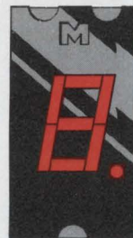
MAN 74 Common Cathode; Right Hand Decimal
