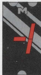
MAN 73 Common Anode; Overflow ( \pm 1 )
