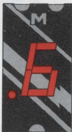
MAN 72 Common Anode; Left Hand Decimal
