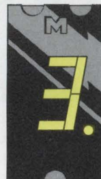
MAN 84 Common Cathode; Right Hand Decimal
