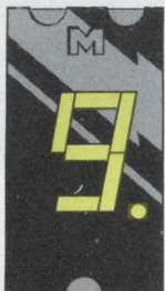
MAN 81 Common Anode; Right Hand Decimal
