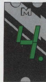
MAN 54 Common Cathode; Right Hand Decimal
