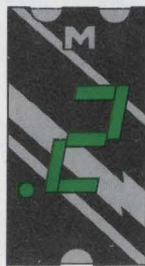
MAN 52 Common Anode; Left Hand Decimal
