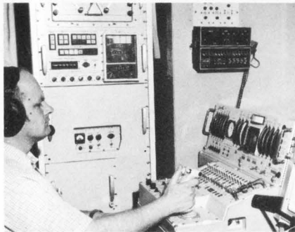
A new technique for armchair control of RPVs (Remotely Piloted Vehicles) has been developed by Motorola Government Electronics Division for the Navy. The Ruggednova in the background helps provide either discrete or proportional control for up to six RPVs of any variety at ranges exceeding 250 nautical miles.
