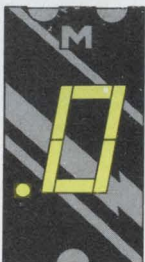
MAN 82 Common Anode; Left Hand Decimal
