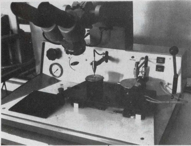
2. Epoxy pads for mounting components can be accurately placed by well-designed machines.
