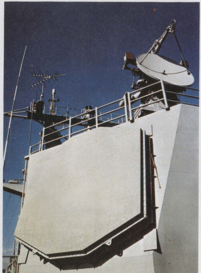
The U.S. fleet's air defense system, Aegis, developed by RCA, includes a phased-array radar, AN/SPY-1, that automatically detects and tracks multiple targets while maintaining surveillance coverage of the air.
