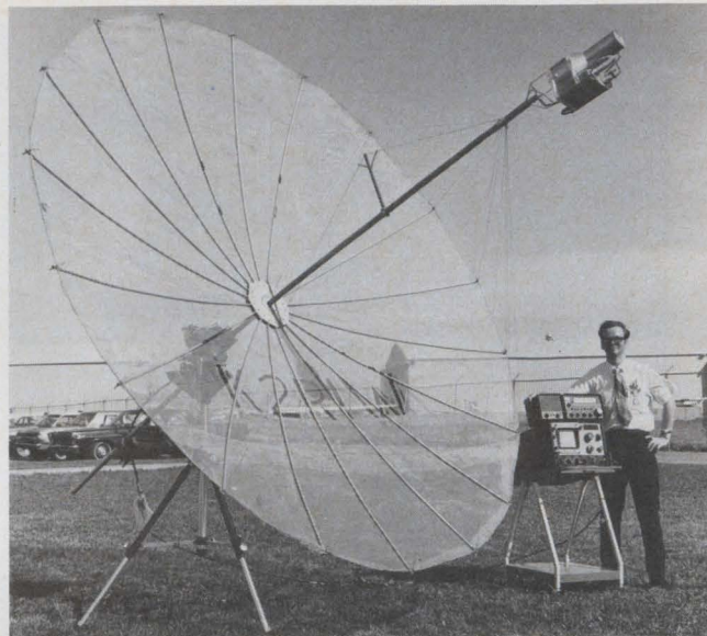
Voice signals from Apollo 15 and 16 astronauts on the moon, were received by radio amateur Richard Knadle using his home-made $42 parabolic antenna. Transmitter power on the moon was only 13 W.
