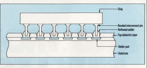
the sites. Then, the BIP chip is placed in position on the substrate and reflowsoldered to the interconnection sites.
