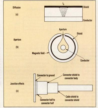
skin depth. For the most common metals, only a few thousandths of an inch thickness is required at higher frequencies to satisfy the three-skin-depths criterion. In cases where only moderate shielding is needed, a thinner shield may be used as long as high conductivity is maintained.
