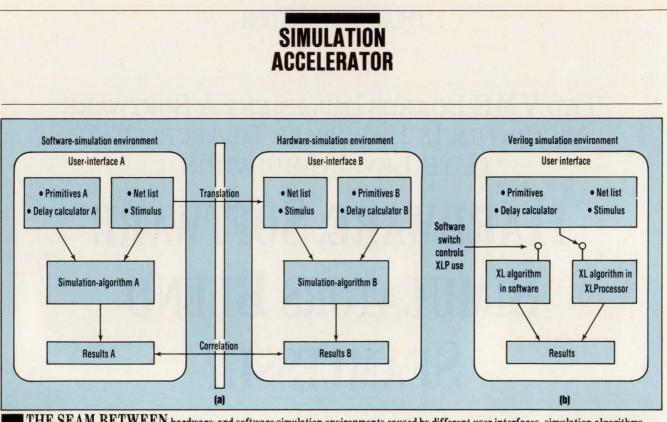
THE SEAM BETWEEN hardware- and software-simulation environments caused by different user interfaces, simulation algorithms, primitives, and delay calculators can produce different results and incur a large amount of overhead (a). The Verilog environment has no seam because the hardware and software simulators use the same primitives, delay calculator, net list, stimulus, and user interface. A software switch determines if the simulation is sent to the hardware accelerator (b).
