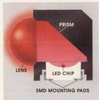
The introduction of the PRISM CBI means there is one less component on the board that has to be through-hole mounted because now a reliable surface mount version exists. Using this
