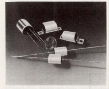
A series of MIL-quality, metallizedpolycarbonate-film capacitors features a 50% smaller package than standard capacitors with no sacrifice in performance. The 5MC capacitors are specifically designed for switchmode power applications. Five available configurations include axial leads with tab terminations in high or low profile, and internal coaxial leaded with or without grounded copper shielding. Call for pricing and delivery.
