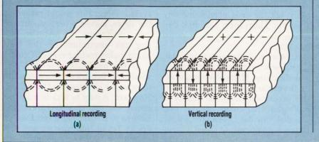
The vertical-recording disk is comprised of two layers. The top layer stores the data; the lower layer is a soft magnetic material that conducts the magnetic flux to the return pole in the recording head. This lets the head and media operate as a unified system.
