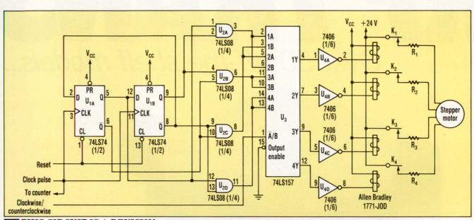
THIS CIRCUIT IS A REVISION of a previously published bidirectional stepper-motor sequencer. The new circuit uses four chips, with an option of using just three (the flip-flops and AND gates can be combined). The rate of clock pulses determines the motor's rpm. Switching transistors can replace the relays to increase the circuit's efficiency.
