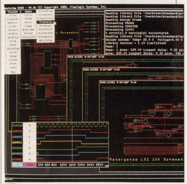
IN THIS EXAMPLE, the Retargeter software optimizes the Actel FPGA design located in the upper-left window, and maps it into an LSI Logic 10k gate array. The retargeted design is in the lowerright window. Viewlogic's Viewsim tool simulates both designs and compares the results in a single window in the lower left.
