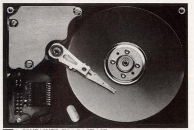
1. CONTAINED IN A PACKAGE that's about 2-3/4 by 4 in. (shown here in actual size), Seagate's ST9051A drive holds 40 Mbytes of data. The media is made of thin-film aluminum. The drive uses just 0.5 W in the standby mode. E L E C T R O N I C D E S I G N 33 MAY 23, 1991
