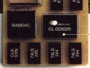
This full 16-bit CL-GD5320 lets you implement 16-bit or 8-bit VGA capabilities on your motherboard with as few as 5 other chips and two 256K x 4 DRAMs. Get a complete solution that saves time, space, power, and expense. You still get all the speed, features and flexibility you're looking for.
