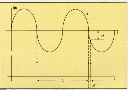
4. THIS EXAMPLE OF A SINE WAVE sampled by a clock of period  $T_s$  shows how the effects of aperture jitter increase with the input's slew rate. For a given jitter ( $\Delta t$ ), the voltage error ( $\Delta V$ ) increases as the slew rate increases.
