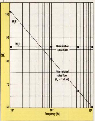
5. DESIGNERS CAN PREDICT the theoretical limits of the rms-signal-to-rms-aperture-jitter noise ratio,  $SN_jR$ . For an rms aperture uncertainty,  $t_a$ , of 150 ps, performance begins to degrade above 53 kHz, approximately. Also shown on this plot is the maximum SNR that can be achieved if only quantization noise is considered.
