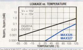
The MAX326/327 offer at least 100 times less typical leakage at +25°C than DG201/202
