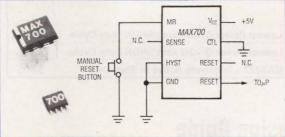
The MAX700 includes a 5V monitor, RESET and RESET outputs, and debounced manual reset input, but consumes only  $200\mu$ A.
