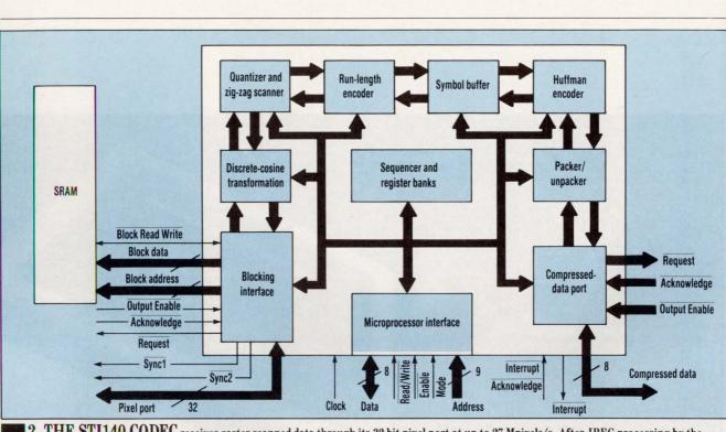
2. THE STI140 CODEC receives raster-scanned data through its 32-bit pixel port at up to 27 Mpixels/s. After JPEG processing by the codec, compressed data exits through an 8-bit port at the same data rate for synchronous or asynchronous operation.
