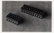
A line of surface-mounted DIP switches is designed for automaticinsertion equipment. The ESM Series switches are offered in up to 10 positions. Top tape sealing for board washing is optional. Material is UL 94V-O-rated and contacts are gold plated. An eight-position switch costs \$1.26 in lots of 1000. Delivery is in four to six weeks.
