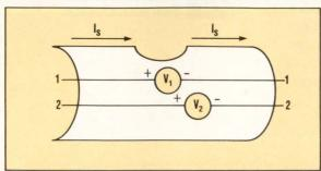
1. A good measure of a shield's performance is its transfer impedance. This parameter is defined as the ratio of the longitudinal voltage source in series with the conductors to the shield's surface current. The lower the transfer impedance, the more effective the shielding.
