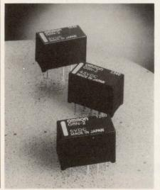
standard for some seven years. A principal feature of the relay is its 2.5-kV surge-withstand voltage between coil and contacts. That's a significant improvement compared with the 1.5-kV requirement of the previous operative standard, which was defined by FCC Part 68.
