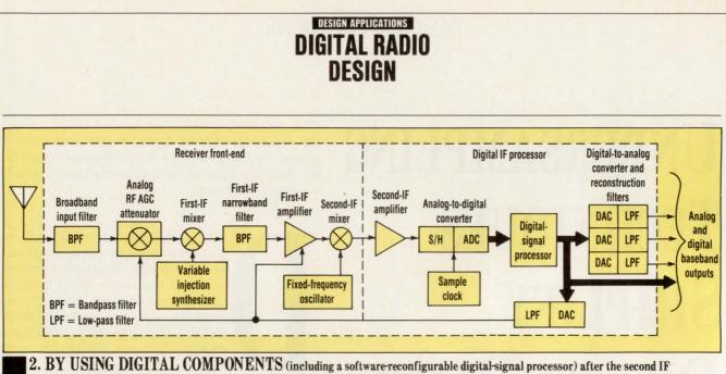
2. BY USING DIGITAL COMPONENTS (including a software-reconfigurable digital-signal processor) after the second amplifier, designers can simplify the receiver circuit and reduce costs.
