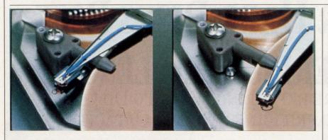
2. THE RAMP-LOADING TECHNIQUE, designed by PrairieTek, increases the drive's reliability by keeping the head from making contact with the disk. The head lays on the plastic surface when the disk is turned off.
