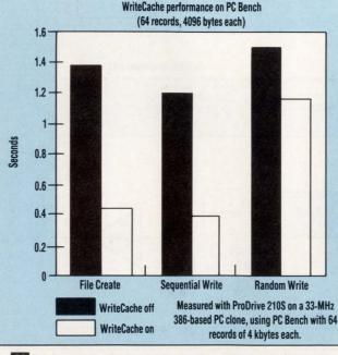
increase in the sustained data-transfer rate of 50 to 200%. However, by studying the way data is accessed and stored, engineers at Quantum Corp., Milpitas, Calif., have developed a scheme that lets them exploit write-caching benefits, particularly because the time needed for data storage is usually less than 25 ms.
