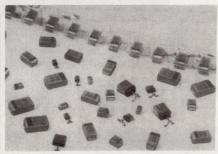
Designed specifically for surface mounting directly to pc boards or alumina substrates, the T491 series of precision molded tantalum chip capacitors withstands a variety of processes. The chips can be wave soldered, infrared reflowed, or vaporphase soldered. Values range from 0.1  $\mu$ F to 150  $\mu$ F with  $\pm 10\%$  and  $\pm 20\%$  tolerances available. Working voltages range from 4 to 50 V dc. Call
