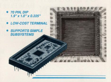
The input clock frequency is selectable for either 12 or 16 MHz operation. This helps support a number of different applications with enhanced zero crossing distortion tolerance and provides superior word error rate performance.
