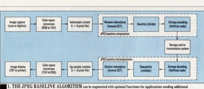
1. THE JPEG BASELINE ALGURITHM can be augmented with optional functions for applications needing additional compression and decompression features. The extended system enables the encoder to handle pixels with greater than 8-bit precision, additional data-interleaving schemes, and more color components. It also provides arithmetic coding for up to 10% better compression, and progressive build-up to successively improve an image as more data becomes available.
