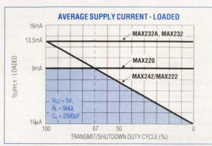
To conserve power, use the MAX220 when transmitting data more than 2/3 of the time. Use the MAX222/MAX242 with shutdown when transmitting less than 2/3 of the time.
