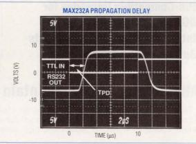
The MAX232A improves propagation delay and symmetry.
