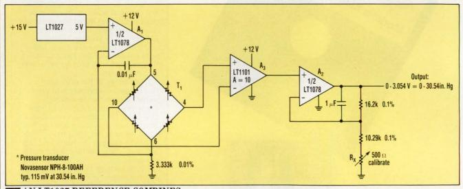
AN LT1027 REFERENCE COMBINES with an op amp  $(A_1)$  to send exactly 1.5 mA through transducer  $T_1$ . The gains from  $A_2$  and  $A_3$  yield an output that's calibrated directly in inches of mercury.
