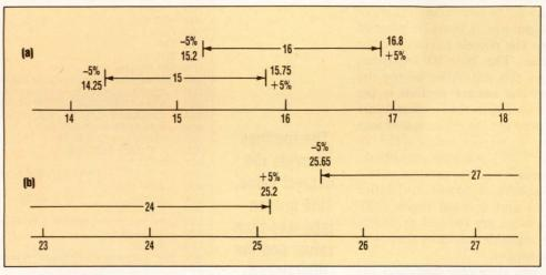
1. Computation results, such as 15.525, fall within 5% of two standard values (a). On the other hand, 25.44 isn't within 5% of any standard value.
