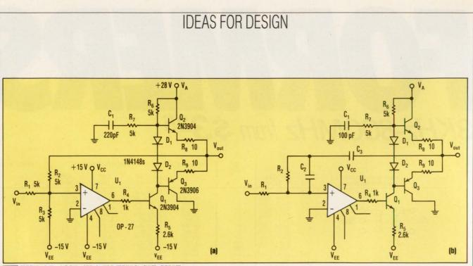
THE OP AMP (U1) IN THIS CIRCUIT operates from a standard ±15-V supply and its output is scaled from 5 to 25 V (a). With a slight modification, the circuit becomes an active lead-lag filter that can drive an rf or microwave voltage-controlled oscillator directly (b).
