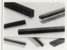
includes straight and right-angle options on single and double rows with up to 36 positions per row. Pricing is from \$0.025 per pin. Delivery is in five days for up to 1000 pieces.
