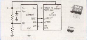
The MAX690 features a 5V monitor, battery backup switch, watchdog timer, and a comparator for early power-fail warning or battery sending.
