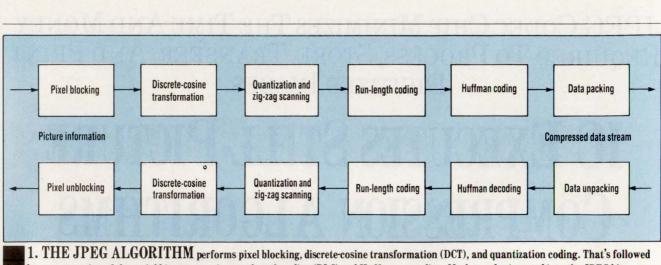
by a compression of the serial bit stream using run-length coding (RLC) and Huffman encoding. Marker codes inserted into the JPEG bit stream ensures agreement between encoder and decoder.
