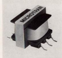
ries units are designed for dry-circuit, 600- $\Omega$  lines and have a frequency response of 300 to 3500 Hz  $\pm 0.5$ dB over a power-level range of -45 to +7 dBm. Distortion is 0.5% maximum. Pricing in large quantities is about \$3. Delivery is from stock.
