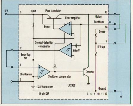
the LP2952 comes in a 14-pin DIP and the LP2953 in a 16-pin DIP. The LP2954 also comes in a standard 3pin TO-220 package. It can drop in to the socket of an LM340, a 1-A conventional linear regulator that needs at least 2.5 V across it, regardless of load current.
