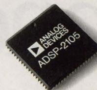
**ADSP-2105**—High performance DSP at an incredibly low price. So low, in fact, you can now consider DSP in a host of new applications. And since it's pin-compatible with the ADSP-2101, and code-compatible with all of our other DSP processors, upgrading is easy and inexpensive.
