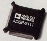
ADSP-2111—Better integration on the best architecture in the industry. Adds an 8/16-bit host port to the two serial ports, timer, hardware companding and memory already on the ADSP-2101. And like all our DSPs, it's got fast, flexible arithmetic, wide dynamic range and a single cycle fetch of two operands (on- or off-chip). Plus it's code-compatible with the rest of our DSP family, so what's written today will be useful tomorrow.
