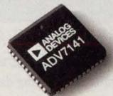
ADV7141—Our new Continuous Edge Graphics™ RAM-DAC gives users of standard low-end color monitors better graphics on their PCs. Graphics that are virtually the same as those produced on expensive engineering and scientific workstations. It does this by eliminating jagged edges, providing photo-realistic colors and shading, and displaying text comparable to a 300-dpi laser printer.
