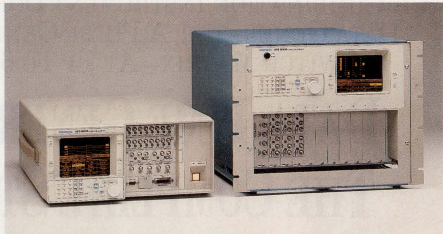
1. THE HFS 9000'S MODULAR FORMAT lets designers choose between a three-slot mainframe that supplies up to 12 channels (left) and a nine-slot chassis that accommodates up to 36 channels.
