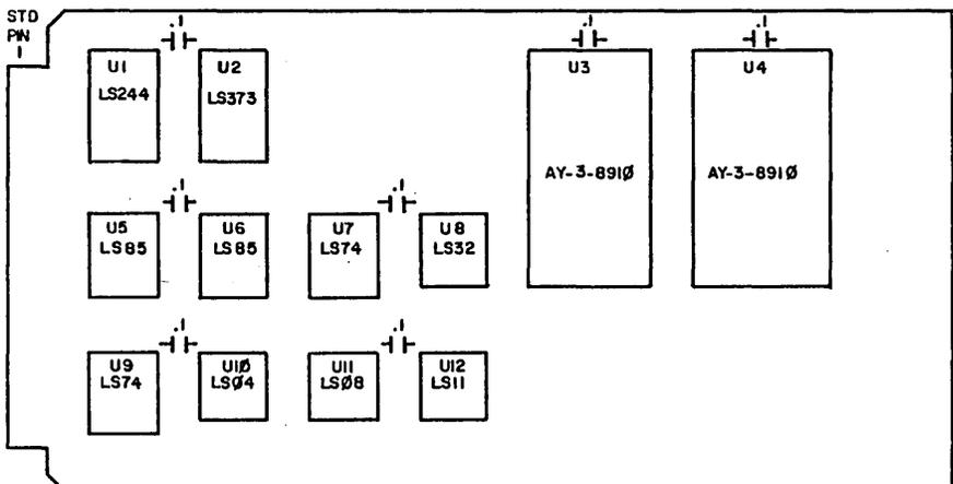
Figure 4 - STD BOARD IC Layout
