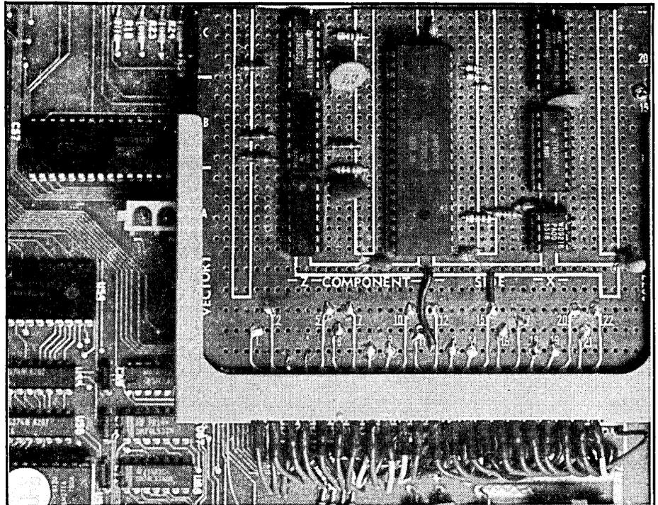
New disk controller card mounted on flexible leads on the Xerox 820-II motherboard. The card plugs into a 44 pin socket which is wired to the J12 connector pads.
