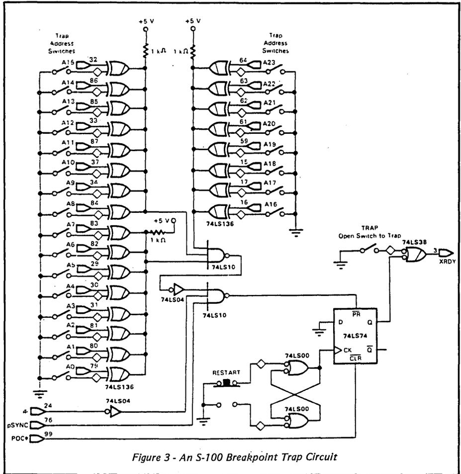
Figure 3 - An S-100 Breakpoint Trap Circuit
