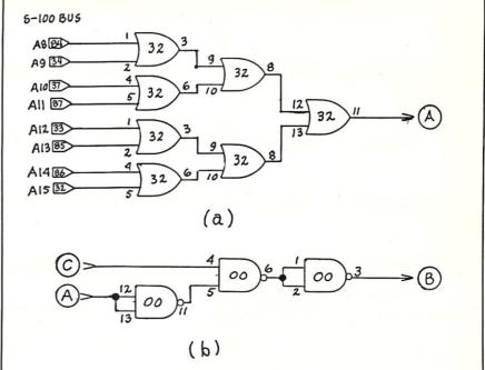
Figure 1 - a)Address decoding of A8 to A15. Required for all three CompuPro boards. b) Circuit that ANDs low byte
