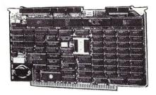
The CPZ-186 can be used as a single board computer or as a master (file server) in a local area network. Up to 4,000 users can be linked to up to 255 file servers, in combination, via ICM's ARCnet hardware and TurboLAN software. Users can be IBM-PC's, AT's, Jr's, PC compatibles, S-100 systems etc. A multi-user system can be built using Software 2000's TurboDOS and TurboDOS/PC with CP/M, MP/M, MS-DOS, CP/M-86 and PC-DOS compatibility.
