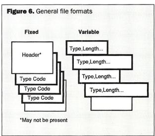
teristics. After the header they get down to a repetition of fixed-length database records. With dBASE, each record is of fixed size, preceded by an active/deleted flag. SMART uses a 2-byte prefix on each record to define the length of the following record, with a high-order bit flag showing active and deleted status. For fixed-length Data Manager files, the length value is the same for each record. A variable-length record format is also available.
