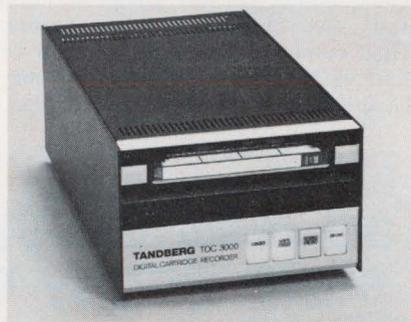
mother board. One formatter handles four recorders. Data transfers to and from the formatter can be either eight bits parallel or bit serial, buffered or unbuffered, depending on the I/O controller. Recording is 1600 bpi. *Tandberg, Berkeley, CA.*
