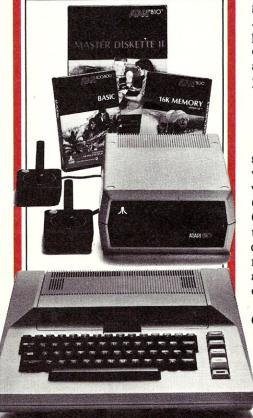
business accounting, play video games. Programmable in Basic or Assembly, the 800 can use all Atari peripherals and can control up to four disk drives and a 60 lpm printer. In all, the 800 and its accessories form a package worth a full \$1620 at retail!
