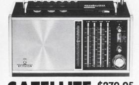
The world's finest all-wave, high-fidelity portable . . . the Grundig Satellite offers no-gap international short wave reception from 10 to 187 meters, with unsurpassed station separation and noise suppression. Exclusive band-spread selector covers frequencies from
