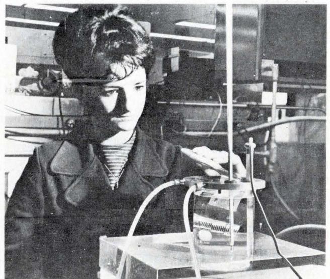
IC receiving a gross-leak test using an inert liquid.
