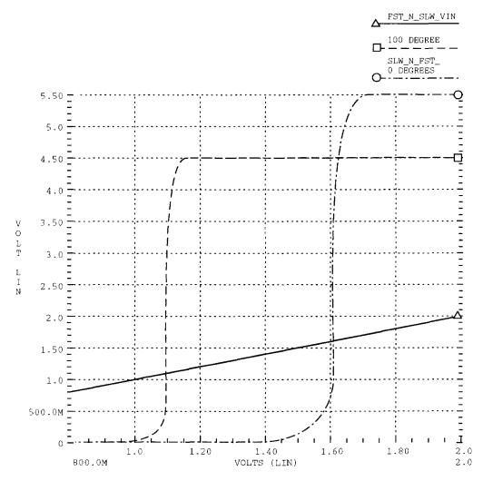
PCI Bus Inputs VIN vs. VOUT, Fast N, Slow P, and Slow N, Fast P, 5 volts
