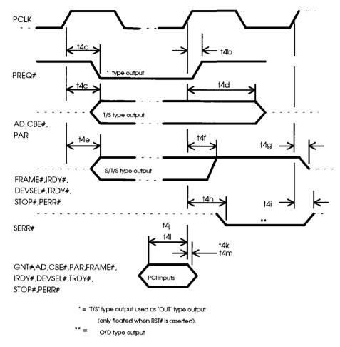
Figure 9-12. PCI Signal Input Output Timing
