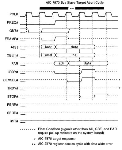
Figure 10-9. Slave Target Abort (width error)
