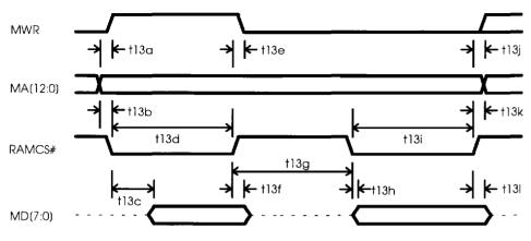
Figure 9-21. Sequencer Read-Modify-Write Memory Port Timing
