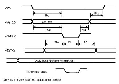
Figure 9-17. PCI SRAM Write Memory Port Timing
