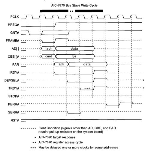
Figure 10-6. Slave Single Transfer Write
