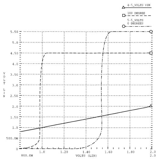
PCI Input VIN vs. VOUT, Fast N, Slow P, and Slow N, Fast P, Always 5 volts
