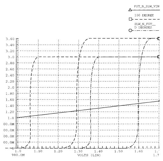
PCI Bus Inputs VIN vs. VOUT, Fast N, Slow P and Slow N, Fast P, 3.3 Volt
