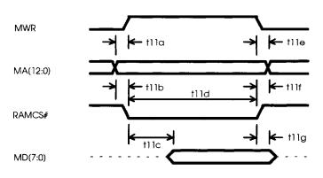
Figure 9-19. Sequencer Read Memory Port Timing
