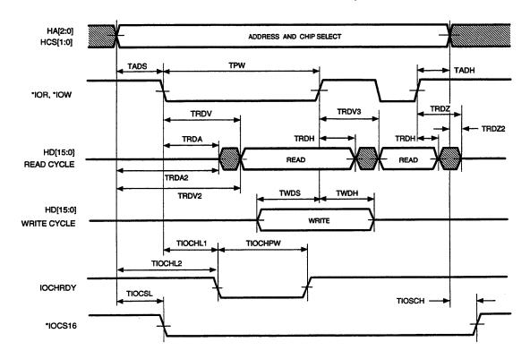
Figure 8-34 AT PIO Timing
