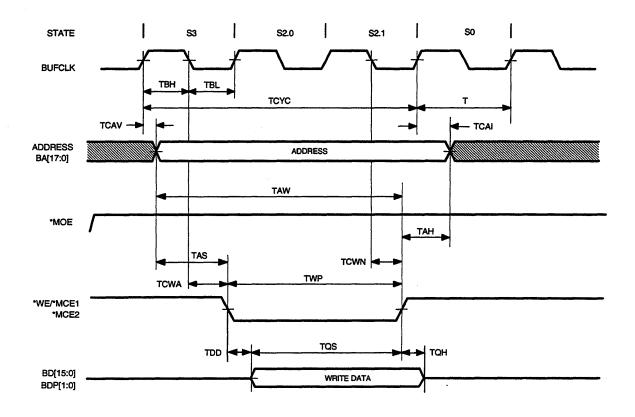
Figure 8-14 SRAM Timing (Write, 3T Access)
