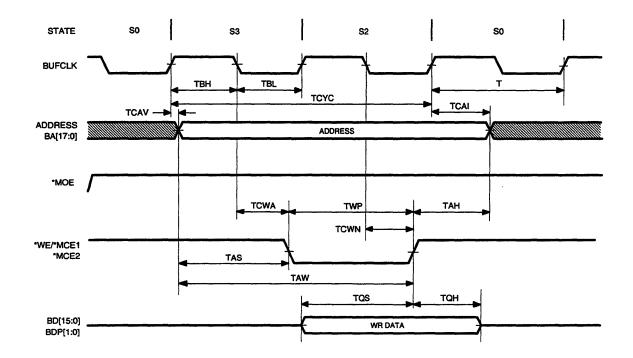
Figure 8-13 SRAM Timing (Write, 2T Access)
