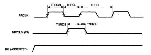
Figure 8-27 Single- and Dual-Bit: Disk Read Timing
