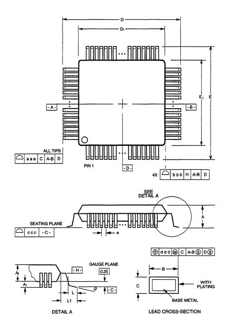
Figure 9-2 128-Pin TQFP Package Outline
