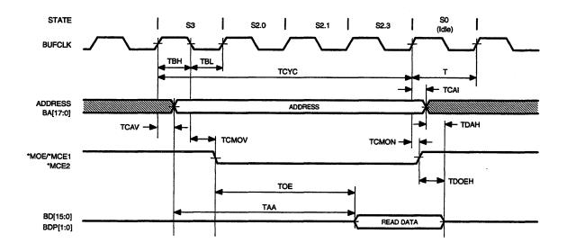
Figure 8-11 SRAM Timing (Read, 4T Access)
