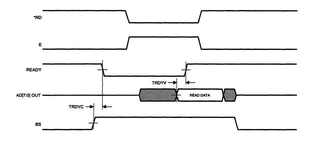
Figure 8-6 Microprocessor Ready Timing (Buffer RAM Read Cycle)
