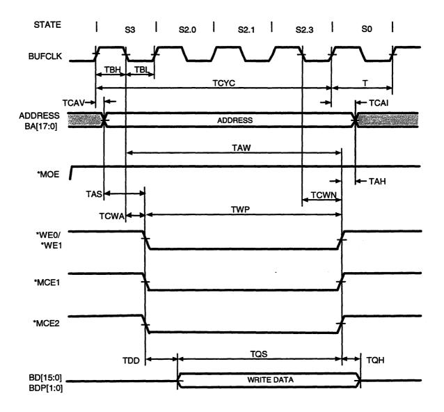
Figure 8-15 SRAM Timing (Write, 4T Access)
