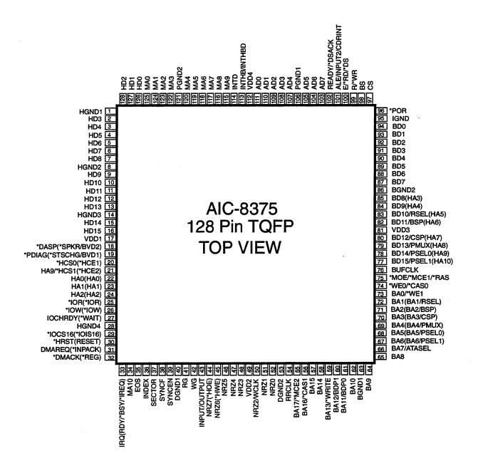
Figure 2-2 AIC-8375 TQFP Pin Assignments
