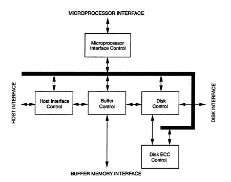
Figure 1-1 AIC-8375 Block Diagram
