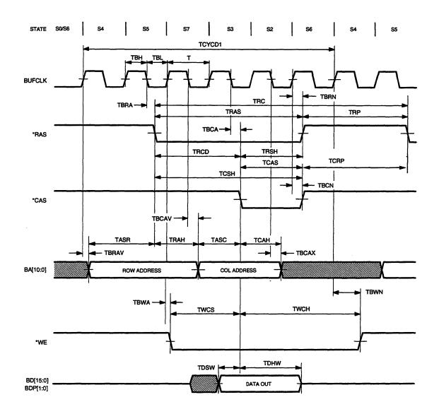
Figure 8-19 DRAM Timing (No Wait State, One Byte Write)
