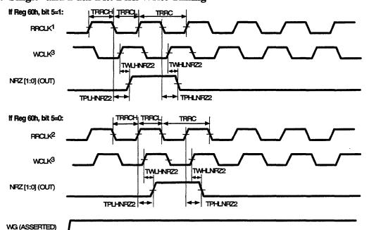
8.4.4 Single- and Dual-Bit: Disk Write Timing
