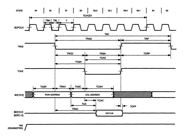
Figure 8-18 DRAM Timing (Wait State, One Byte Read)
