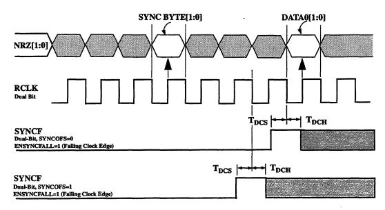
*NOTE:* SYNCF is shown for Sync Offset = 0 and =1. SYNCF can be internally delayed to get the alignment shown here. See DCTL1 Reg 61h, R/W, bits 2:0.
