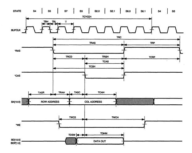
Figure 8-20 DRAM Timing (Wait State, One Byte Write)
