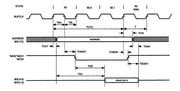
Figure 8-10 SRAM Timing (Read, 3T Access)
