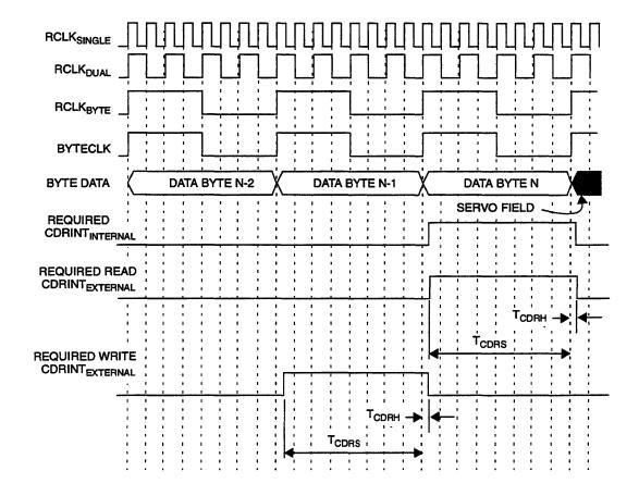
Figure 8-33 External CDR Interrupt Timing
