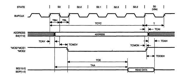
Figure 8-12 SRAM Timing (Read, 5T Access)
