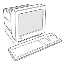
This terminal can emulate a number of ASCII and ANSI terminals, including PC-Term and SCO<sup>TM</sup> Console. The keyboards supported by the terminal include the 101/102 key extended PC (EPC), the 106/107 PC/+, the VT220<sup>TM</sup>-style ANSI keyboards, and ASCII keyboards.
