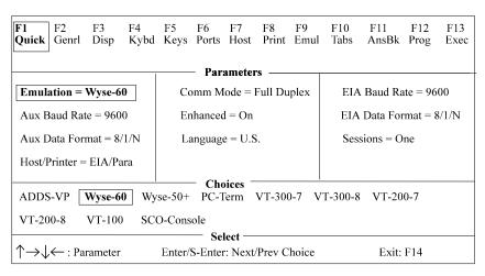
Emulation: ADDS VP, Wyse 60, Wyse 50+, PC Term, VT300/8, VT300/7, VT200/8, VT200/7, VT100, SCO Console, AT386, TVI 925
