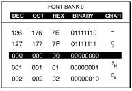
Characters appear in decimal, octal, hexadecimal, and binary number representations. The CHAR column contains the ASCII representation of the character. Use the following keys to change the display of the ASCII chart:
