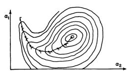
Figure 2a. Optimum Gradient Method.
