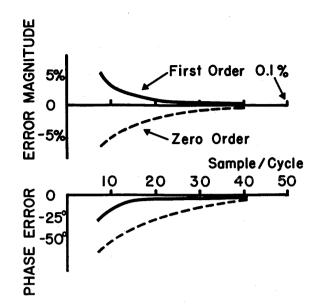
Figure 13. Zero and first order conversion methods are compared, after filtering. The errors are functions of the number of samples per cycle of full scale signal frequency. A good rule of thumb for the zero order filter is that 50 samples per cycle, the errors are less than 0.1% and 3.6 degrees.
