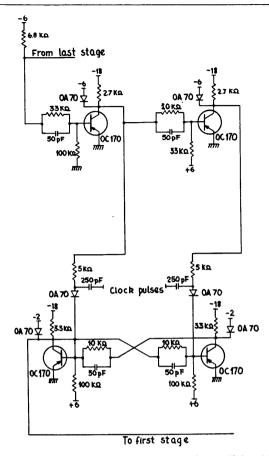
Figure 17. Carry Feedback on a Serial-Parallel Adder.
