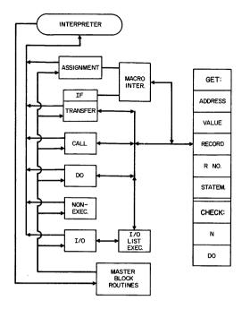
Figure 2.7c. General Diagram of Process Control Flow —Interpreter.
