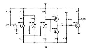
Figure 7. Schematic of Discriminating Amplifier.
