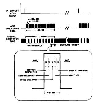
Figure 7. Typical times are shown for the steps in the conversion cycle of the example system of Figure 5. All ten channels are converted and stored in memory as fast as possible before proceeding with calculations—at the expense of intervals of "waiting time."
