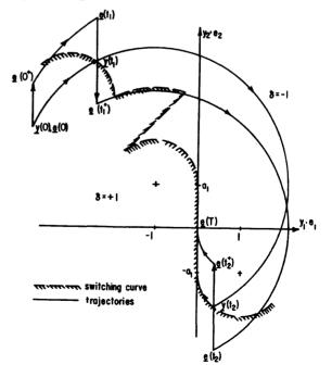
Figure 7. Optimum Trajectories of e(t) and y(t) (minimum time).
