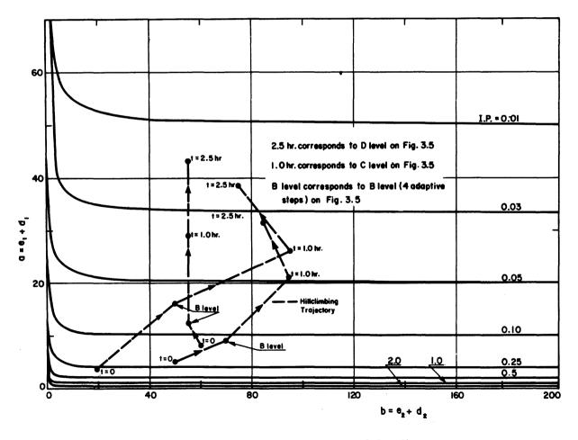
Figure 4. Index of Performance for I =  $\frac{k(b+1)}{ab}$
