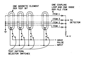
Figure 2. Core-Wiring Arrangement for MIRF Memory.
