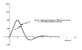
Figure 9. Output Response for a Pulse Input for Circuit Shown in Figure 8.
