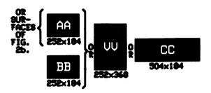
Figure 2a. Names and sizes of surfaces large enough to hold complete fine-resolution movie frames (252 x 184). Alternate uses of total 7090 storage area are indicated, including the uses of region AA in ways shown in Fig. 2b.
