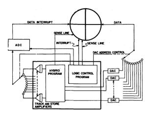
Figure 8. Several improvements to the interface system of the example of Figure 5 include: simultaneous sampling, external ADC and multiplexer timing by a parallel logic program, use of sense lines to reduce conversion channels, detection of random events, multiple sampling frequencies, and/or asynchronous sampling.
