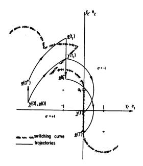
Figure 9. Optimum Trajectories of e(t) and y(t) (minimum time).
