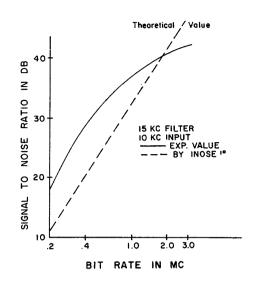
Figure 12b.  $\triangle \Sigma$  S/N Ratio as a Function of Bit Rate.
