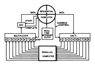
Figure 5. An early hybrid system configuration. The sequential program controls the timing of the conversion cycle. The cycle is initiated by the "interrupt clock." For a tyical problem the clock might be set for 100 cps; and 7 to 8 milliseconds per cycle would be available for calculation.
