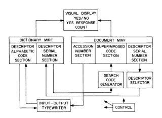
Figure 1. Simplified Block Diagram of MIRF Experimental Model.
