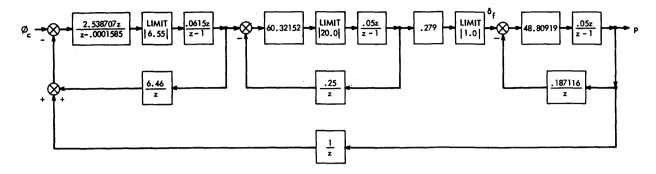
Figure 12. Roll Channel Z Transform Transfer Function (Roots and Steady-State Gain Unadjusted).
