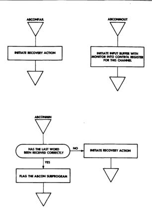
Figure 8. Interrupt Flow Diagram.
