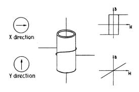
Figure 3. An Isolated Specimen of Magnetic Thin Film, showing its magnetic characteristic on the X and Y Directions. magnitudes: 1) Input currents, 2) Remanent magnetization states, 3) Voltage outputs.
