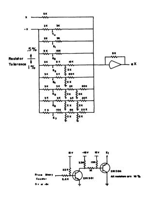
Figure 16. D/A Multiplier and Switch.
