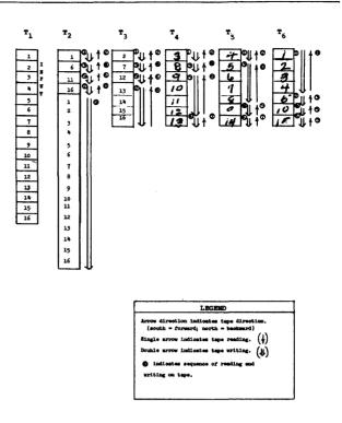
Figure 2. Tape Motion of Read-Backward Oscillating Merge.
