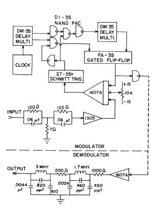
Figure 6.  $\Delta \Sigma$  Modulator Demodulator.
