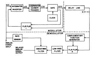
Figure 1. Block Diagram of Analog Delay Unit.
