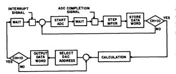
Figure 6. The sequential program flow diagram, for the example hybrid system of Figure 5, shows the steps required for control of the converters.
