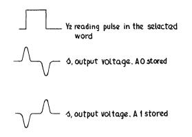
Figure 6. Reading Pulse and Outputs in the Ternary Store.
