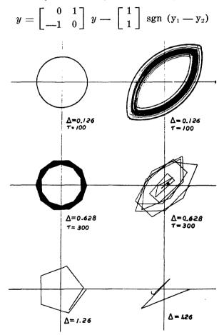
Figure A-2. Trajectories showing the effects of different integration step sizes ( $\triangle$ ) on the Runge-Kutta method. Period of unforced system being integrated was T = 6.2836.
