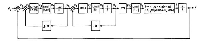
Figure 1. Transfer Function Diagram for Aircraft Roll Channel.
