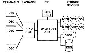
Figure 1.1. Remote-Computing System: Equipment Configuration
