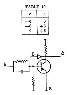
Figure 7. Fundamental Connection for the Active Stages.
