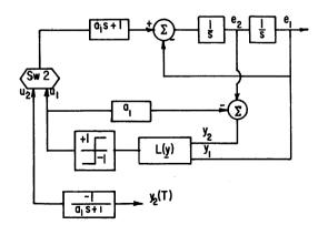
Figure 16. Block Diagram of the Controlled Plant.
