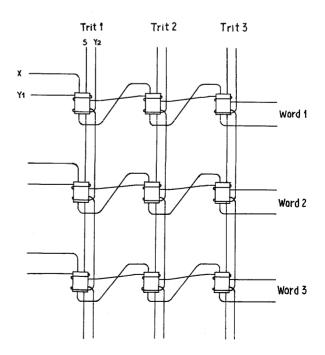
Figure 4. Word Selection Array. Three Words of Three Bits Each.
