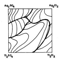
Figure 3. The function defined represents a system composed by particular percentages of each of the four compounds shown at the corners. Contour lines are drawn in order to indicate values of a property on the system. The heavy lines are lines of discontinuity in slope.<sup>5</sup>
