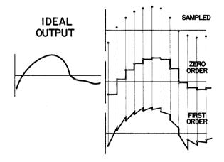
Figure 12. The discrete to continuous signal conversion requires smoothing and hence yields only an approximation to the ideal output from the sequential computer. The zero order conversion simply holds the output voltage at the last sampled value until the next arrives. When the "steps" are filtered out the result is shifted in time by the width of one half step. The first order scheme uses the past two converted values to predict the value between points, before "resetting" to the next value.
