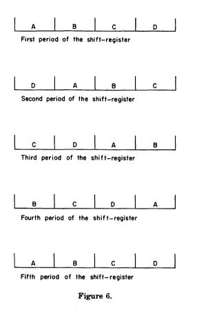
outputs have the same binary sequence, but each of them is delayed from the previous one by approximately 8, 388, 608 bits. That is, for the outputs A(t), B(t), C(t) and D(t),
