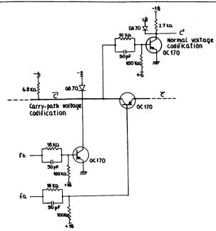
Figure 15. Carry Propagation: Electronic Diagram of a Typical Stage, Including Normalization of Voltage Levels.
