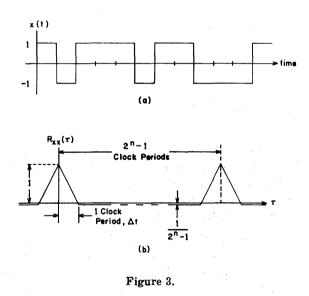
shows the autocorrelation function of a maximum length sequence x(t). It can be seen that for time delays equal to or greater than one clock period, the correlation is essentially zero for large values of n.
