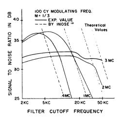
Figure 12e.  $\triangle \Sigma$  S/N Ratio Using Four Bit Rates.
