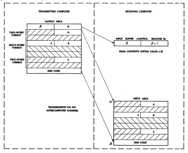
Figure 6. Intercomputer Buffer Format.
