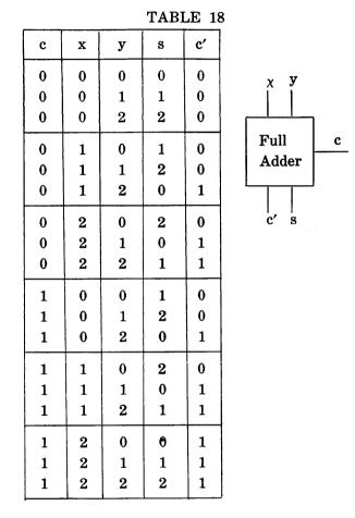
The case c = 2 is not included because the propagation of any carry value other than 0 or 1 is not possible in a full adder, whichever the numerical base used.
