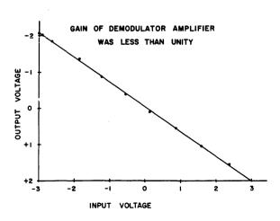
Figure 5. Static System Response.
