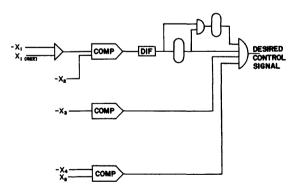
Figure 9. A parallel logic program is used to detect random events in the parallel computer. The "desired control signal" interrupts the sequential program when the overshoot in  $x_1$  exceeds  $x_2$  after the third oscillation; but only when  $x_s$  is negative and  $x_4$  is less than  $x_5$ .  $x_1$  through  $x_5$  are analog voltages.
