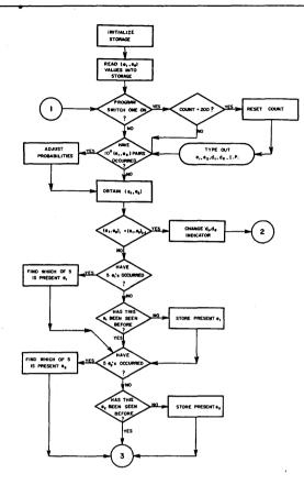
Figure 6. Flow Diagram (Part I).
