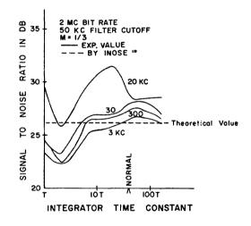
Figure 12a.  $\triangle \Sigma$  S/N Ratio Using Four Modulating Frequencies.
