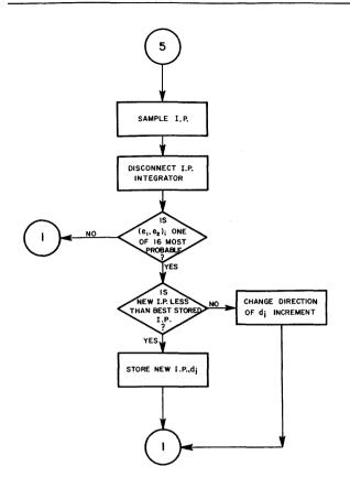
Figure 8. Flow Diagram (Part III).
