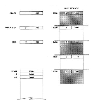
Figure 10d. 'Removing' Blocks from Free Storage-Final Condition.
