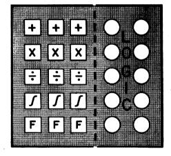
Figure 2. The modern analog computer must be characterized as a parallel machine. Not solely a computer for continuous variables, it is a parallel assemblage of building blocks: integrators, multipliers, etc., for continuous variables; and flip-flops, gates, counters, etc., and "digital" circuits for discrete variables. It is organized for convenient simulation of an "analogous" physical system by a computer model that is constructed of these building blocks.
