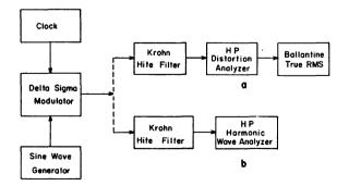
Figure 11. Equipment Setup for Measurement of Signal to Noise Ratio and Spectrum.
