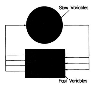
Figure 15. The relative speeds of computation inherent in the different computing techniques are important considerations in the planning of a computer simulation of a large complex system. The presence of a wide range of signal frequencies in a system to be simulated is the one characteristic that most clearly indicates the need for a hybrid computer.
