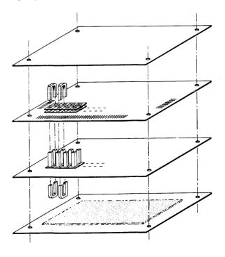
Figure 11. Exploded View of MIRF Module.
