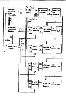
Figure 18. Digital Logic Block Diagram.
