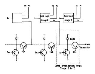
Figure 14. Block Diagram of the Kilburn Adder.
