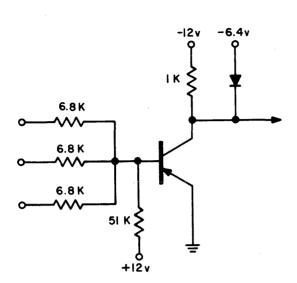
Figure 8. RTL Circuit Designed for the MIRF System.
