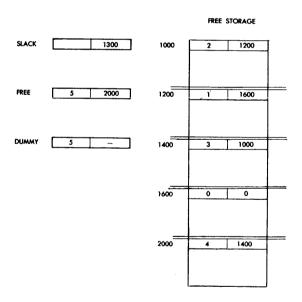
Figure 12d. 'Returning' Blocks to Free Storage— Final Condition.
