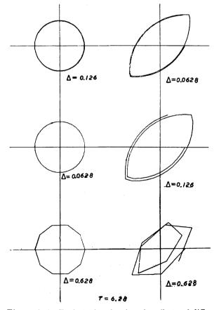
Figure A-1. Trajectories showing the effects of different integration step sizes  $(\triangle)$  on the Runge-Kutta method. Period of unforced system being integrated was T = 6.2836.
