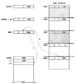
Figure 10a. 'Removing' Blocks from Free Storage— First Step.
