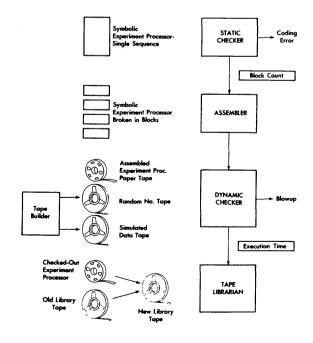
Figure 8. Flow of Experiment Processor from Coding to Library Tape.
