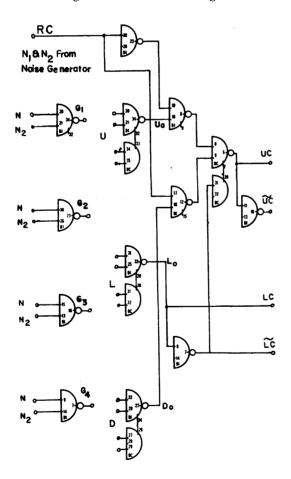
Figure 10a. U-L-D Selector Circuit.
