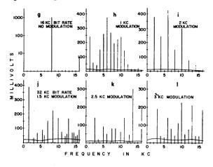
Figure 13. Spectrum Study of Flip-flop Output.
