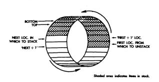
Figure 5. 'Barrel-Like' Composition of Stacking Buffers.
