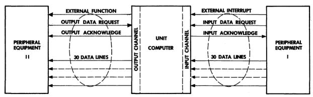
Figure 1. Normal Channel Configuration.
