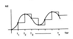
Figure 5. Arbitrary Input Sampled by Zero-Order Hold.
