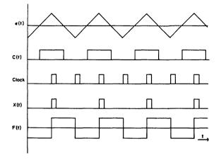
Figure 2. Modulator Waveforms for Zero Input Signal.
