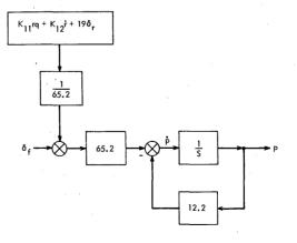
Figure 11. Transfer Function Diagram for Aircraft Roll Rate.
