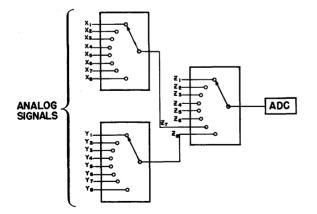
Figure 10. Cascaded multiplexers, in this or other configurations, can aid in establishing multiple sampling rates for different groups of analog signals.
