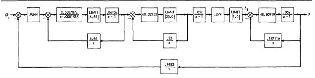
Figure 14. Roll Channel Z Transform Transfer Function (Roots and Steady-State Gain Adjusted).
