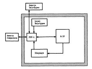
Figure 1. Remote Equipment Configuration.
