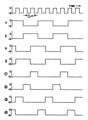
Figure B. Four Staggered 1 Mc Sampling Pulses.
