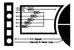
Figure 3. ADC's and DAC's are format converters, changing voltage to numbers and vice versa. As components of the parallel machine the converters together with logic components must act to "match impedances," i.e., resolve the incompatibility between the parallel and sequential programs.
