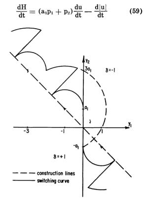
Figure 6. Optimum Switching Curve (minimum time).
