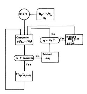
Figure 5. Flow Diagram for a Typical Optimization Routine.
