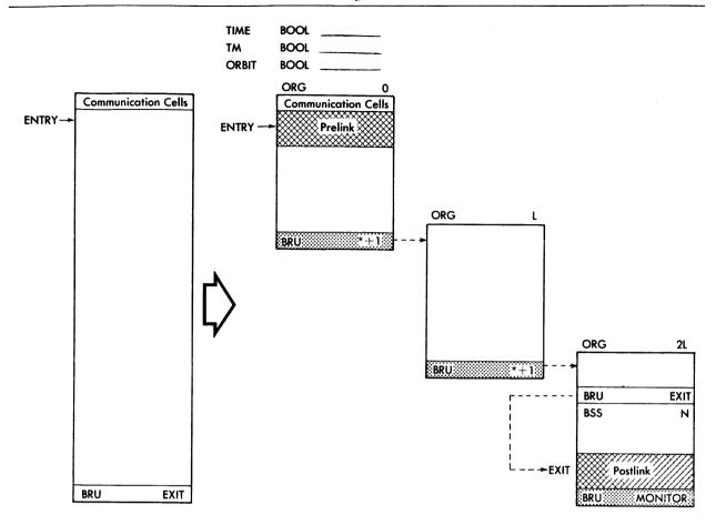
Figure 7. Conversion to Uniform-Length Blocks by Static Checker.
