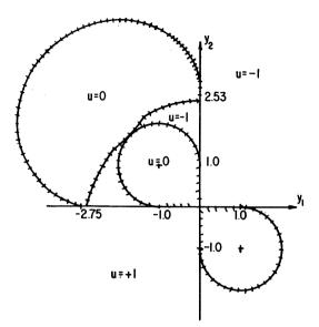
Figure 15. Switching Criteria for Minimum Fuel,  $a_1 = 1.0.$
