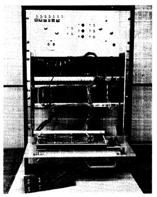
Figure 6. Photograph of the Optimizer. A D/A multiplier card is shown at bottom left.
