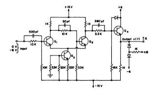
Figure 8. Level-Shifting and Clamping Circuitry.
