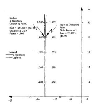
Figure 13. S-Flane Root Locus Plot with Gain Factor (K) as a Parameter.
