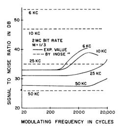
Figure 12c.  $\triangle \Sigma$  S/N Ratio Using Four Filter Cutoff Frequencies.
