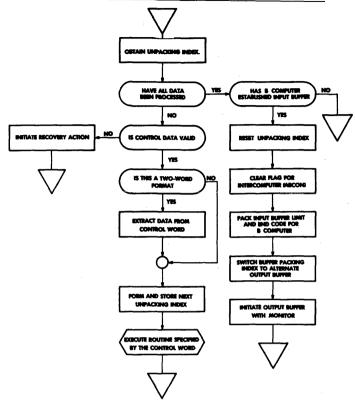
Figure 9. A-B Intercomputer Control Subprogram (ABCON).
