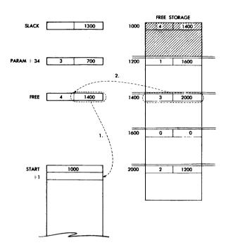
Figure 10b. 'Removing' Blocks from Free Storage-Second Step.
