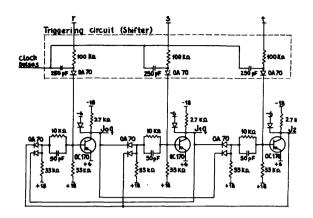
Figure 10. Electronic Diagram of a "3-input" Tristable Multi-vibrator, Selected as the Basic Sequential Unit.
