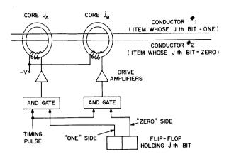
Figure 4. Circuit for Testing Identity.
