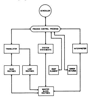
Figure 2.7a. General Diagram of Process Control Flow
