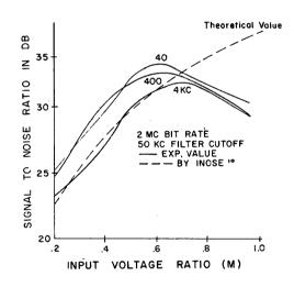
Figure 12d.  $\triangle \Sigma$  S/N Ratio Using Three Modulating Frequencies.
