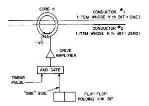
Figure 3. Circuit for Testing Inclusion.
