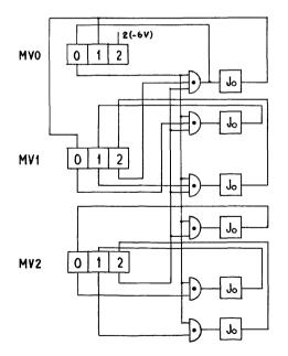
Figure 12. Logical Diagram Showing a Base Three Decade Counter.
