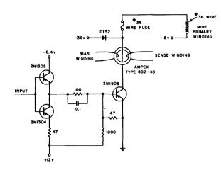
Figure 5. Schematic of MIRF Driver.
