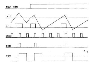
Figure 7. Modulator Waveforms for Half Full Scale Input.
