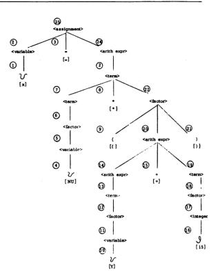
Figure 2. Syntax Tree for the  $\langle Assignment \rangle$ "X = NU\* (Y + 15)."
