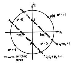
Figure 10. Switching Criteria in p1 vs. p2 Phase Plane.
