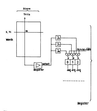
Figure 13. Concerning to the Transfer of Information from the Thin-Film Store to a MVs. Register.
