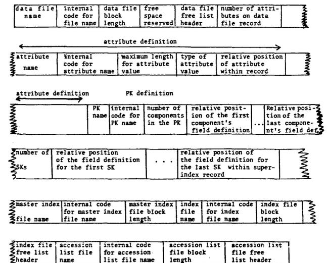
Figure 8—Superindex record structure
