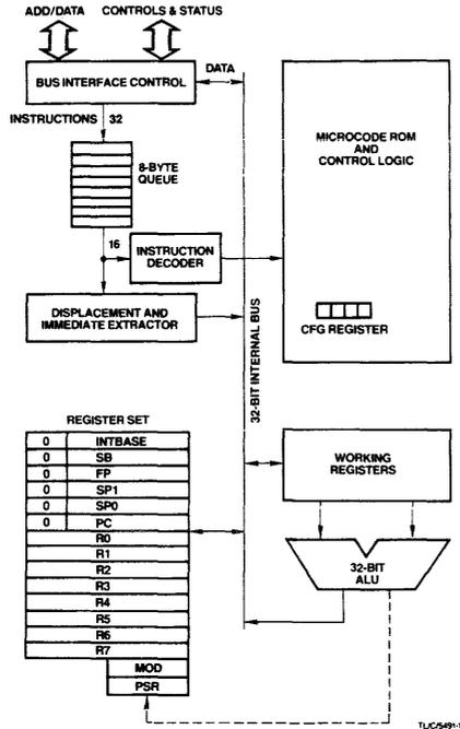
Figure 1—Special NS32032 circuitry avoids alignment restrictions
