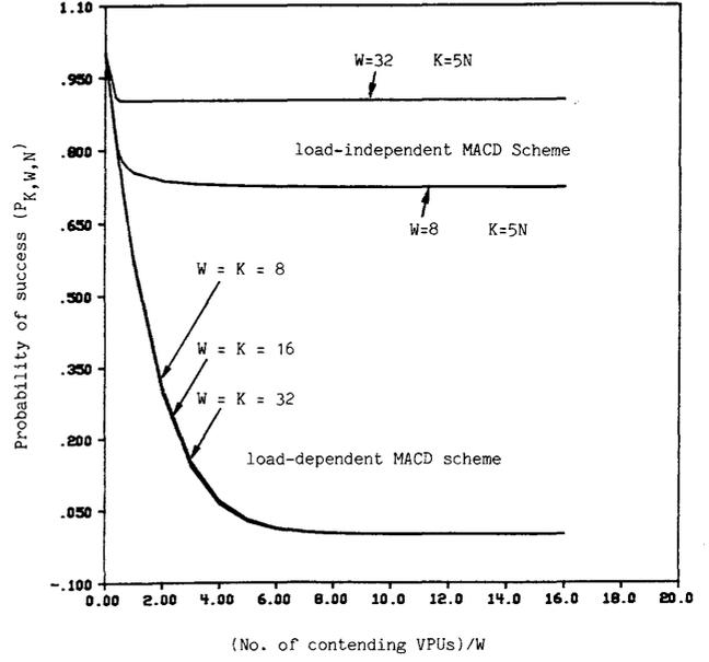
Figure 3—Probability of success in one contention using multiaccess code-deciphering bus arbitration scheme ( $K$  is the size of code space;  $W$  is the bus width,  $N$  is the number of contending VPU's)
