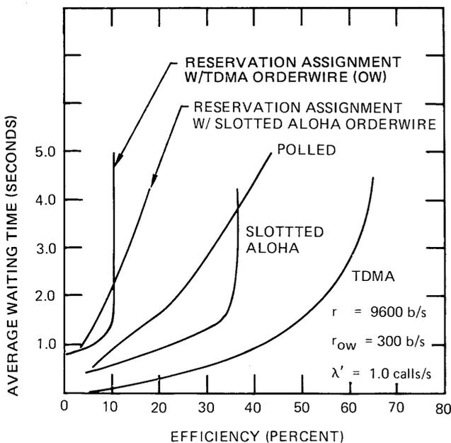
Figure 7—Efficiency of channel sharing protocols at high call rate
