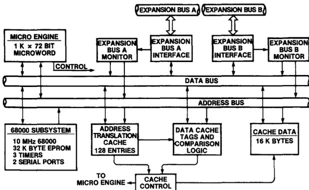
Figure 12—Synapse general-purpose processor
