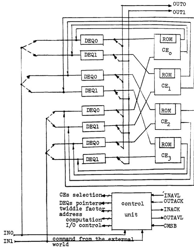
Figure 6—The circuit diagram of the parallel FFT quotient network (PARQUO) with four computation elements
