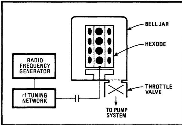
Figure 14—Reactive-ion etched schematic
