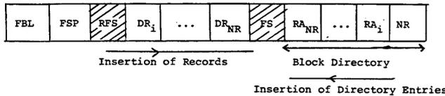
Note: FBL: free block link; FSP: free space pointer; RFS: reserved free space; DR<sub>i</sub>: *i*th record in the block (see Figure 2); FS: free space; RA<sub>i</sub>: relative address of the *i*th record in the block; NR: number of records in the block.
