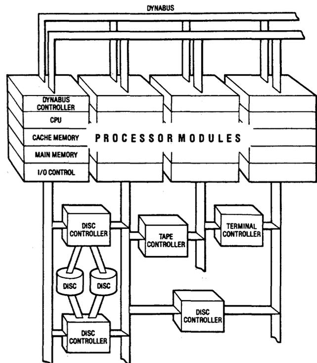
Figure 1—Tandem's NonStop system architecture
