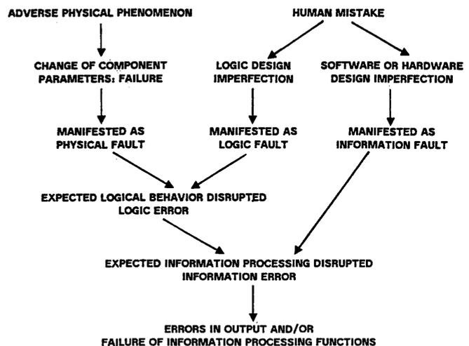
Figure 1—An analogy between physical and design faults
