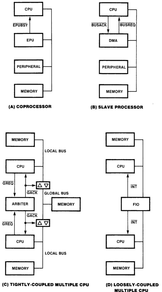
Figure 7—Multiprocessing support
