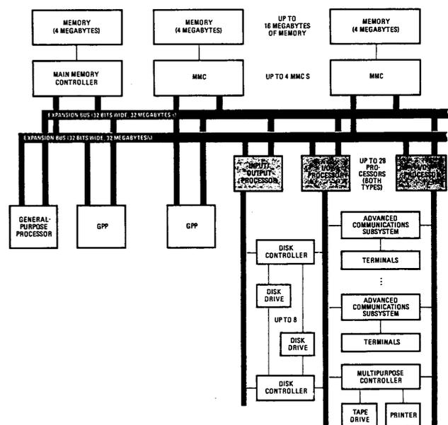
Figure 3—The Synapse system architecture
