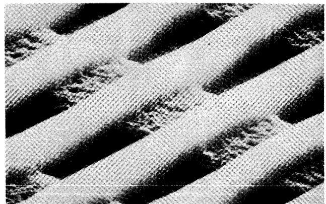
Figure 13—Reactive-ion etched structure
