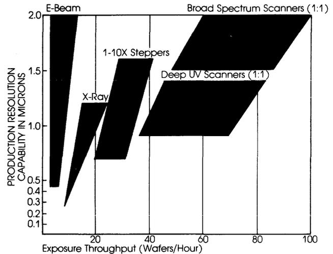
Figure 12—IC lithography strategy vs. image resolution and wafer throughput
