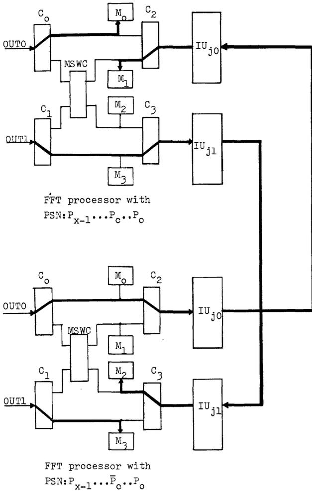
Figure 12—The data exchange of parallel 1-D FFT processing scheme
