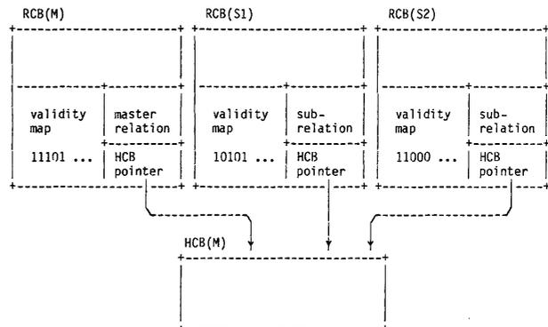
Figure 3—Linkage of subrelations S1 and S2 to the heap of their master relation M
