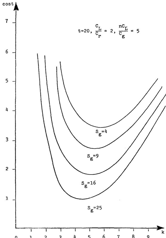
Figure 5—Cost versus k for k-step t/S-fault diagnosability ( $S_g$  is constrained)
