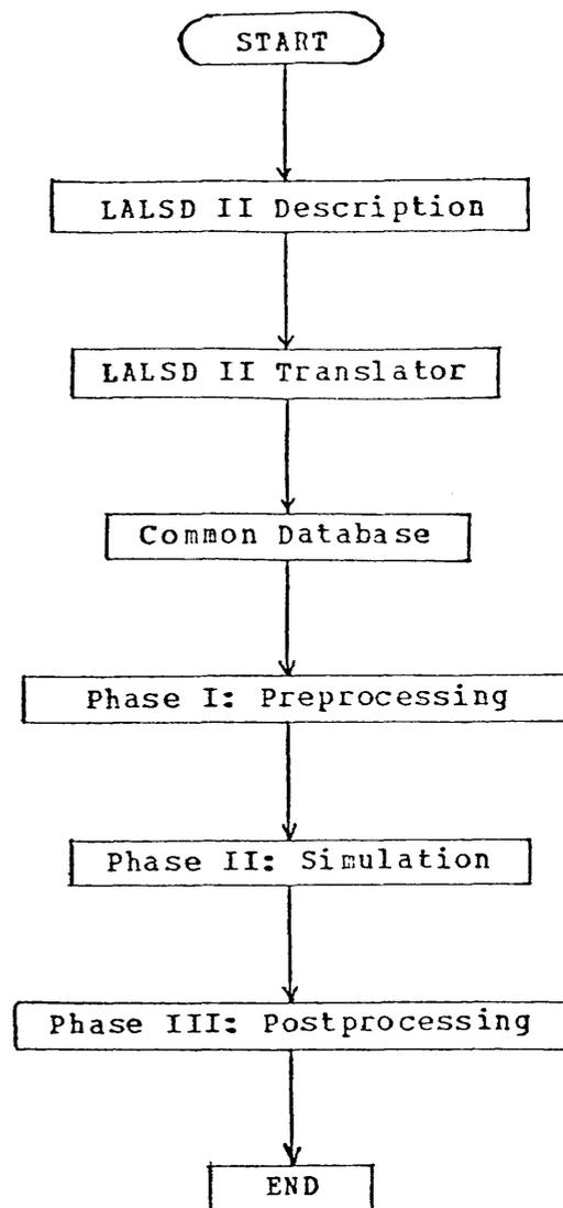
Figure 3—Overall structure of LALSD-II-driven simulator
