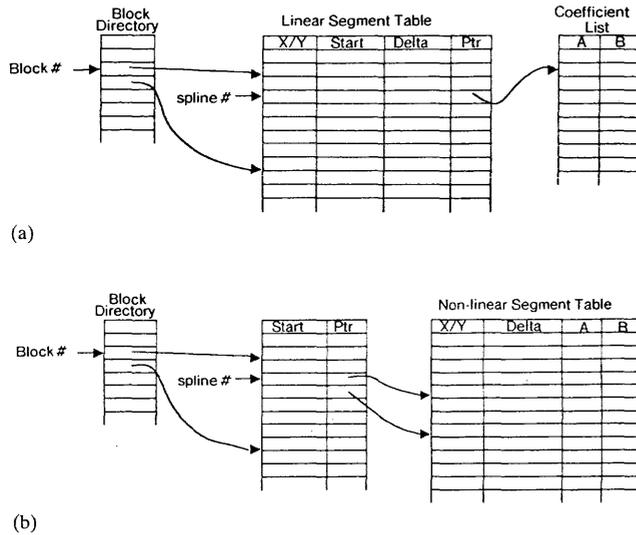
Figure 12—Picture database: (a) linear segments; (b) nonlinear segments
