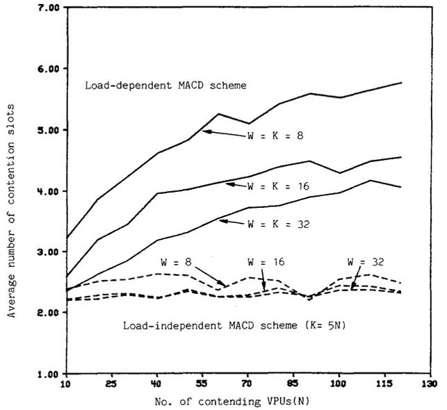
Figure 4—Average number of contention slots for resolving conflicts of bus requests using multiaccess code-deciphering scheme ( $K$  is the size of code space;  $W$  is the bus width,  $N$  is the number of contending VPU's)
