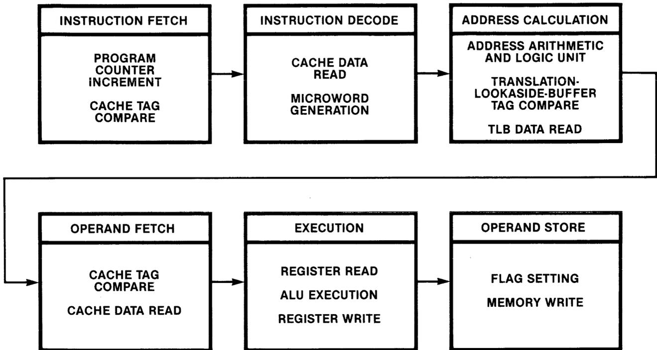
Figure 5—Six-stage pipeline
