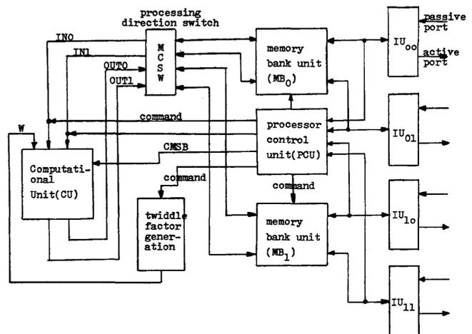
Figure 2—The block diagram of a versatile VLSI FFT processor
