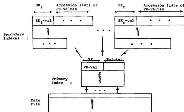
Figure 2—Inverted file organization using primary and secondary indexes
