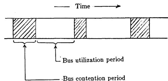
Figure 2—Operation mode of a shared bus
