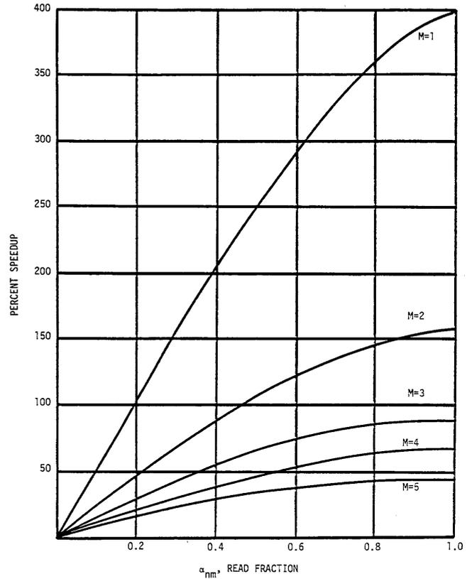
Figure 5—Speed-up as a function of read fraction for N = 5 processors
