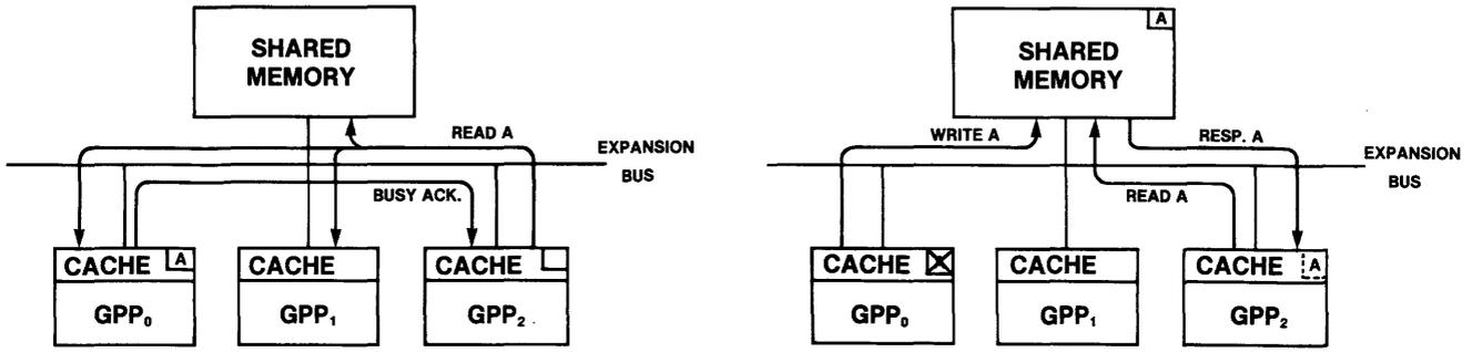
Figure 11—Read public request (a) causes the owner to busy the request; (b) shared memory responds to subsequent request
