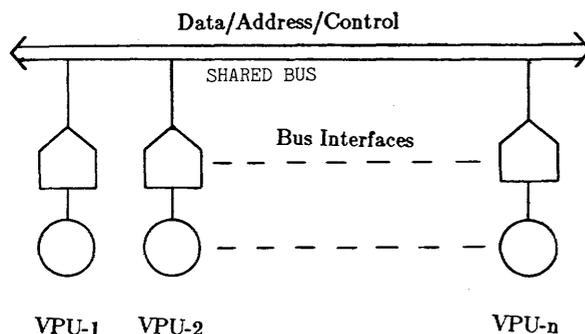
Figure 1—Configuration of a VLSI-densed system
