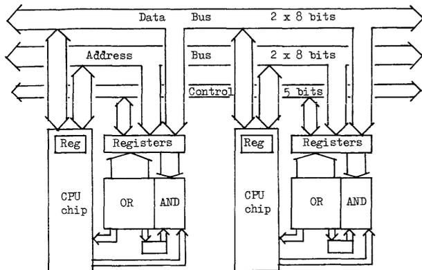
Figure 12—Bus and memory controllers
