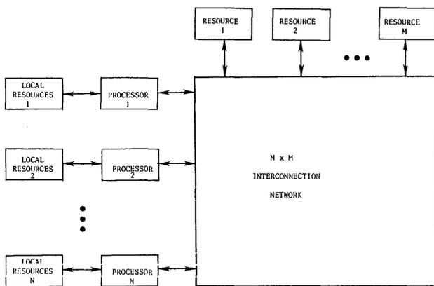
Figure 2—A multiprocessor computer block diagram
