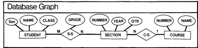
Figure 2—E-R graph representation of a database schema
