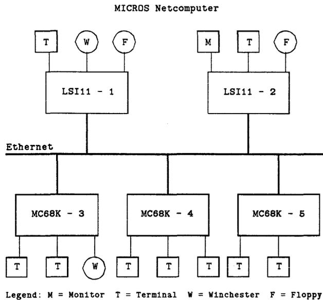
Figure 2—Initial network configuration used by SAM2S
