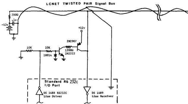
Figure 2—RS232C to LCNET adapter
