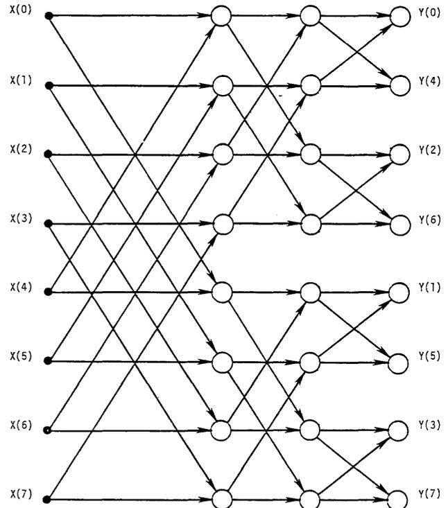
Figure 3—Signal flow graph for an eight-point FFT
