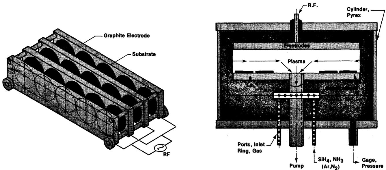
Figure 16—Two types of PECVD reactors
