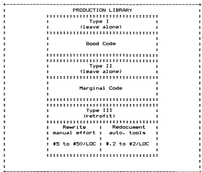
Figure 1—Decision schematic for production code
