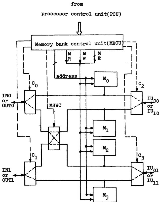
Figure 3—The circuit diagram of memory bank unit
