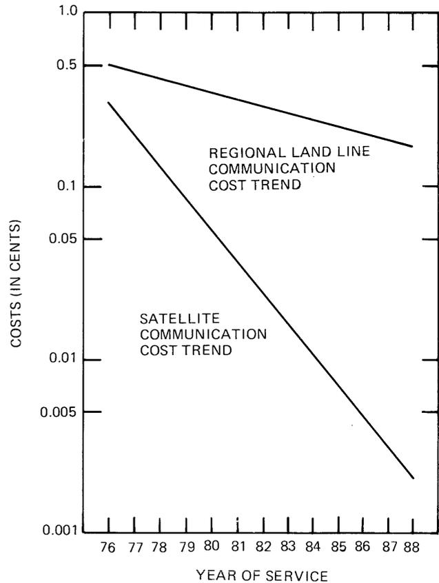
Figure 8—Incremental cost for sending 1 megabit through nationwide network
