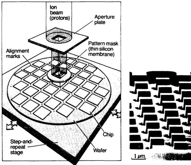
Figure 11—Ion beam exposure principle and resist image
