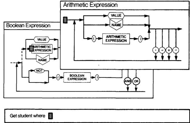
Figure 4—User selects “arithmetic expression” option, and the arithmetic expression syntax diagram is displayed
