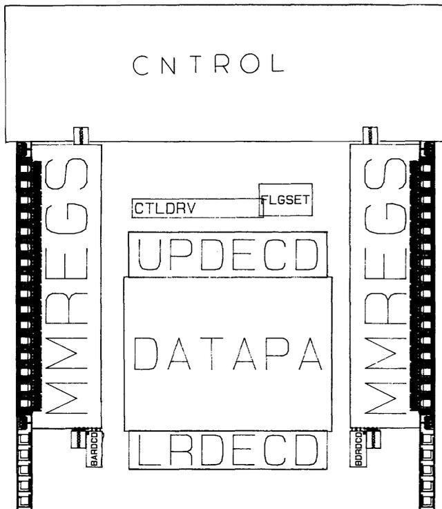
Figure 14—Floor plan of CPU chip
