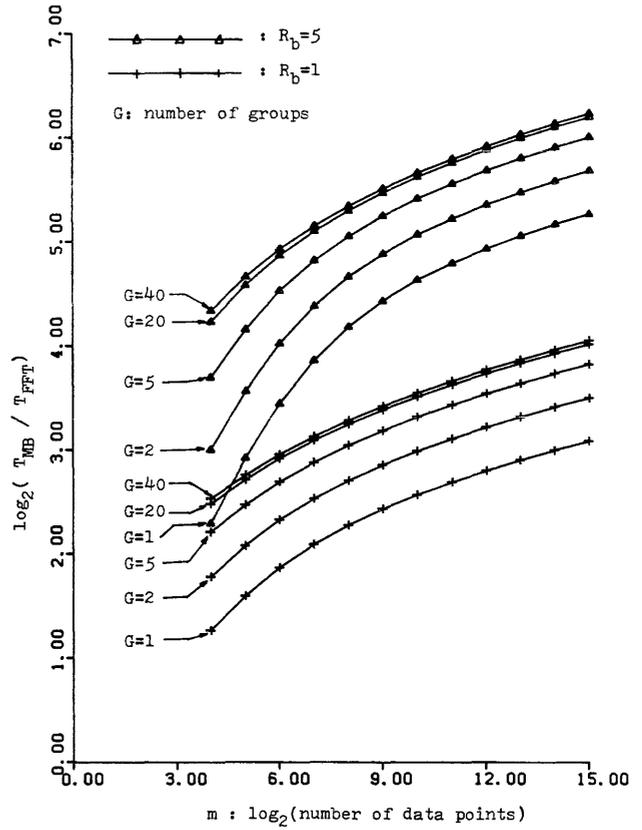
Figure 15—The  $\log_2$  speed-up of the cascade 1-D FFT processing scheme, as a function of  $m$  and  $G$
