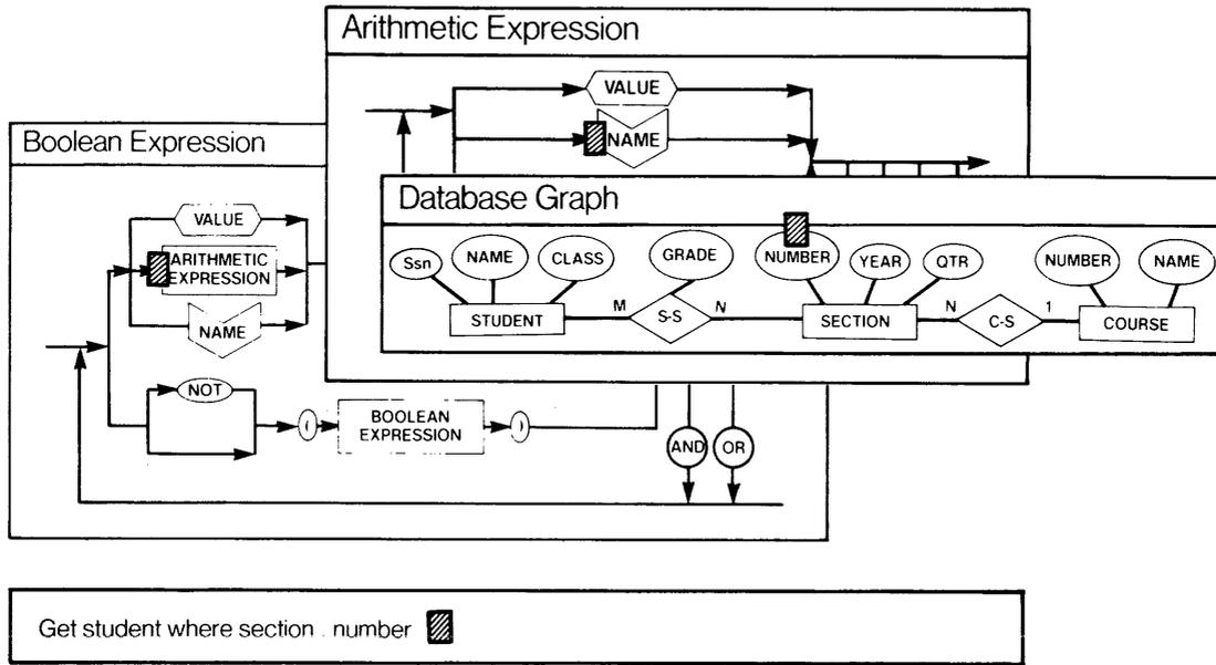
Figure 6—User selects “section.number” option from database graph
