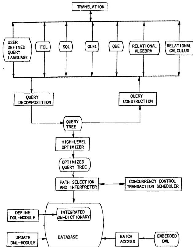
Figure 1—The general structure of the system
