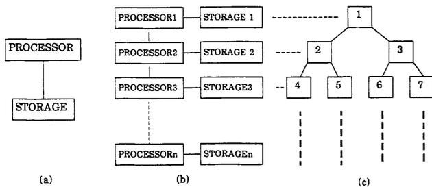
Figure 6—Three methods of realizing index circuits and function storage circuits: (a), microprocessor system; (b), a tree realized by assigning one processor to each level; (c), storage cells integrated with processors
