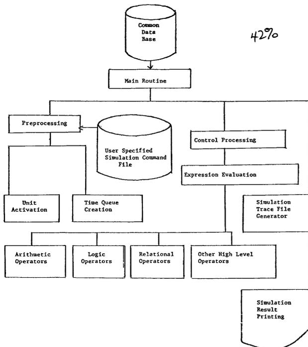
Figure 4—Overall flow of the simulation process
