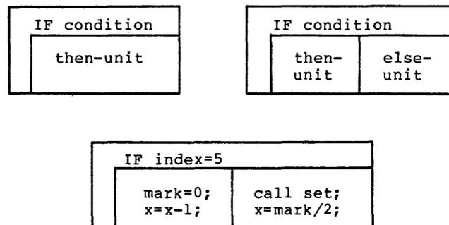
Figure 3—The two alternative forms of the IF construct and an illustrative example
