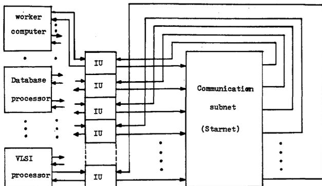
Figure 1—The block diagram of the Star communication subnet.
