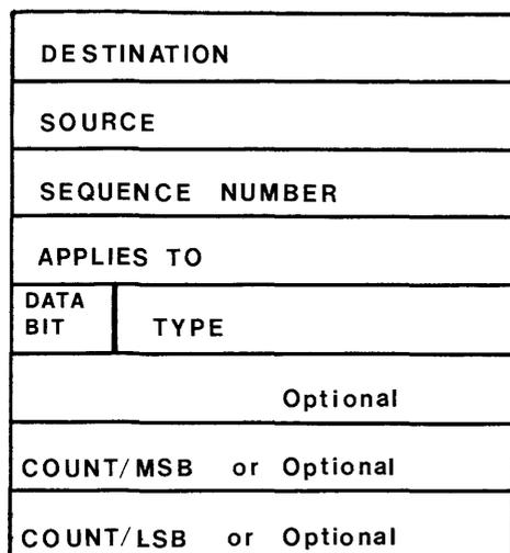
Figure 3—LCNET to message header structure
