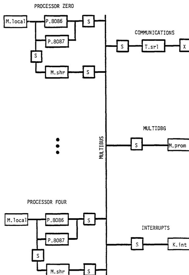
Figure 1—PMS diagram of a multiprocessor with replicated shared memory
