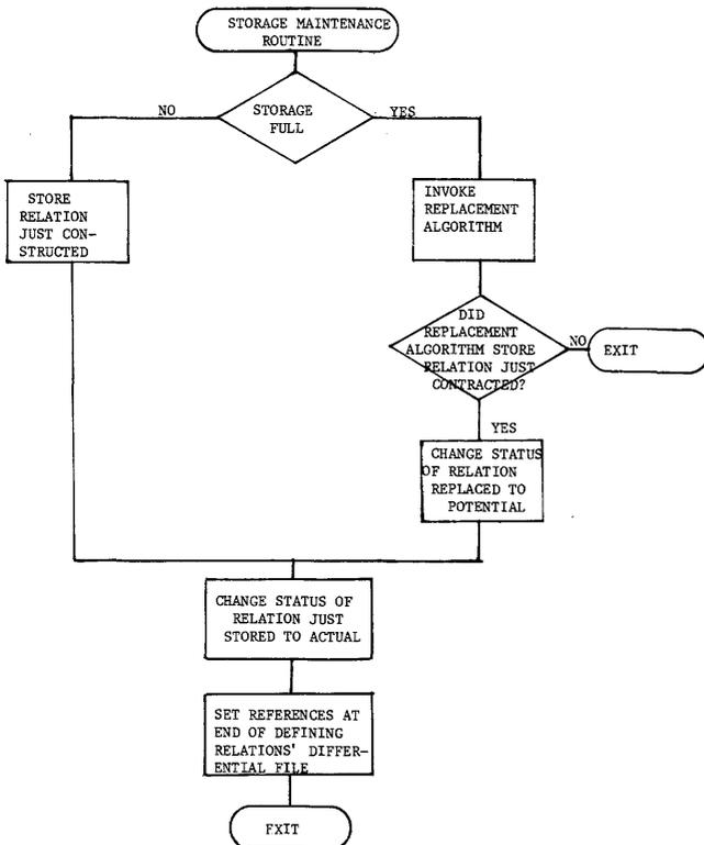
Figure 5—General flow for maintaining use of storage
