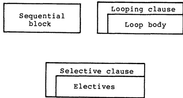
Figure 1—The basic flow block graphics corresponding to the three fundamental control forms of sequence, repetition, and selection
