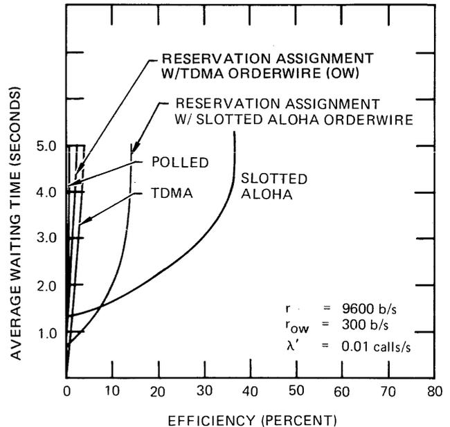
Figure 5—Efficiency of channel sharing protocols at low call rate
