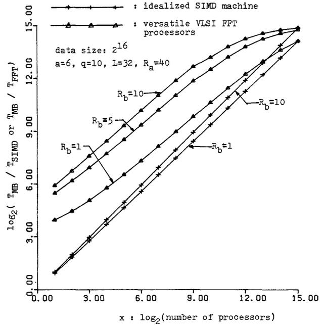
Figure 16—The  $\log_2$  speed-up of an idealized SIMD machine and versatile FFT processors in parallel 1-D FFT processing scheme as a function of  $x$  and  $R_b$
