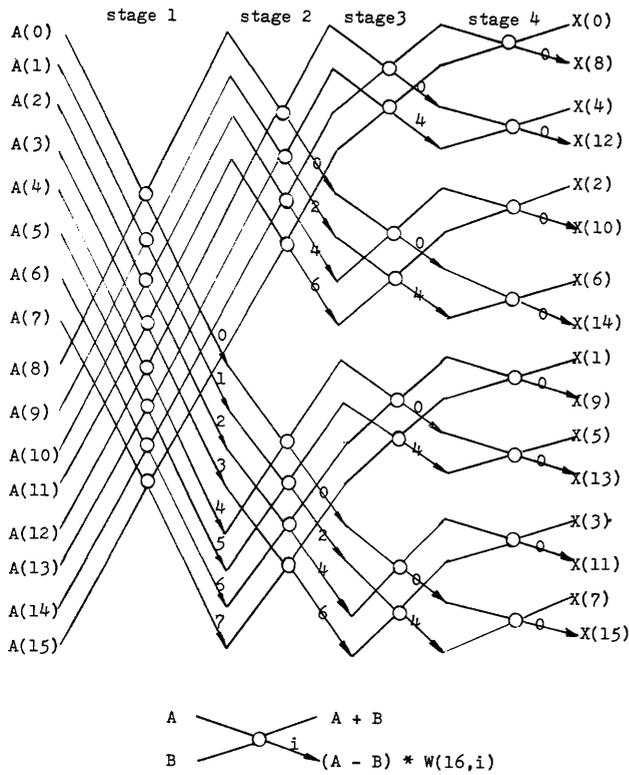
Figure 7—The signal flowgraph of a 16-point radix-2 Decimation-In-Frequency FFT algorithm with the in-place property
