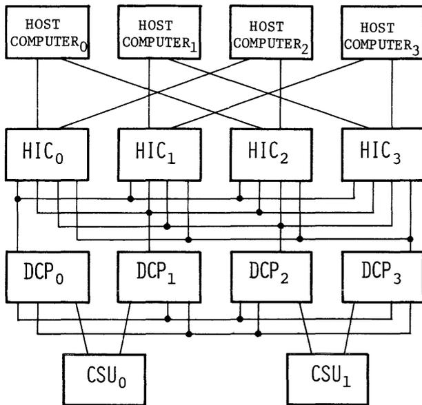
Figure 6—System redundancy in a four-host DCS configuration
