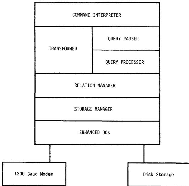
Figure 1—The structure of the components of Sibyl
