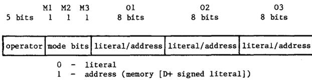
Figure 8—Microcomputer instruction format (2 × 16 bits)
