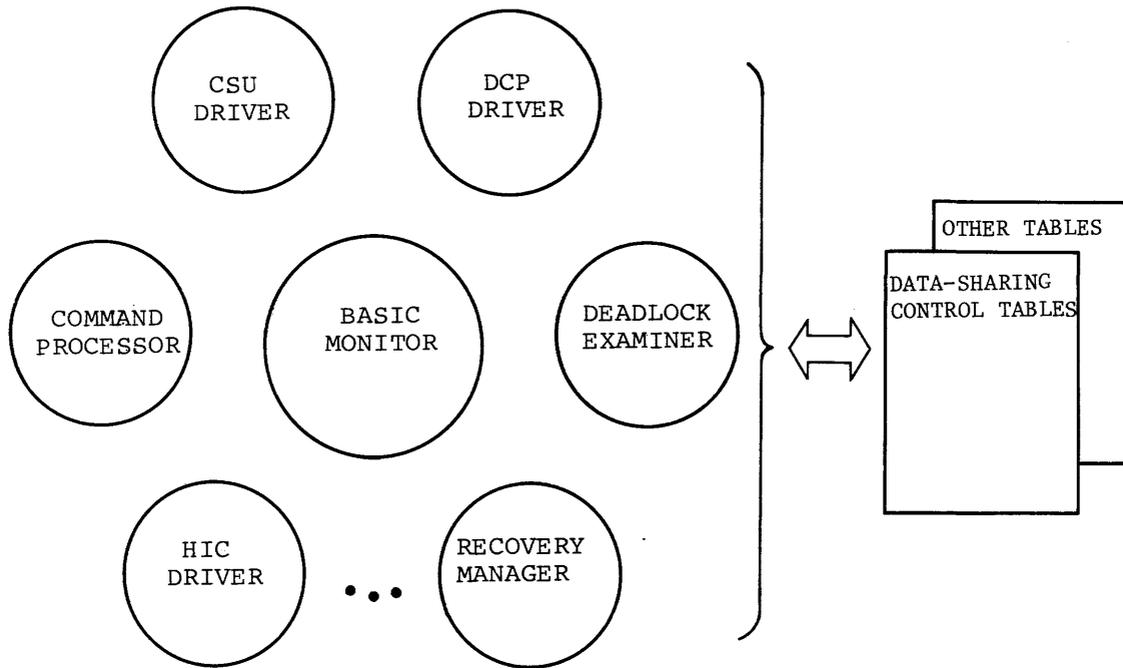
Figure 4—DCP control software
