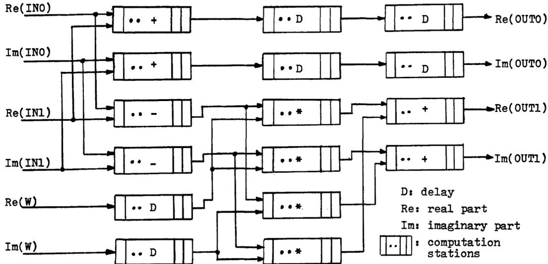
Figure 5—A pipeline butterfly computation element
