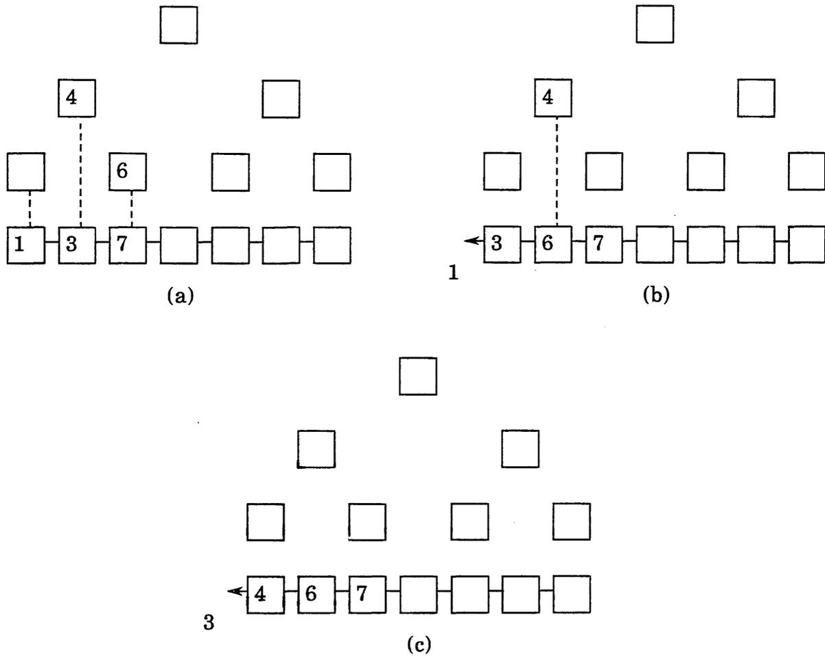
Figure 12—Simulation of the up-down sorter
