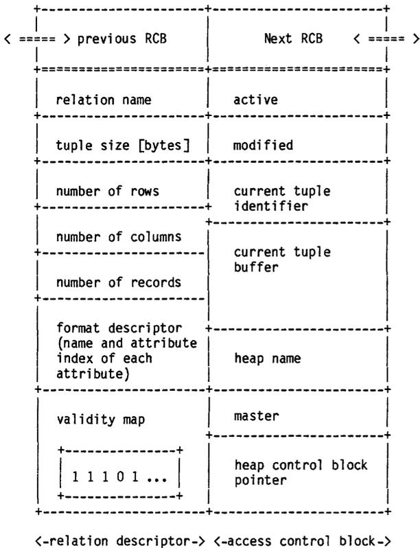
Figure 2—A relation control block consists of a relation descriptor and an access control block
