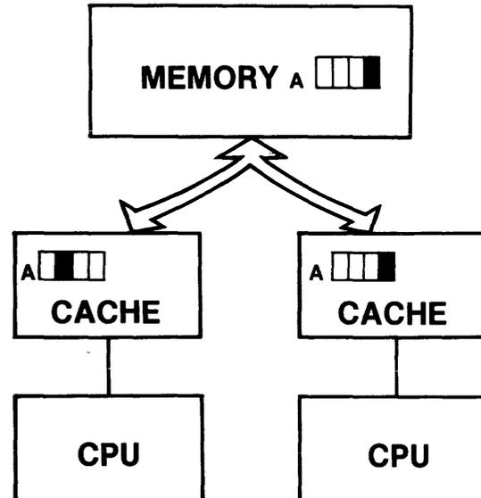
Figure 2—Multicache coherency
