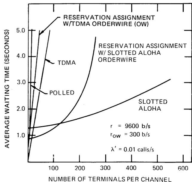
Figure 6—Terminals per channel at low call rate
