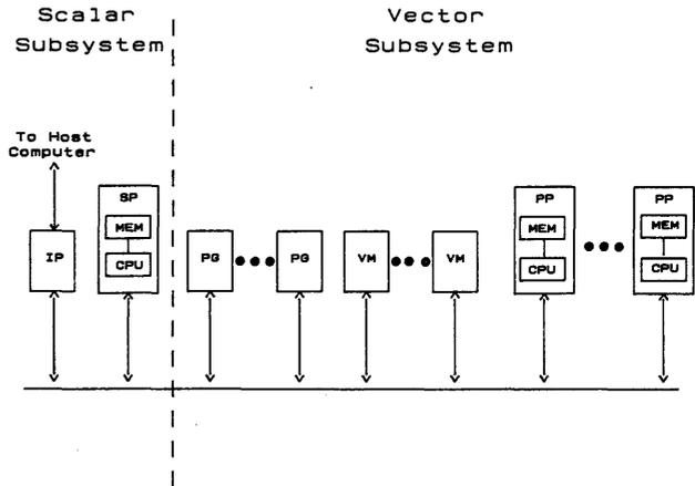
Figure 3—Array processor block diagram
