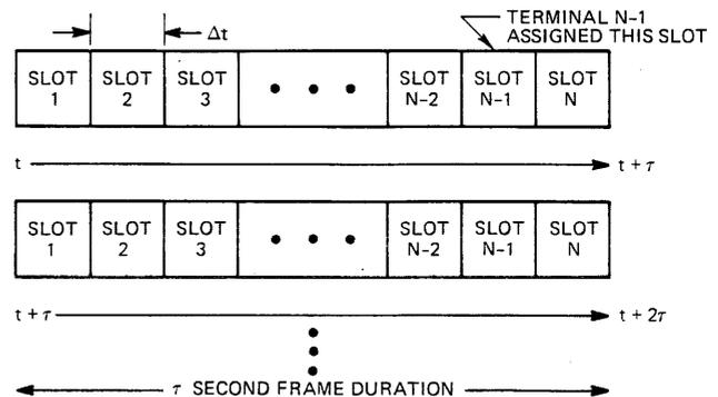
Figure 3—Time division multiple access sharing of the traffic channel
