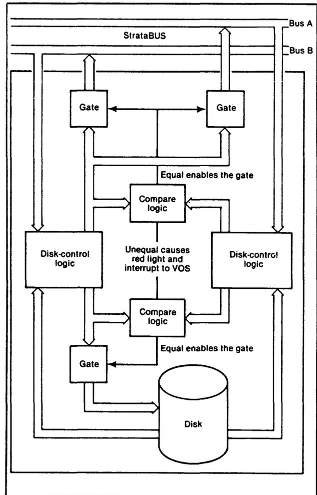
Figure 2—A stratus self-checking disk controller
