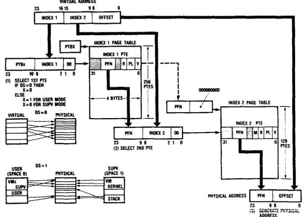
Figure 4—NS32032/NS16082 memory management uses memory-based tables
