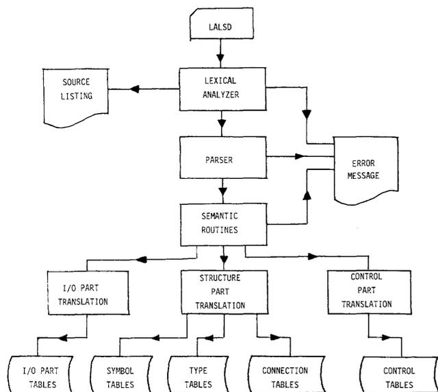
Figure 2—Block diagram for translator
