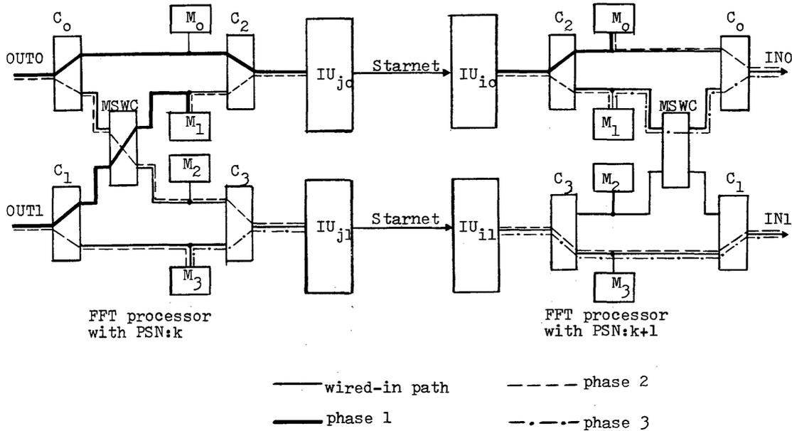
Figure 9—The data movement of cascade 1-D FFT processing scheme
