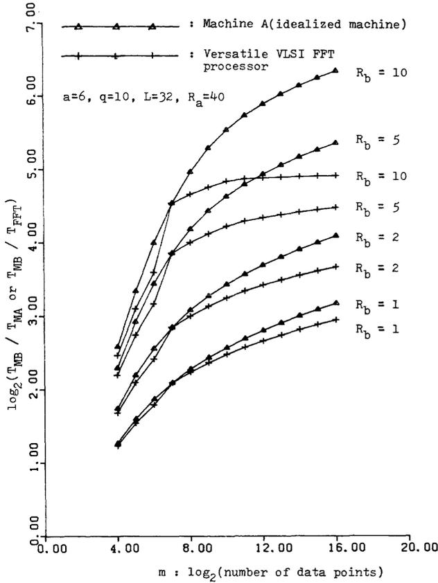
Figure 14—The  $\log_2$  speed-up of the machine A and versatile FFT processor in 1-D FFT processing scheme as a function of  $m$  and  $R_b$
