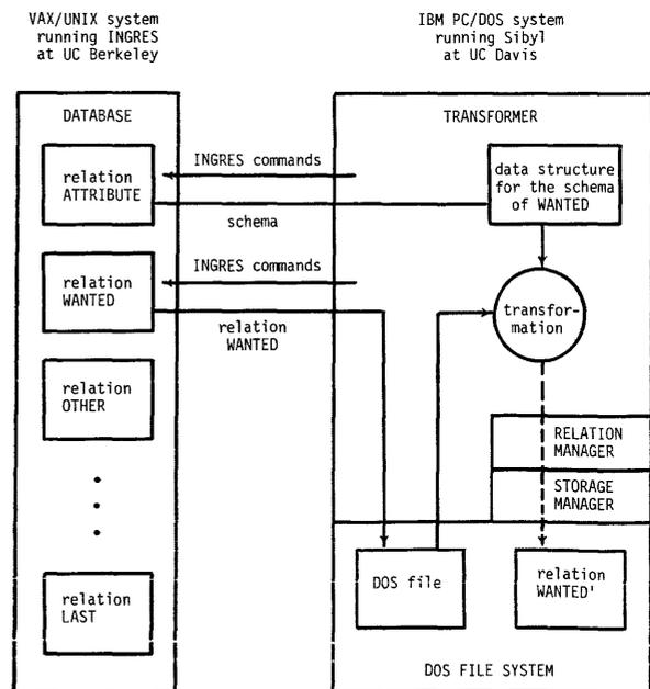
Figure 7—Transformer operations during a transfer from INGRES to Sibyl
