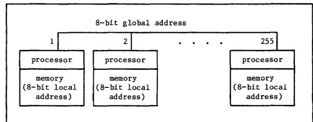
Figure 1—Multi-microcomputer system
