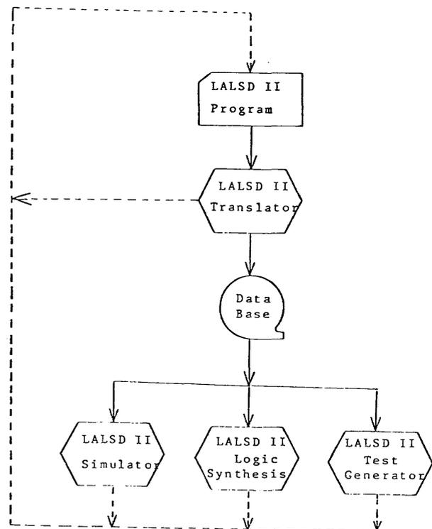
Figure 1—LALSD-II-driven design automation system
