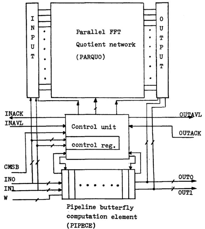
Figure 4—The block diagram of a VLSI FFT circuit
