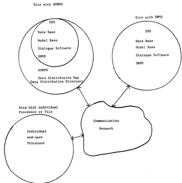
Notes: (1) NDBMS stands for network database management system. (2) The three types of site can be many in a network decision support system. For simplicity, only one of each type is shown. (3) Communication network is a network system for data communication.
