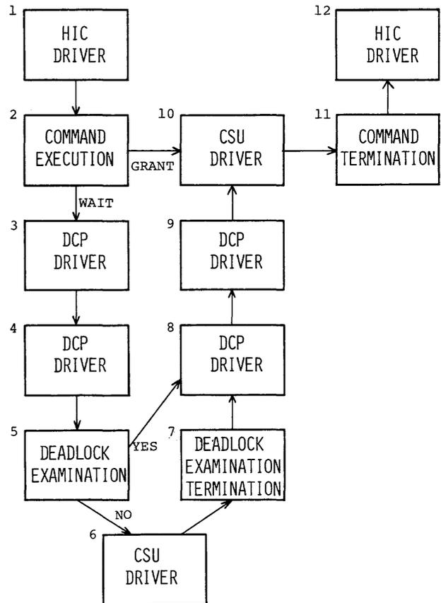
Figure 5—General control flow representing a “LOCK” command execution
