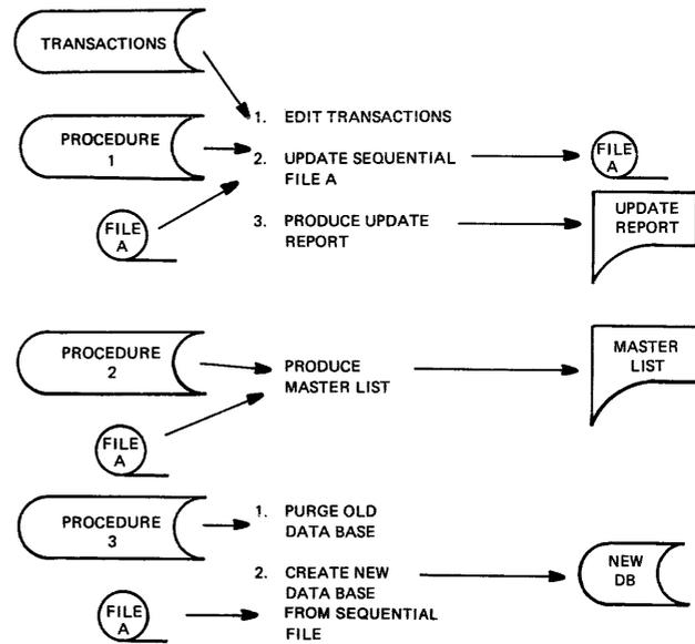
Figure 2—Hierarchical input process output (HIPO)
