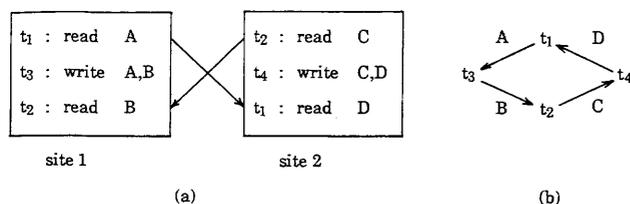
Figure 1—Necessity of the global concurrency control mechanism even if there are no global write transactions
