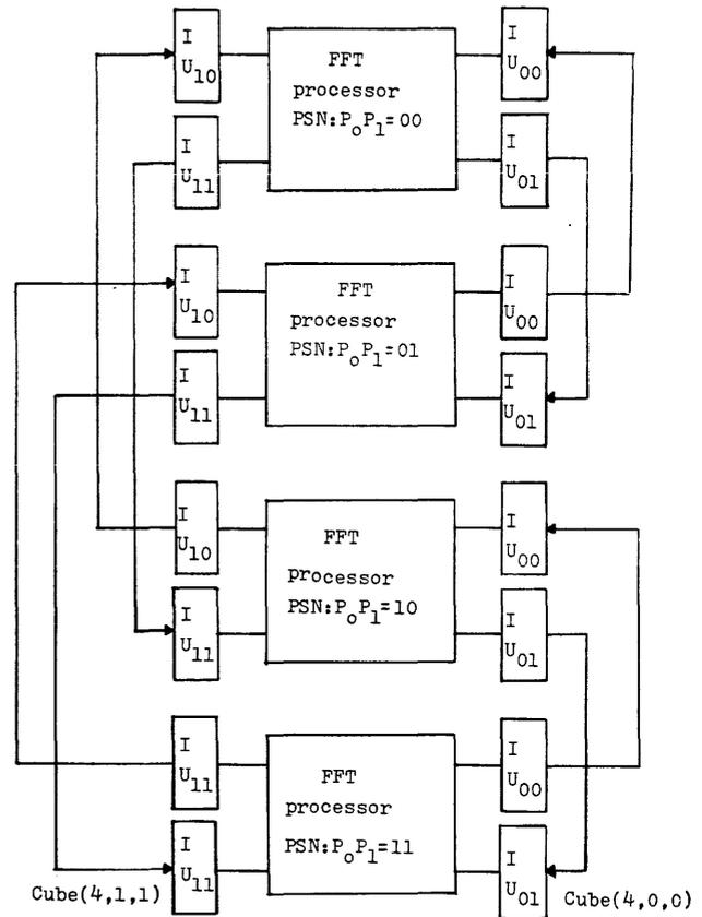
Figure 11—The topology and connection pattern of  $Cube(4, 1, 1)$  and  $Cube(4, 0, 0)$
