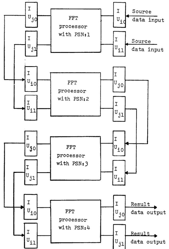
Figure 8—The topology and connection pattern of the linearly connected FFT processors
