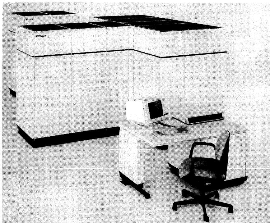
The Amdahl Model 5890-300 is a dual tightly coupled processor which can be configured with up to 256 megabytes of main memory and 64 I/O channels. The 580/Expanded Storage feature is standard and the 580/Multiple Domain Feature is optional.
