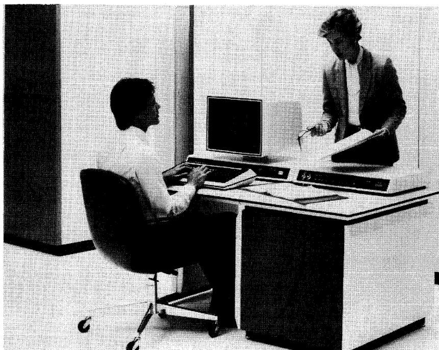
*The Amdahl Model 5860 is the most powerful uniprocessor that Amdahl has ever produced. This member of the Amdahl 580 family represents an evolutionary extension to the product line and offers a compatible growth path for Amdahl 470 users. The 5860 has twice the processing power of Amdahl's 470V/8. Standard features on the 5860 include 16 I/O channels, 16 MB of main storage, two 32K high-speed buffers, power distribution unit, system console and air cooling.*
