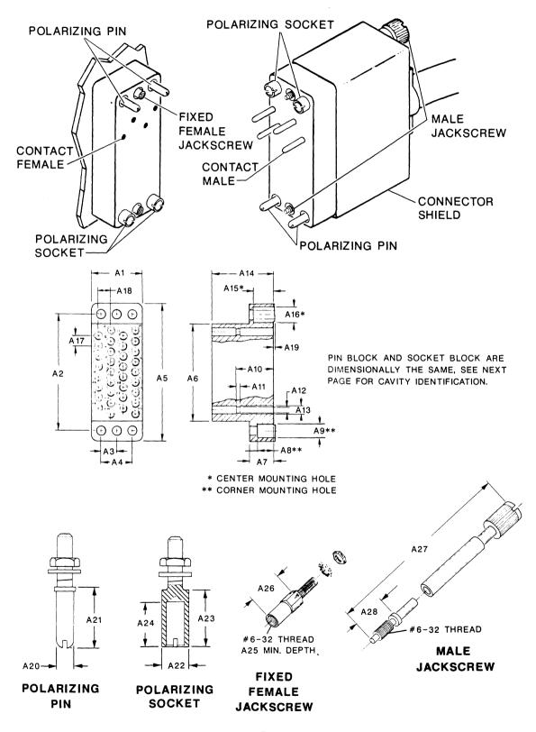
Figure 6 READ/WRITE Round Cable Connectors
