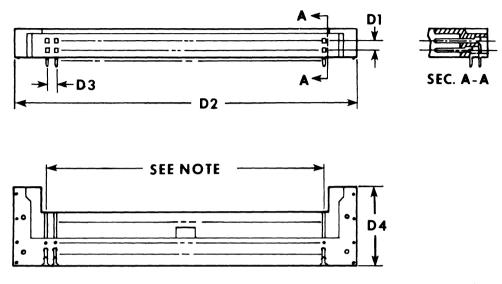
NOTE: 60 contacts on 0.100 inch (2.54 mm) spacing = 2.90 inches (73.66 mm)
