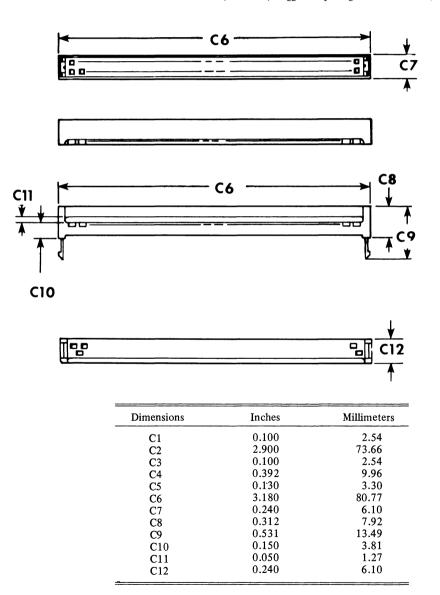
Figure 4 CONTROL Flat Cable Plug
